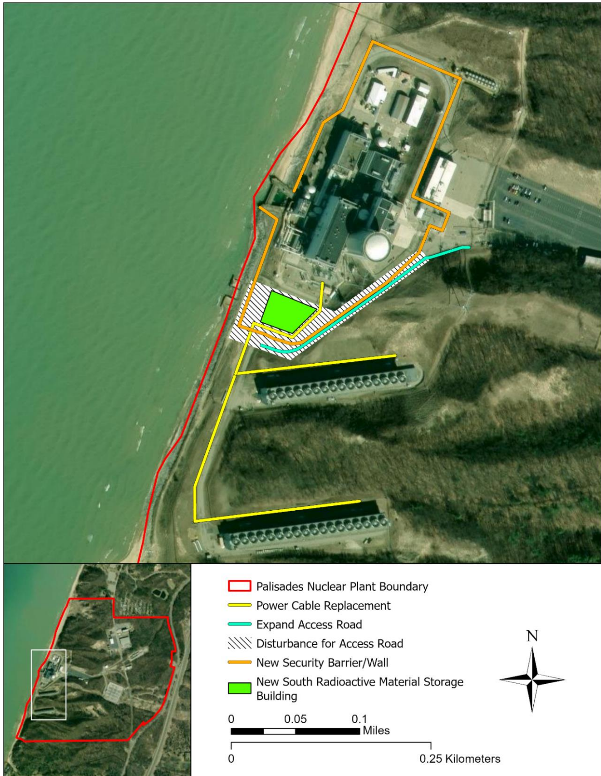
Figure 3-1 Location of Select Ground-Disturbing Activities at Palisades Nuclear Plant Related to the Preparations for the Resumption of Power Operations. Source Data: HDI 2024-TN10670: RAI-GEN-1.
