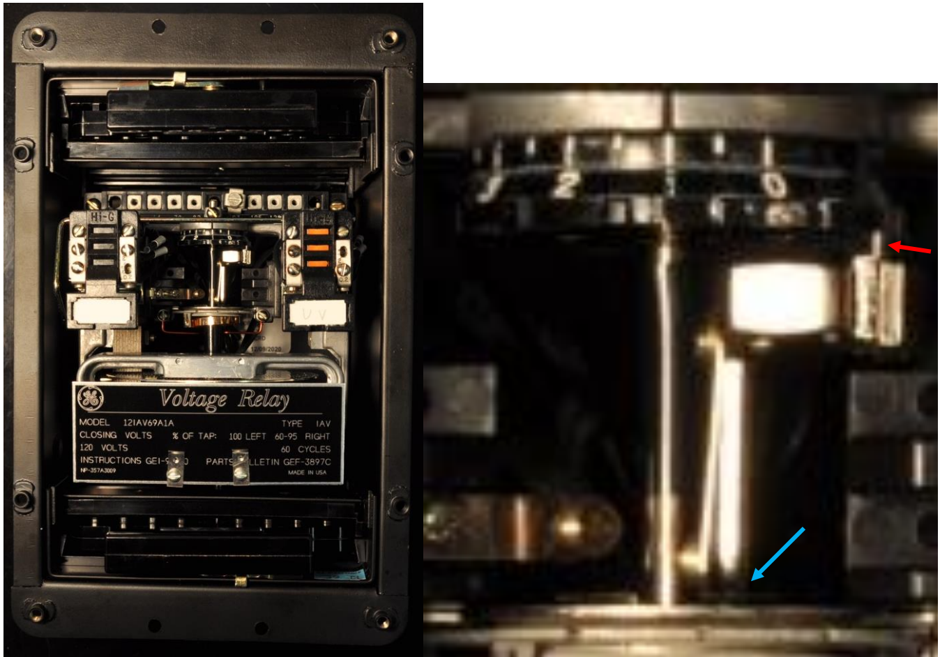
Figure 2. As-received photographs of the front and back of the undervoltage relay are shown in the two photos above. The left photo is with the cover removed. The right photo is a close up of the time dial to show the time dial shaft, as shown with the red arrow, that the stationary undervoltage contact assembly is clamped to. The stationary undervoltage contact was making contact with the plastic disc impeding its travel as shown with a blue arrow.
