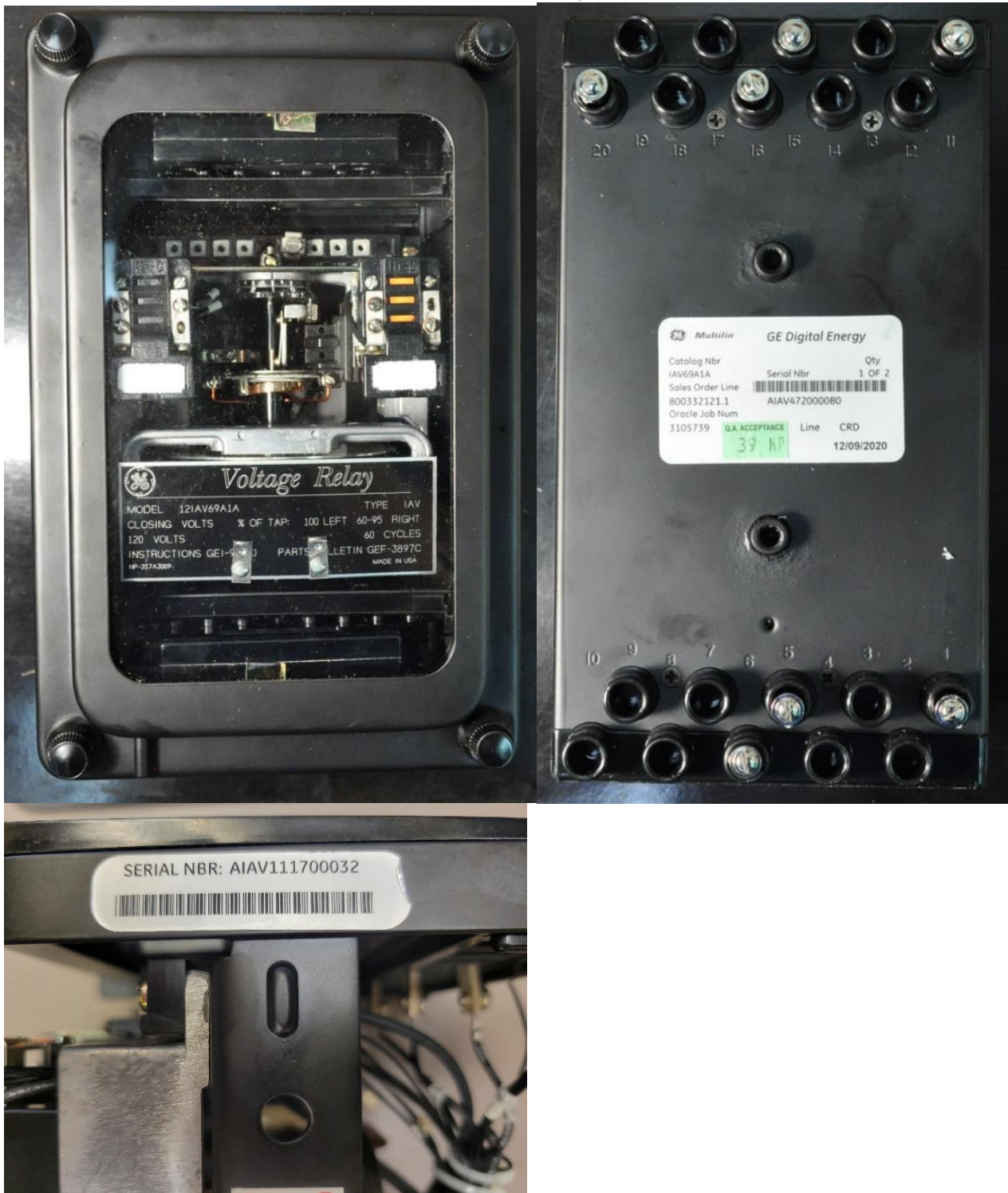
Figure 1. As-received photographs of the front and back of the undervoltage relay are shown. The undervoltage relay was identified as a model 12IAV69A1A, with serial number AIAV111700032, and the manufacturer is General Electric. The relay case had a serial number of AIAV472000080. The Closing Voltage was identified as 100% of the tap for the left overvoltage contactor and 60-95% of the tap for the right undervoltage contactor. It is rated for 120 volts and the instruction for this relay was identified as GEI-90810 which will be reference throughout this report.
