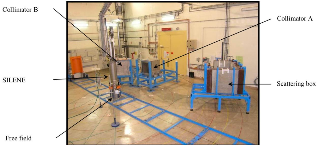
Figure 94. Experimental setup for SILENE Pulse 1 [43].
