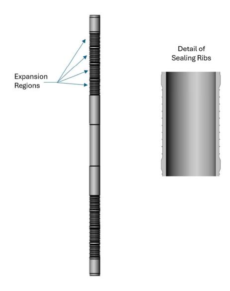
Figure 3.4-2 Sleeve Section Drawing
