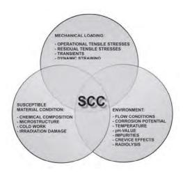
Industry experience has demonstrated that the primary side environment is sufficiently aggressive and that Alloy 600 in all heat-treat conditions (low-temp mill anneal, high-temp mill anneal, and thermally treated) is susceptible to PWSCC when subjected to tensile stresses. Industry-wide, PWSCC has been seen at:
