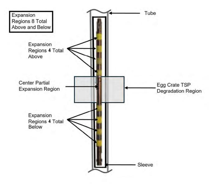
Figure 5-2: Typical Sleeve Installation
