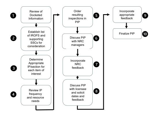
c. From the list created in Step 2, consider the aspects of these items and determine how they may be inspected. If available, utilize IROFS boundary packages to assist in selecting key attributes of the IROFS. Assign an IP or IP section to each of these aspects.
