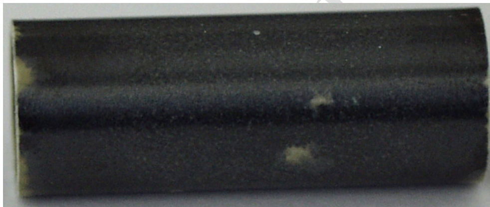
(b) 3,600 s at 1,000°C; 60 wppm hydrogen pickup
