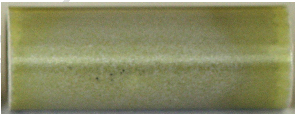
(c) 5,000 s at 1,000°C; 1,350 wppm hydrogen pickup
