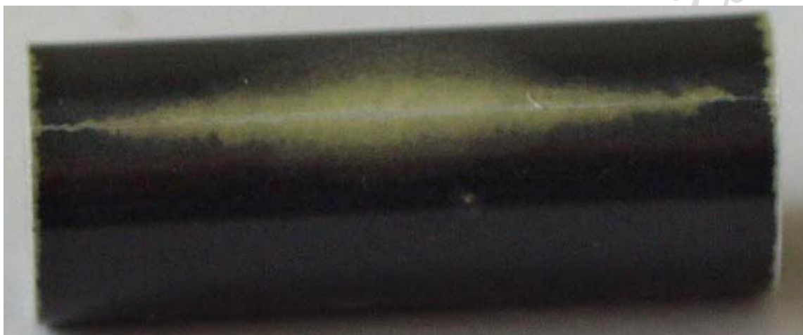
Figure D-5. Outer surface of scratched ZIRLO ® sample following oxidation at 985°C for 3,400 s. Local hydrogen pickup under the yellow surface was 440 wppm; average pickup was 175 wppm.
