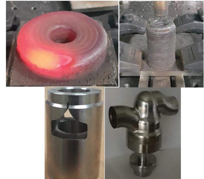
Figure 2. Valve cage in 316L stainless steel in process using GMA-DED, and cage and valve body after final machining [*2] Used with permission from Best Engineering in Energy Solutions
