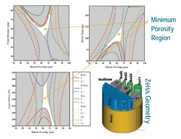
XCT porosity trends for one 316H build PB performed on the Renishaw varying three processing parameters. In each plot, the area between solid and dashed lines indicates porosity below 0.1%. White regions indicate processing space where porosity is minimized for all overlaid curves.
