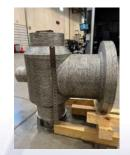
Valve Built Using Gas Metal Arc DED 8" Valve ≅ 1000 lbs. (EPRI/ Lincoln Electric)
