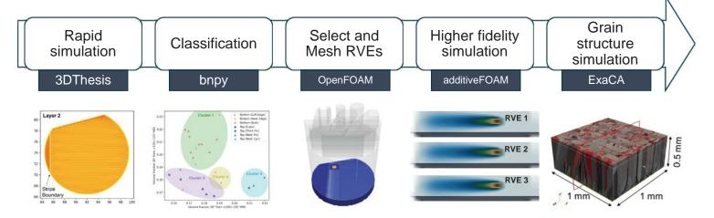
**Output:** Generate representative grain structure statistics for variation found in real parts
