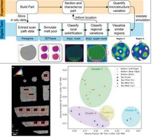
Workflow developed to generate and classify simulated thermal data for AM processing. Classification was experimentally validated for SS316L
