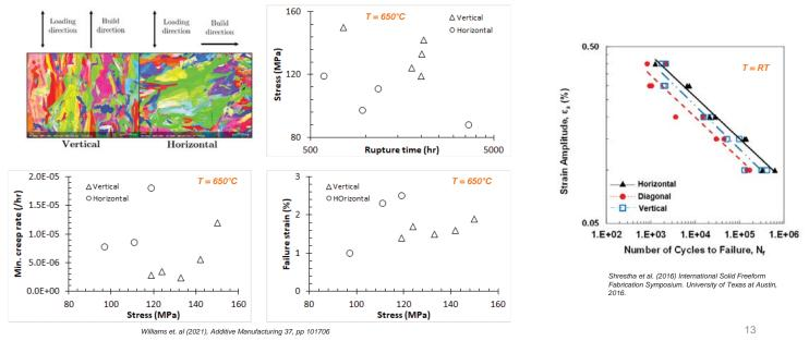
Preliminary high temperature testing – heat treatment
