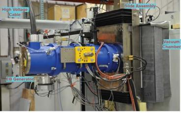
Electron Beam Generator (Gun) set up at PTR
