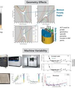
Volumetric energy density provides a reasonable first-pass optimization parameter for porosity minimization.
