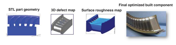
AM defect prediction model successfully applied to complex component build and final process design and control requirements
