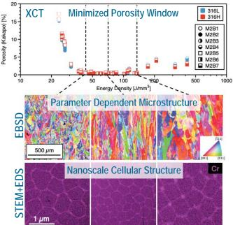
Multiscale characterization using XCT, EBSD and STEM-EDS reveals variations in porosity, grain structure, and nanoscale segregation as a function of varying processing parameters.
