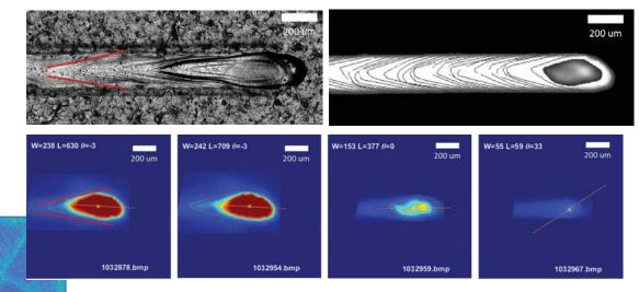
In-situ melt pool observation an analysis is mapped from tracks to layers
