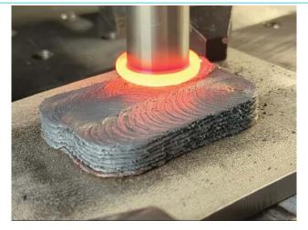
316-H bar stock deposited directly onto 316-L plate at PNNL
