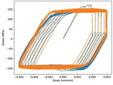
Example of mean prediction vs INL data for an arbitrary creepfatigue test (0.6% strain range, 10 minute hold, 950 C)
