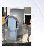
Tee Built using PBF 4" Diameter x 8" Tall ≅ 50 lbs. (Rolls-Royce)
