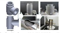
CAD to Part (Non-Symmetric) via Hybrid AM (Laser Hot Wire)
