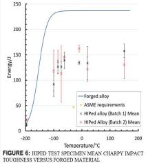
Oxide stripping process applied – equivalent toughness to forged material achieved for first time! 250J
