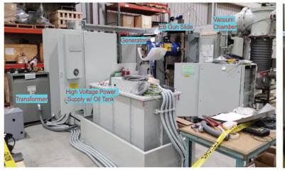
Elements of the EBW equipment set up at PTR
