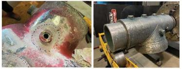
Piping components being printed at Lincoln Electric Additive Services
