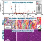
Multiscale characterization using XCT, EBSD and STEM-EDS reveals variations in porosity, grain structure, & nanoscale segregation as a function of varying processing parameters
