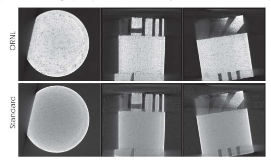
DL-reconstruction allows for resolving the flaws using 6X faster scans in thick dense 316L/H  $\,$
