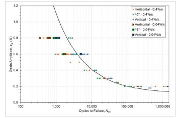
Fig 7: Additional In-air Fatigue Tests at 0.04%/S Strain rates under Ambient Conditions
