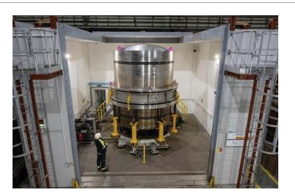
Third parties have independently carried out NDE with no recordable indications. All welds passed internal pressure vessel fabrications standards.
