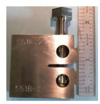
Bolt Loaded Compact Tension Specimens
