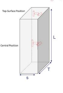
L-T-S orientation testing for Isotropy Assessment
