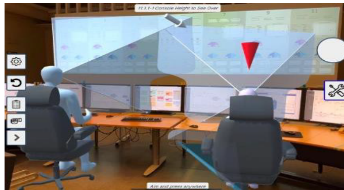
Figure 2-2 Evaluation of sightlines on the large screen, on-site in HAMMLAB using AR
