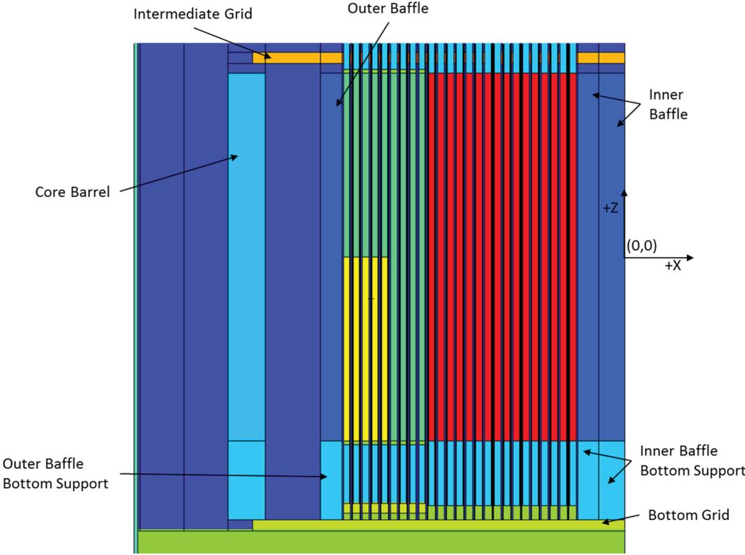
**Figure A-3 Horizontal Cross-Sectional View of the Inner and Outer Baffle of the Monte Carlo N-Particle Transport Code 6 Model of the Vulcain Experimental Nuclear Study 3 Benchmark**
