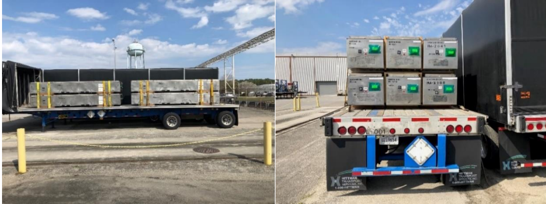
Figure 3-8 Unirradiated Boiling Water Reactor Fuel Shipment Using RAJ-II Packages. (Photos courtesy of Global Nuclear Fuels, General Electric)
