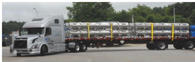
Figure 3-7 Unirradiated Pressurized Water Reactor Fuel Shipment Using Traveller Packages. (Source: Photo provided by the Westinghouse Electric Company, LLC [NRC 2022-TN8089])
