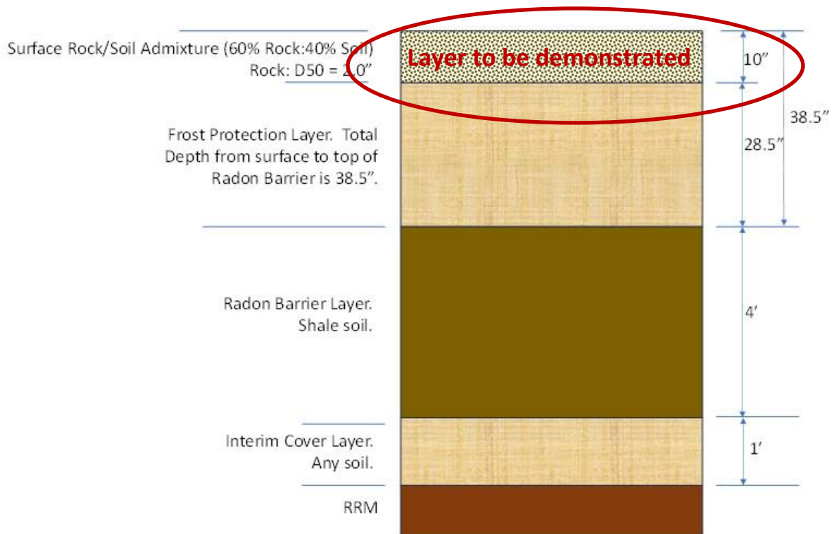
Figure 1. ET Cover Profile with Surface Admixture Layer
