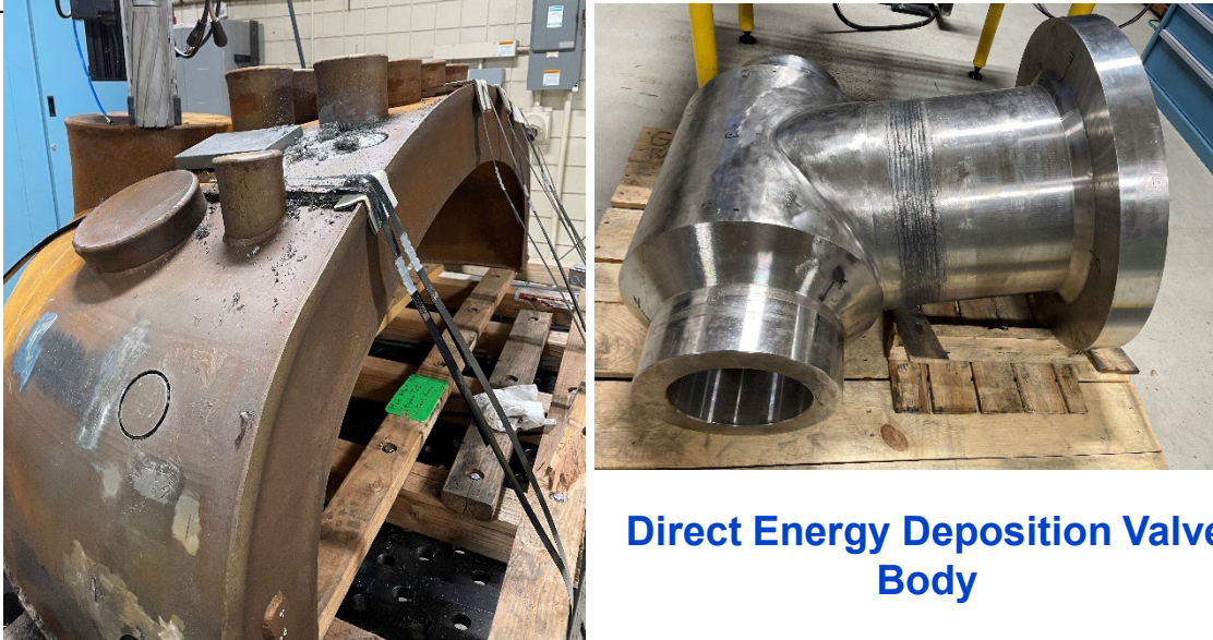
PM-HIP Scaled SMR Head and Valve body
