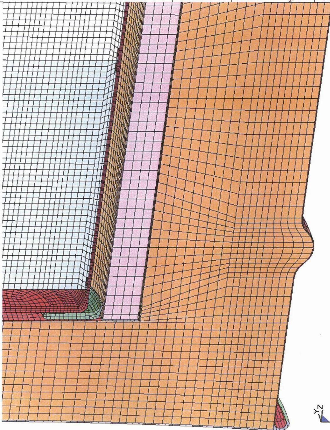
Figure 2.1.4 - Configuration of the HABC Analytical Model Near the Package Bottom
