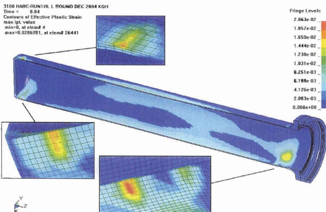
Figure 3.1.11 - HABC-run1hl, Crush Impact, Effective Plastic Strain in the CV Body
