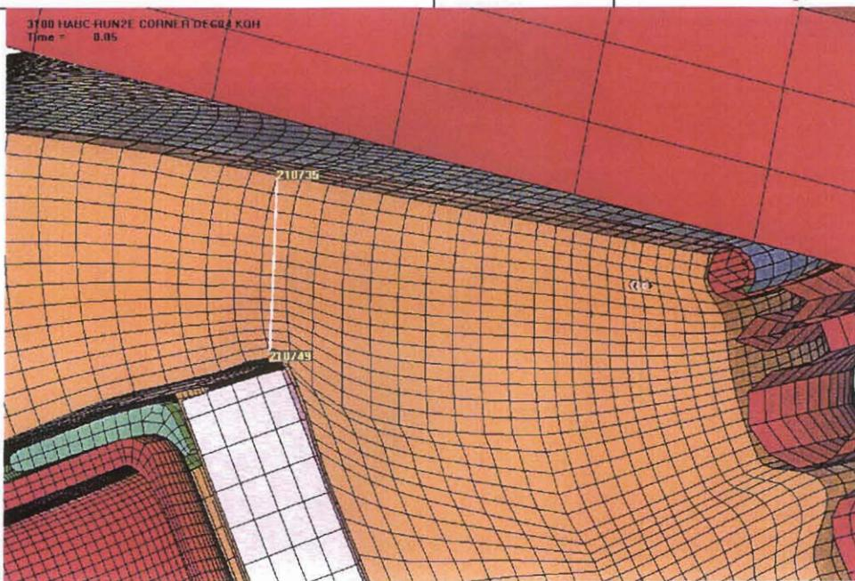
Figure 3.3.13 - HABC-run2e, Bottom Kaolite Thickness After the Crush Impact
