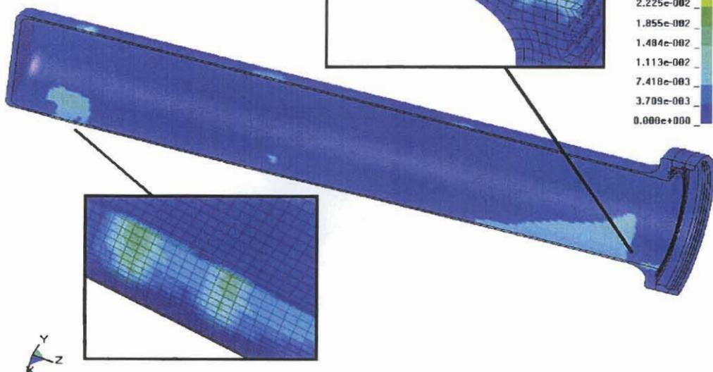
Figure 3.3.6 - HABC-run2e, Crush Impact, Effective Plastic Strain in the CV Body
