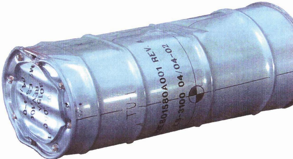
Figure 3.7.1.3 - TU1, View of Crush Damage with the Crush Side Up
