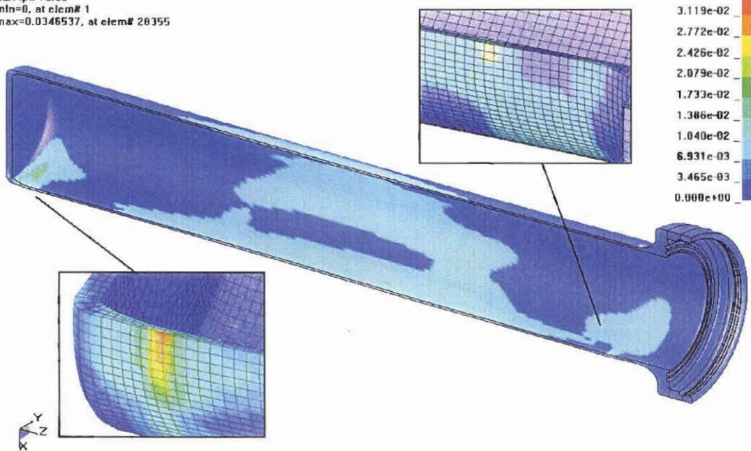
Figure 3.2.6 - HABC-run1hh, 30-Foot Impact, Effective Plastic Strain in the CV Body
