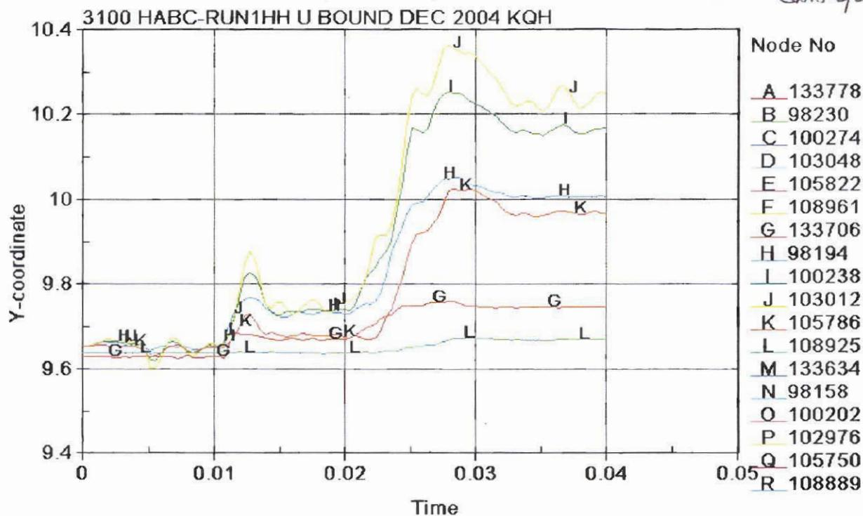
Figure 3.2.17 - HABC-run1hh, Drum Diameter Time History in the Y Direction
