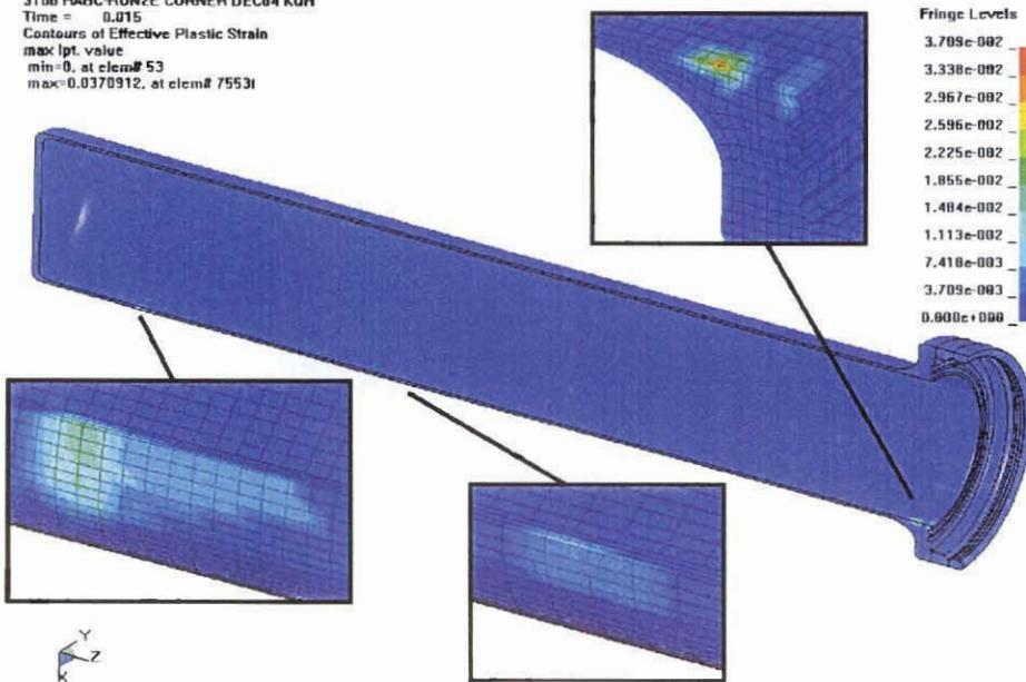
Figure 3.3.2 - HABC-run2e, 30-Foot Impact, Effective Plastic Strains in the CV Body
