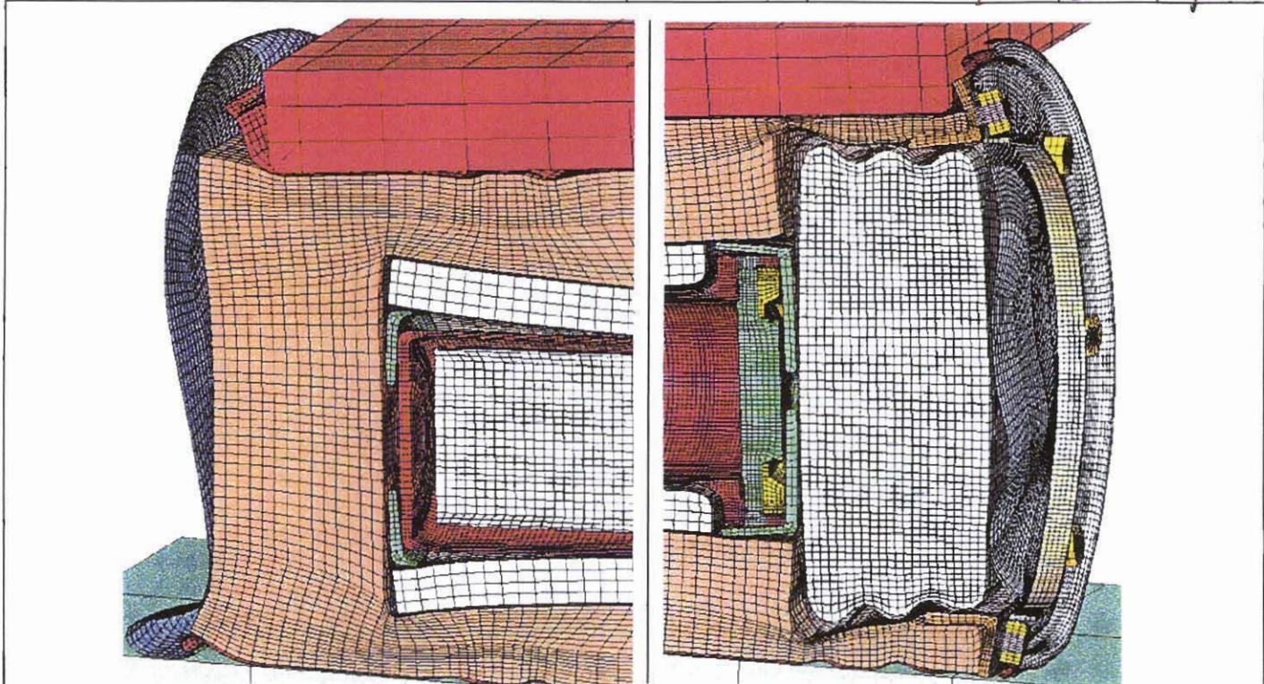
Figure 3.1.10 - HABC-run1hl, Crush Impact, Configuration of the Lid and Bottom
