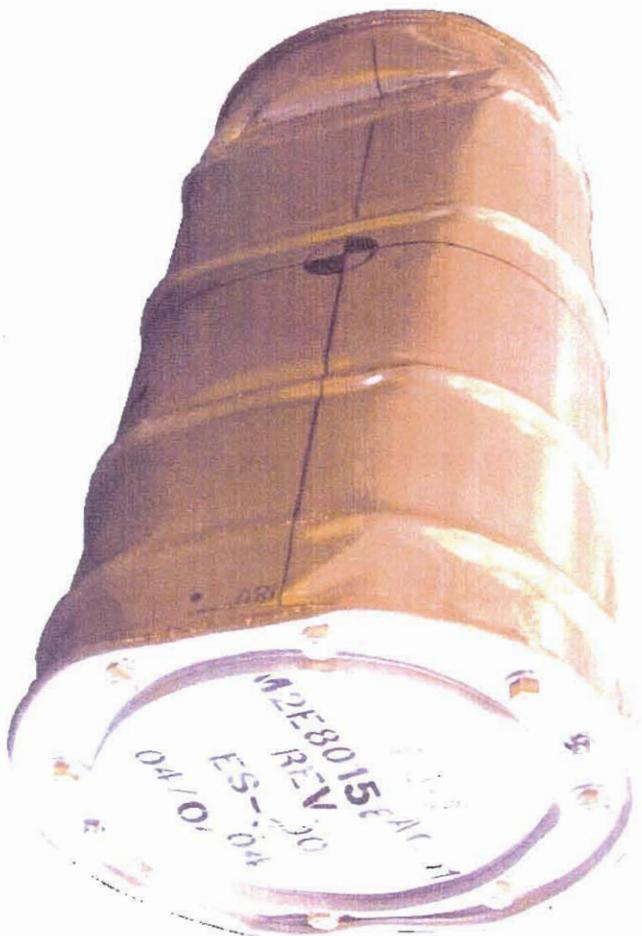
Figure 3.7.4.3 - TU2, Cumulative Damage After the Punch Impact, Crush Plate Side
