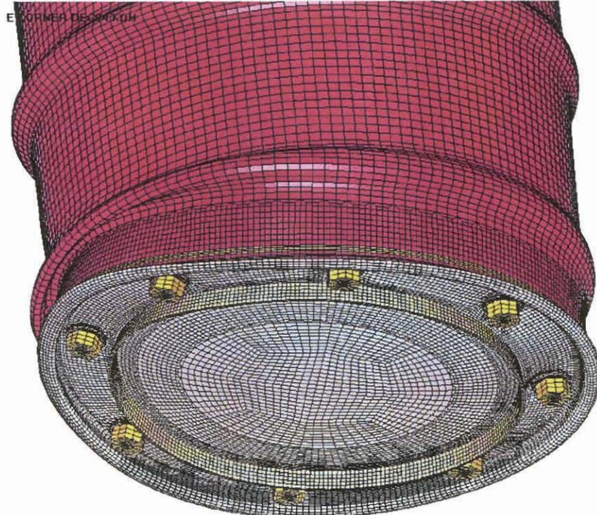
Figure 3.7.2.2 - HABC-run2e, Deformed Shape After the 30-foot Impact
