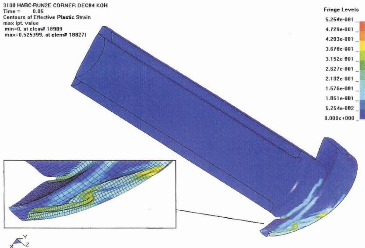
Figure 3.3.9 - HABC-run2e, Crush Impact, Effective Plastic Strain in the Liner
