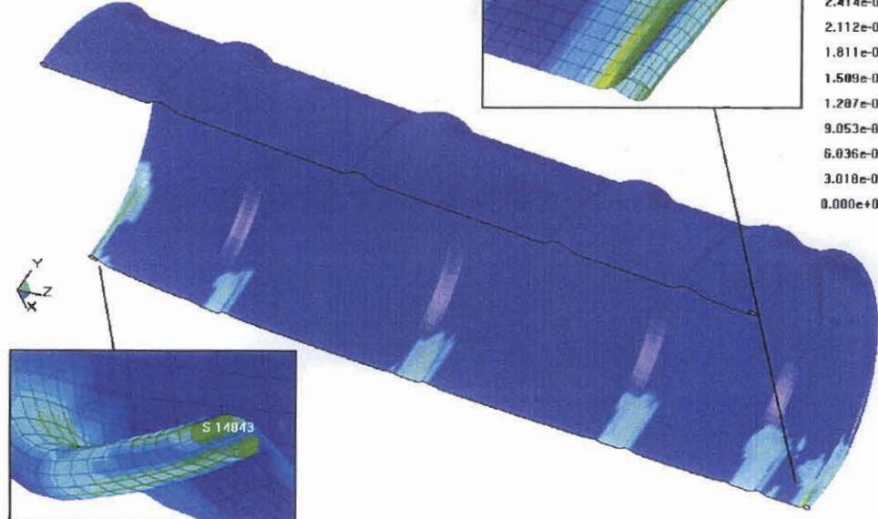
Figure 3.5.5 - HABC-run4g, 30-Foot Impact, Effective Plastic Strain in the Drum
