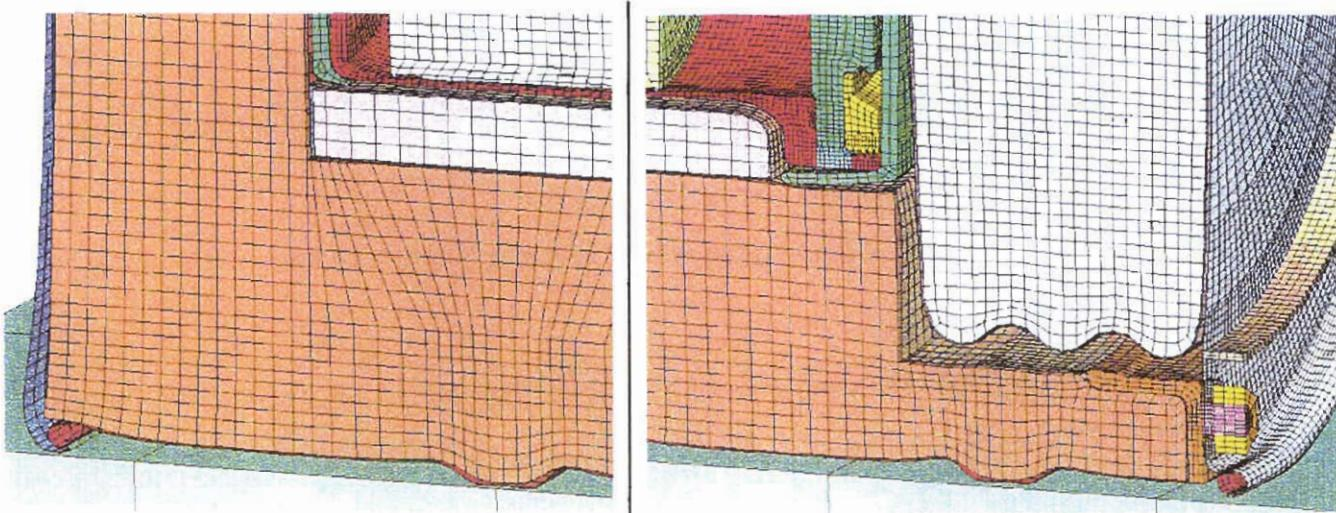
Figure 3.2.2 - HABC-run1hh, 4-Foot Impact, Configuration of the Lid and Bottom
