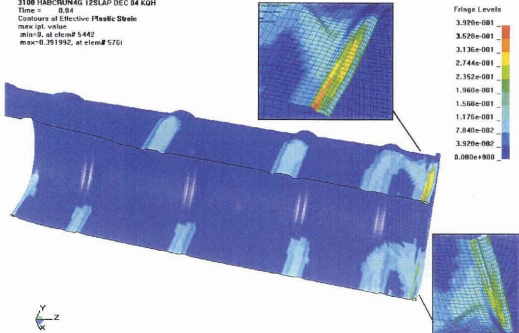
Figure 3.5.11 - HABC-run4g, Crush Impact, Effective Plastic Strain in the Drum
