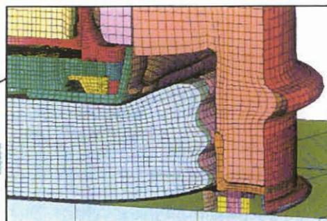
Figure 3.4.5 - HABC-run3b, Configuration After the Crush Impact
