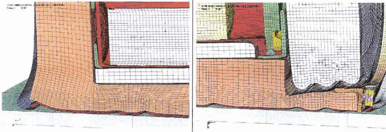
Figure 3.1.6 - HABC-run1hl, 30-Foot Impact, Configuration of the Lid and Bottom
