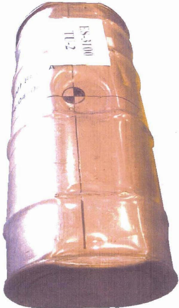
Figure 3.7.4.1 - TU2, Cumulative Damage After the Punch Impact, Rigid Surface Side
