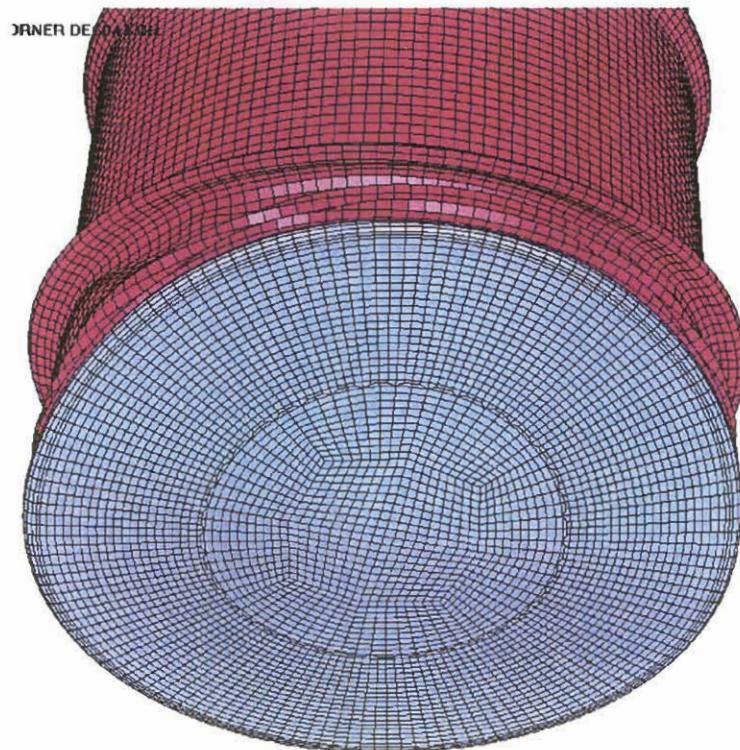
Figure 3.7.2.4 - HABC-run2e, Damage to the Bottom Head in the Crush Impact
