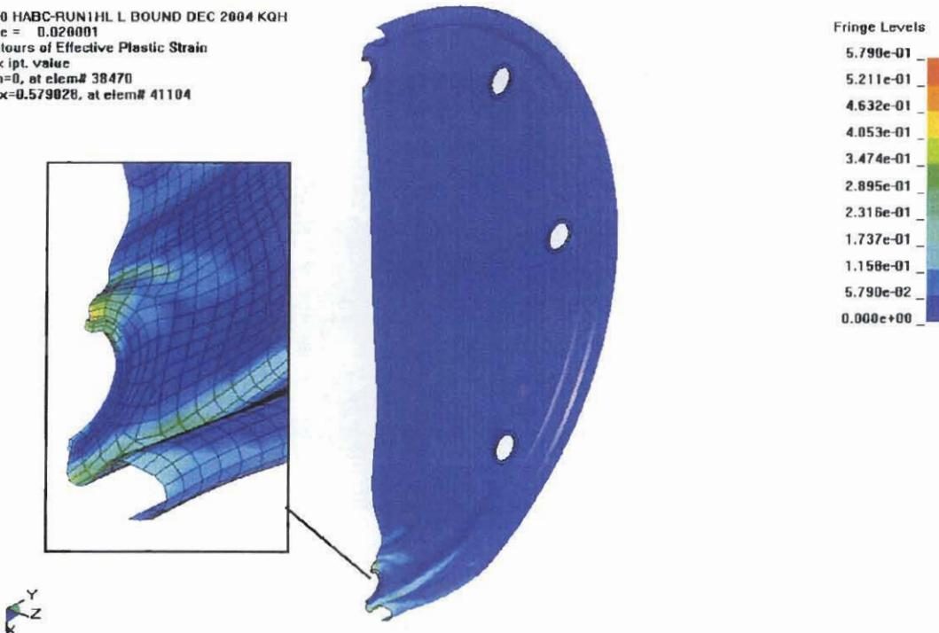
Figure 3.1.8 - HABC-run1hl, 30-Foot Impact, Effective Plastic Strain in the Lid
