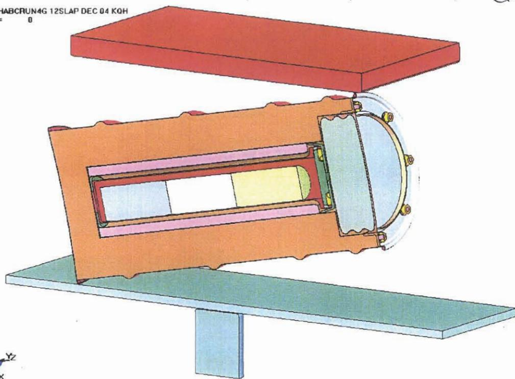
Figure 3.5.1 - HABC-run4g, 12 Degree Slapdown Initial Configuration
