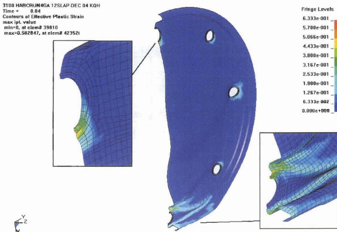
Figure 3.6.6 - HABC-run4ga, Crush Impact, Effective Plastic Strain in the Lid
