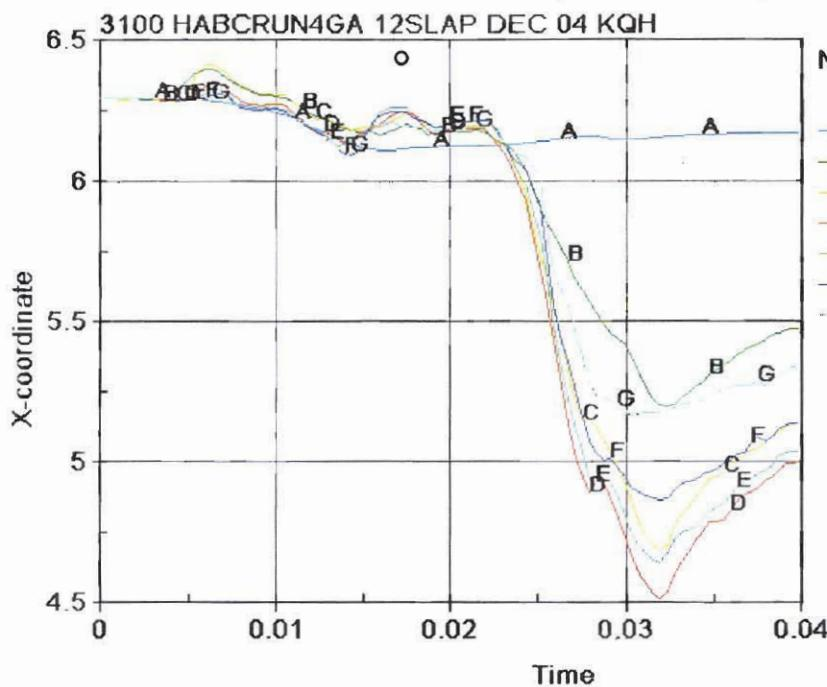
Figure 3.6.11 - HABC-run4ga, Diameter Time History for the Inner Liner
