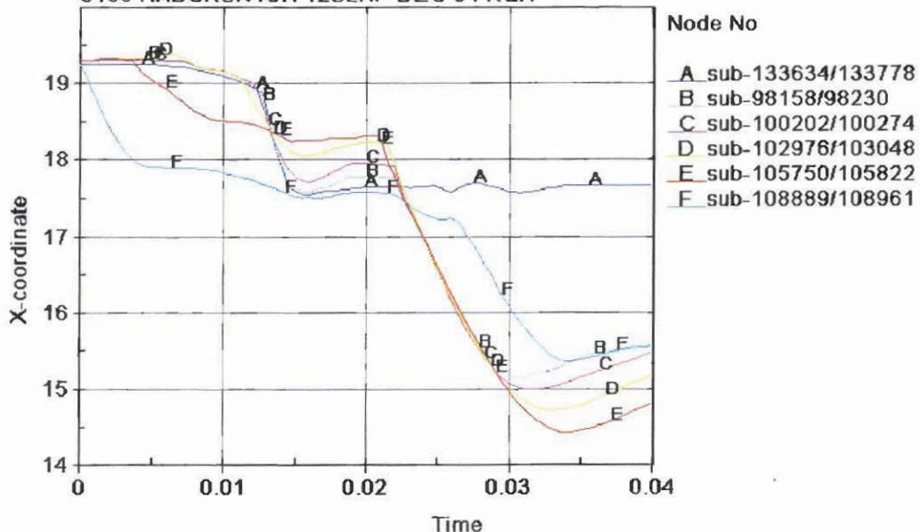
Figure 3.6.9 - HABC-run4ga, Diameter Time History for the Drum in the X Direction
