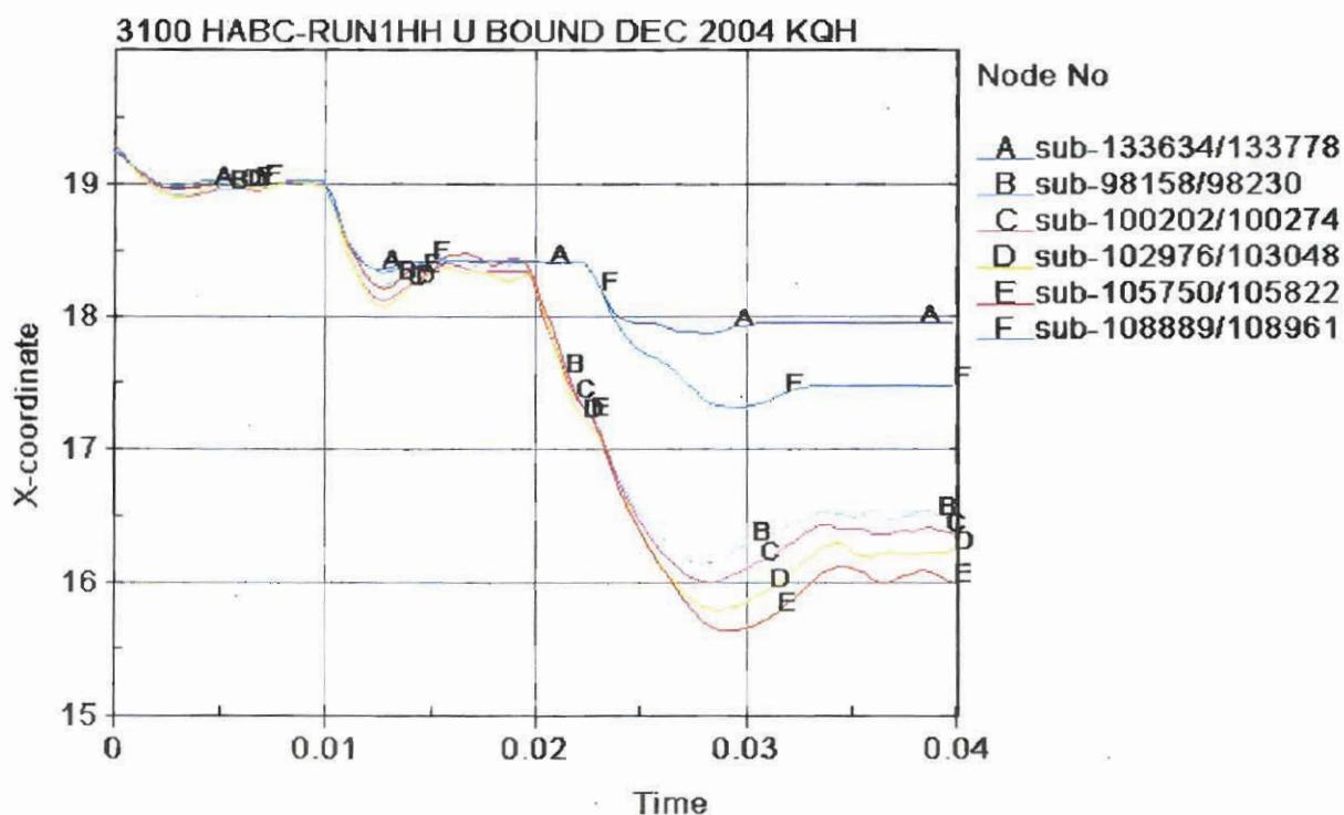
Figure 3.2.16 - HABC-run1hh, Drum Diameter Time History in the X Direction
