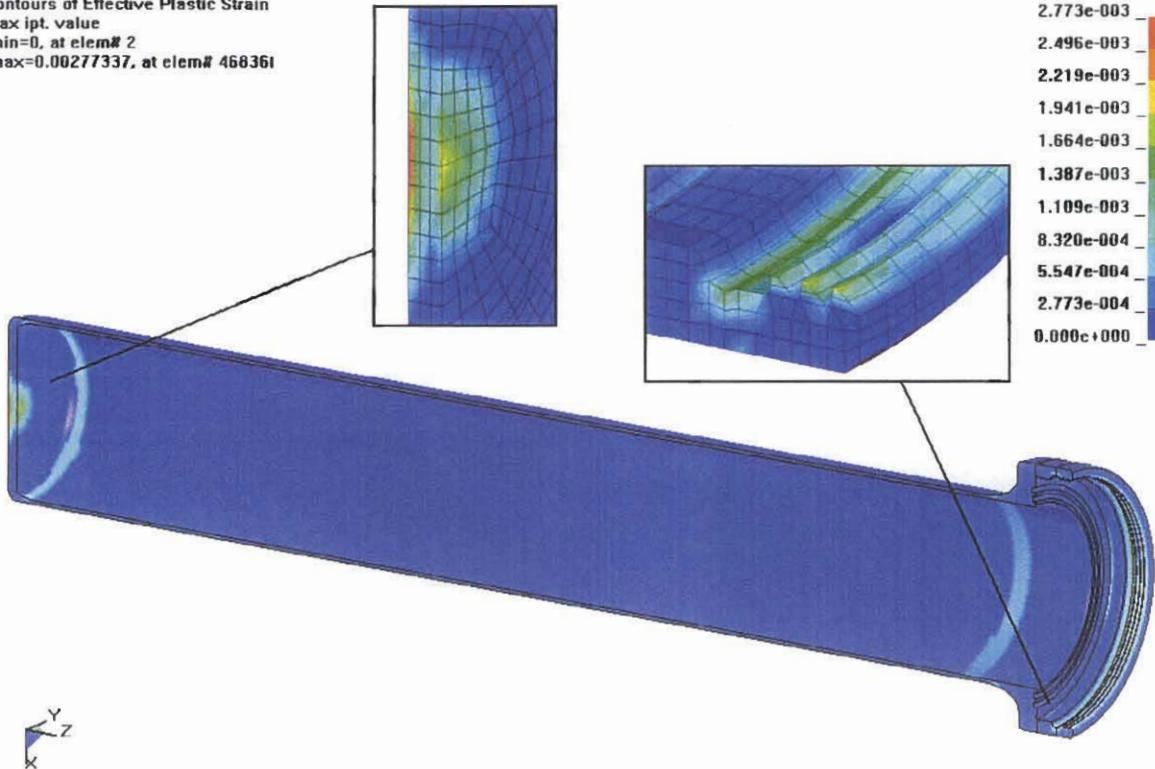
Figure 3.4.2 - HABC-run3b, 30-Foot Impact, Effective Plastic Strain in the CV Body
