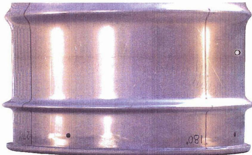
Figure 3.7.3.1 - TU4, 4-Foot + 30-Foot Impact Damage
