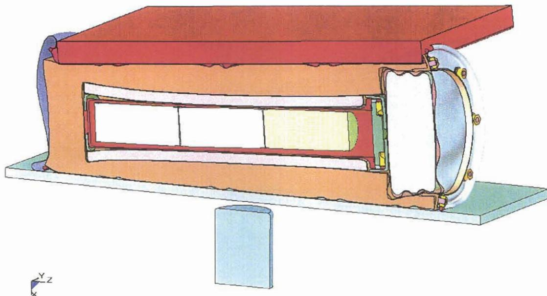
Figure 3.1.9 - HABC-run1hl, Crush Impact, Final Configuration
