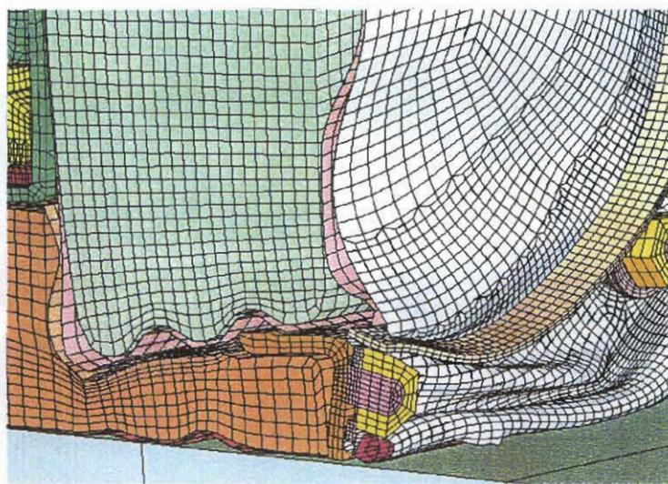
Figure 3.5.9 - HABC-run4g, Crush Impact, Enlarged Views of the Resulting Configuration
