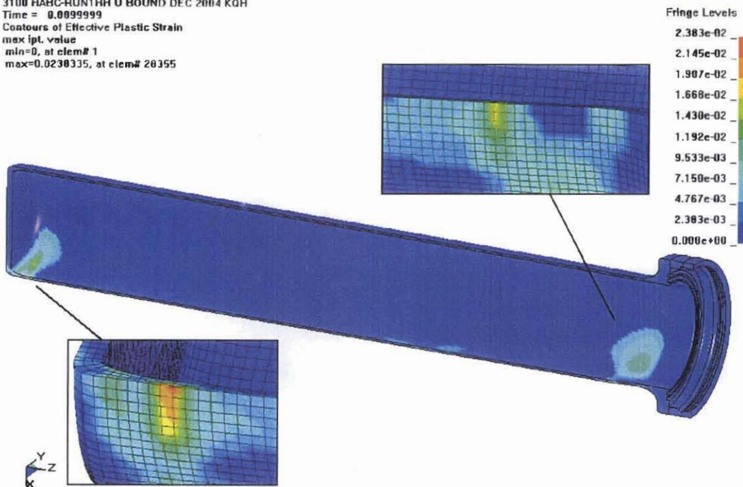
Figure 3.2.3 - HABC-run1hh, 4-Foot Impact, Effective Plastic Strain in the CV Body
