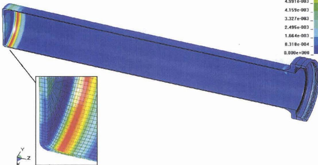
Figure 3.4.6 - HABC-run3b, Crush Impact, Effective Plastic Strain in the CV Body
