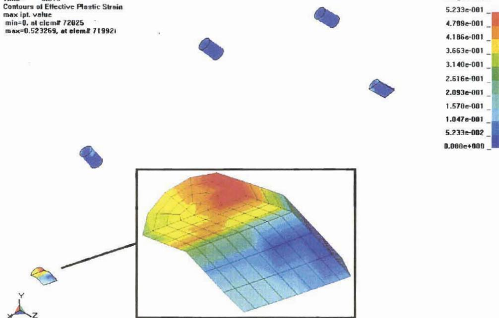
Figure 3.3.4 - HABC-run2e, 30-Foot Impact, Effective Plastic Strain in the Studs
