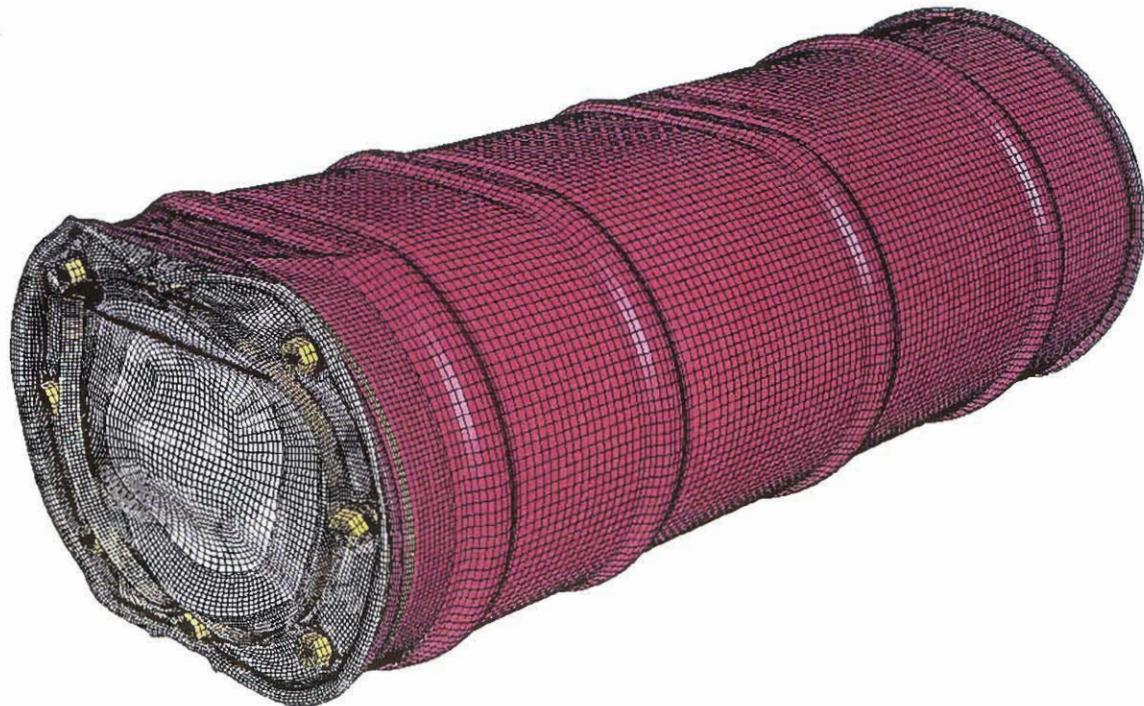
Figure 3.7.1.4 - HABC-run4g, View of the Crush Damage, Crush Side Up
