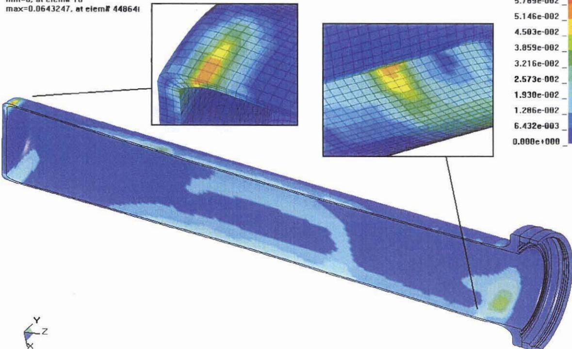
Figure 3.6.4 - HABC-run4ga, Crush Impact, Effective Plastic Strain in the CV Body
