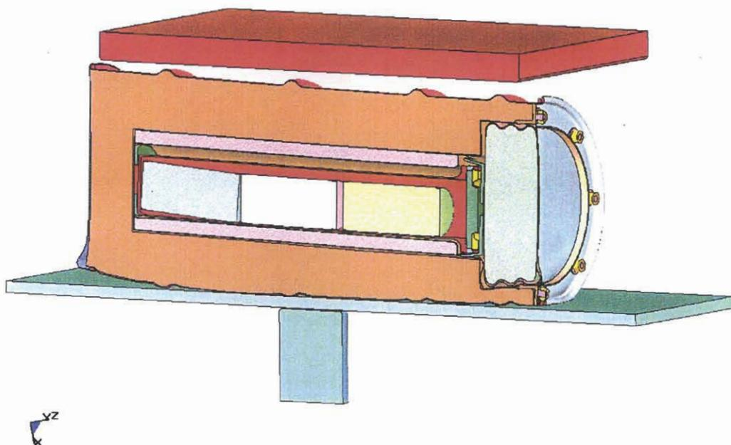
Figure 3.6.1 - HABC-run4ga, Initial Configuration for the Centered Crush Impact
