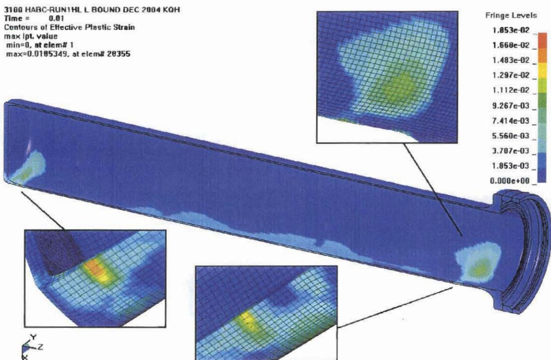
Figure 3.1.4 - HABC-run1hl, 4-Foot Impact, Effective Plastic Strain in the CV Body
