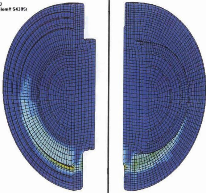
Figure 3.3.3 - HABC-run2e, 30-Foot Impact, Effective Plastic Strain in the CV Body
