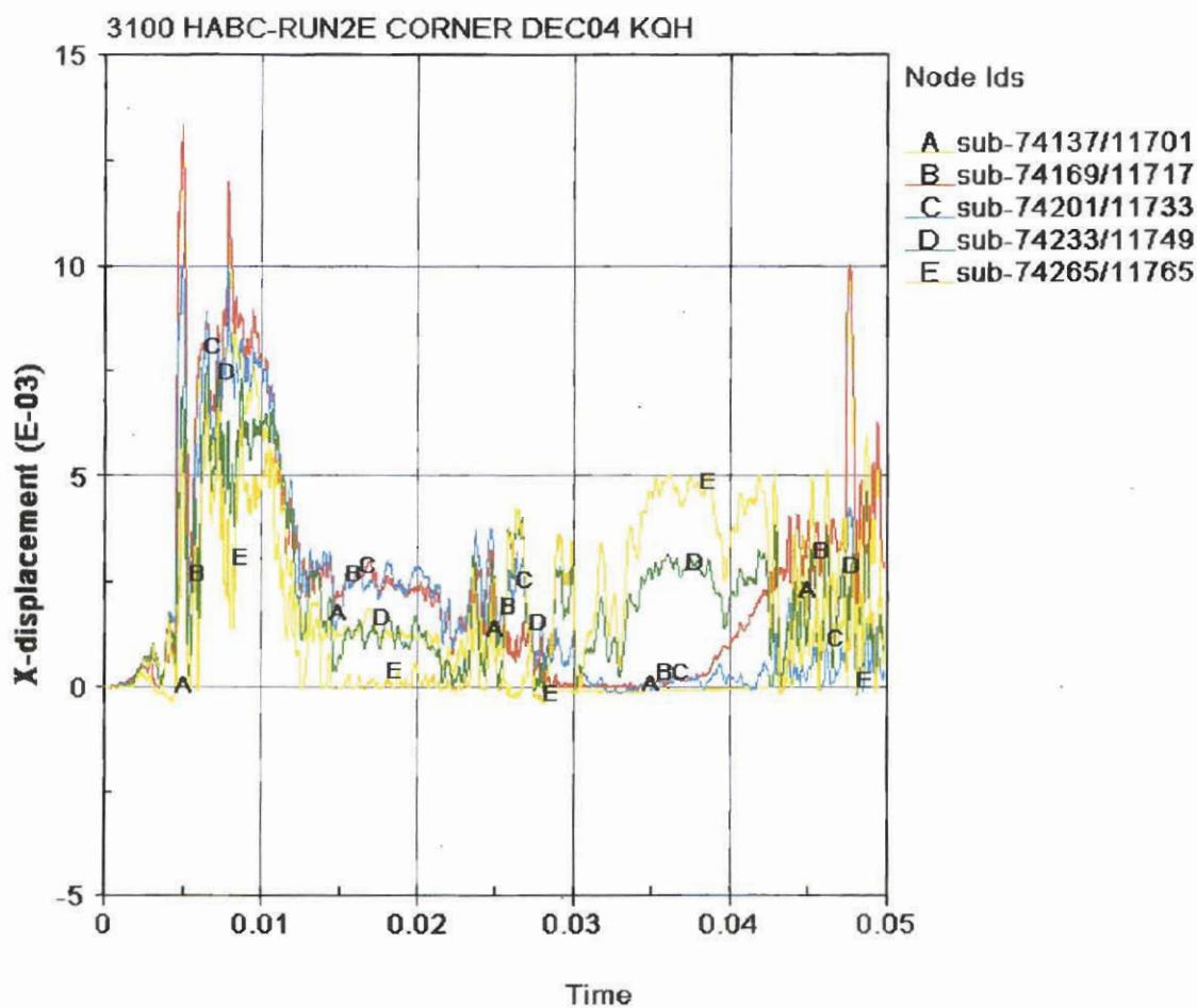
Figure 3.3.10 - HABC-run2e, Crush Impact, CV Lid/Body Separation Time History
