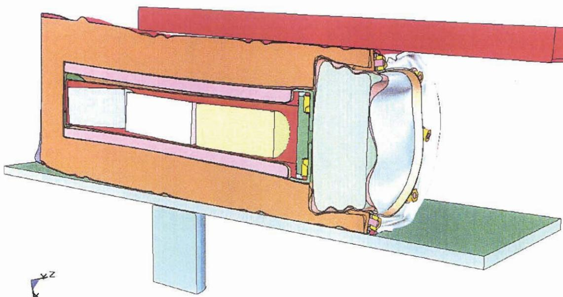
Figure 3.5.8 - HABC-run4g, Final Configuration After the Offset Crush Impact
