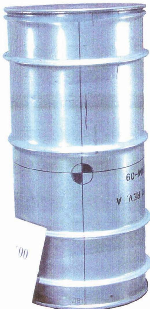
Figure 3.7.3.3 - TU4, Crush Damage
