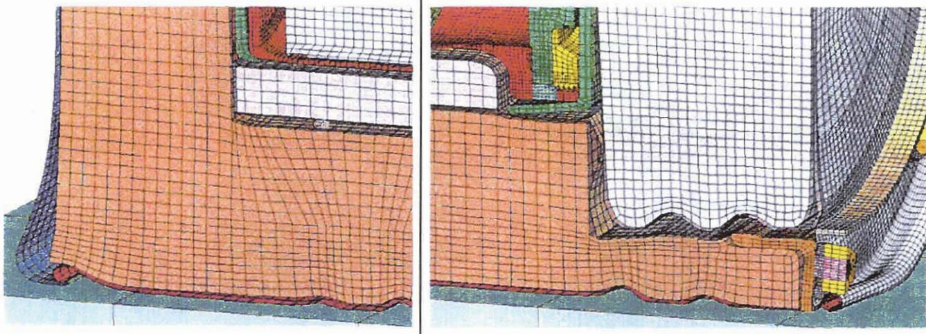
Figure 3.2.5 - HABC-run1hh, 30-Foot Impact, Configuration of the Lid and Bottom
