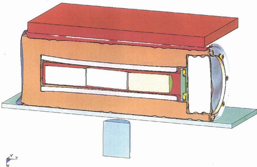
Figure 3.2.8 - HABC-run1hh, Configuration After the Crush Impact
