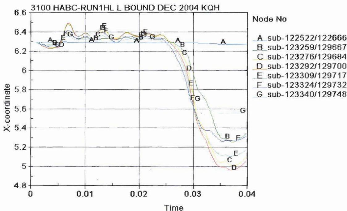
Figure 3.1.20 - HABC-run1hl, Diameter Changes in the Inner Liner
