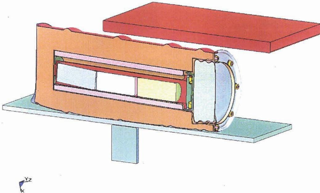
Figure 3.5.7 - HABC-run4g, Initial Configuration of the Offset Crush Impact
