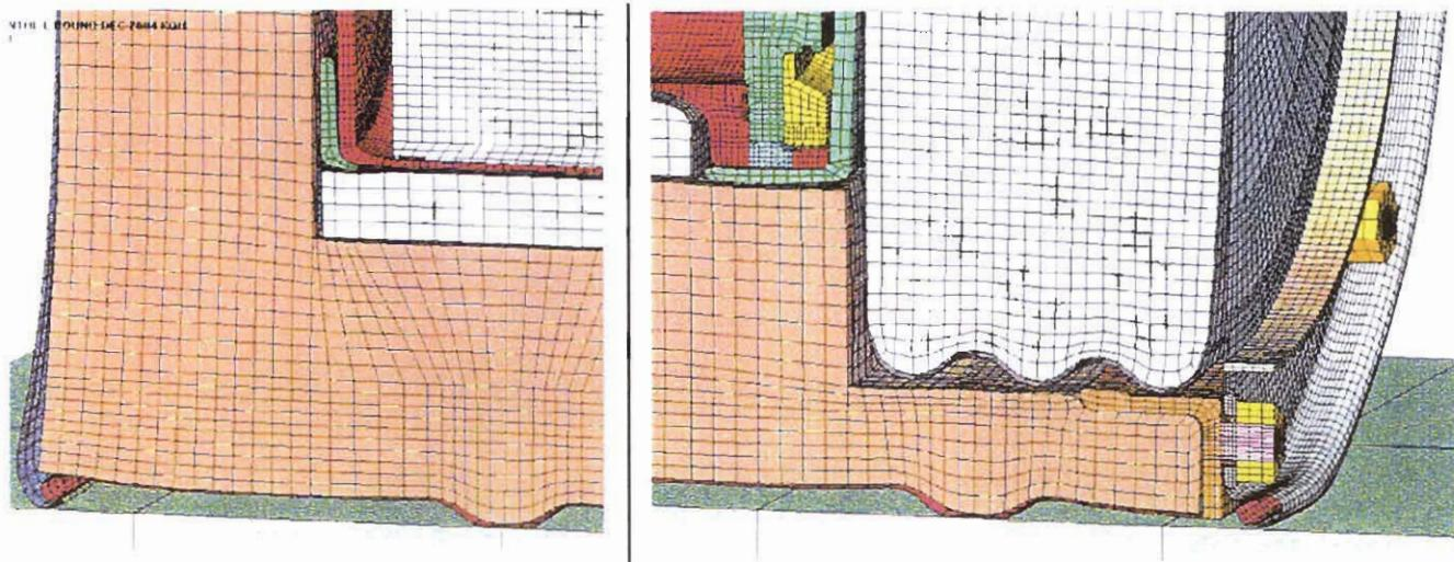
Figure 3.1.3 - HABC-run1hl, 4-Foot Impact, Configuration in the Lid and Bottom
