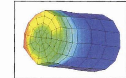
Figure 3.5.13 - HABC-run4g, Crush Impact, Effective Plastic Strain in the Studs
