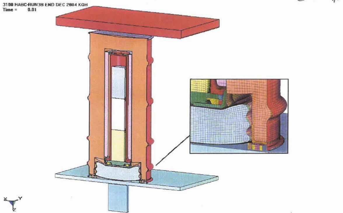
Figure 3.4.1 - HABC-run3b, Configuration After the 30-Foot Impact
