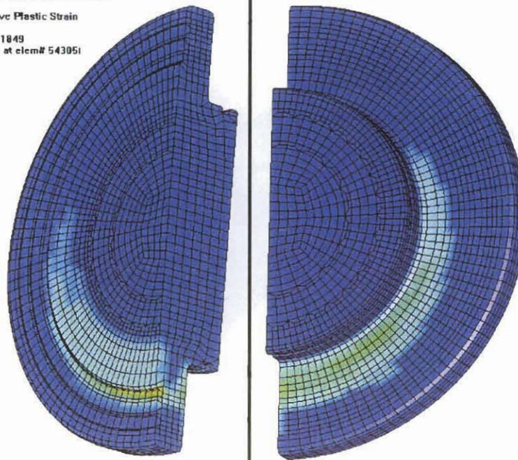
Figure 3.3.7 - HABC-run2e, Crush Impact, Effective Plastic Strain in the CV Lid
