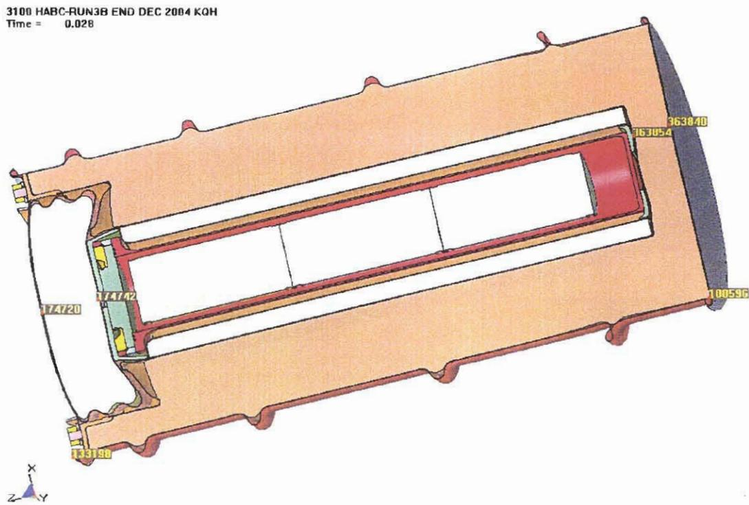
Figure 3.4.8 - HABC-run3b, Nodes to Determine Drum/Kaolite Heights
