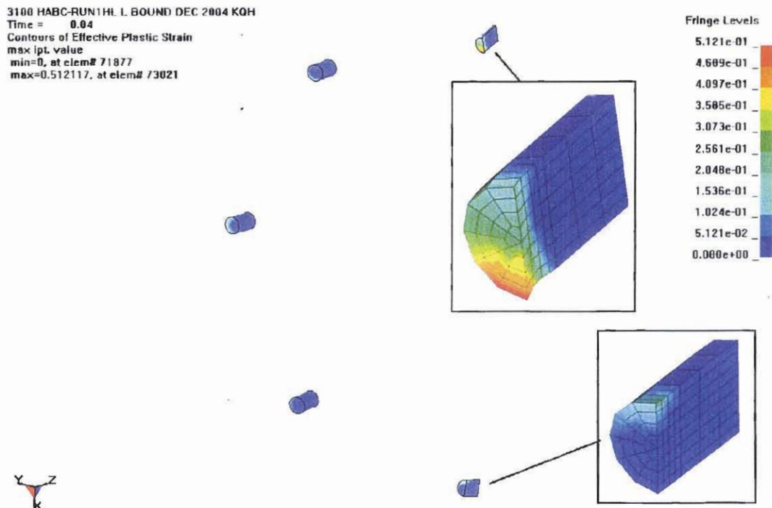
Figure 3.1.14 - HABC-run1hl, Crush Impact, Effective Plastic Strain in the Studs
