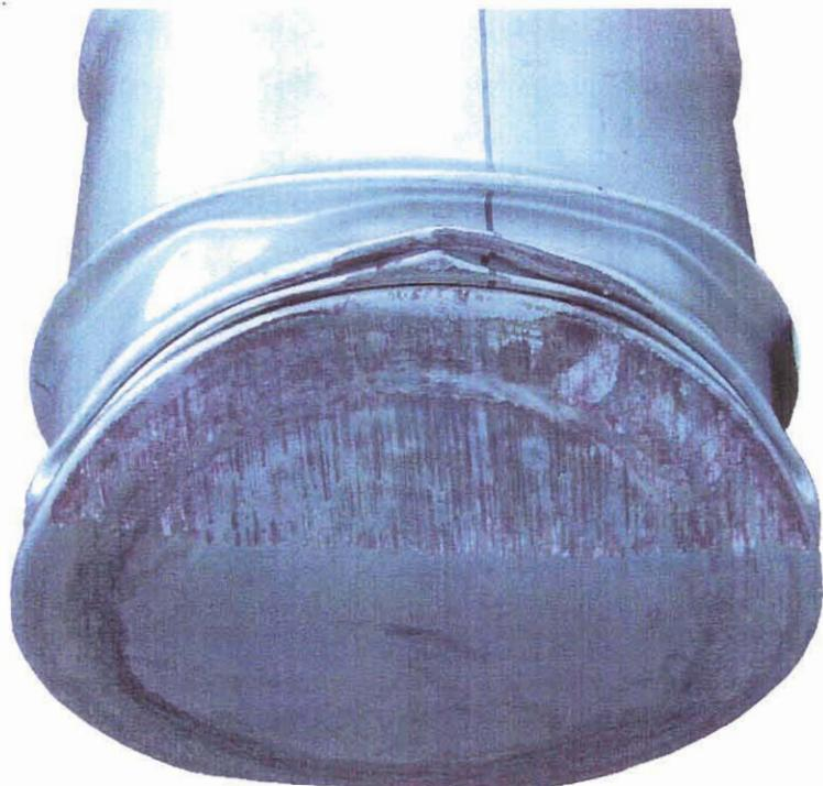
Figure 3.7.2.3 - TU3, Damage to the Bottom Head in the Crush Impact
