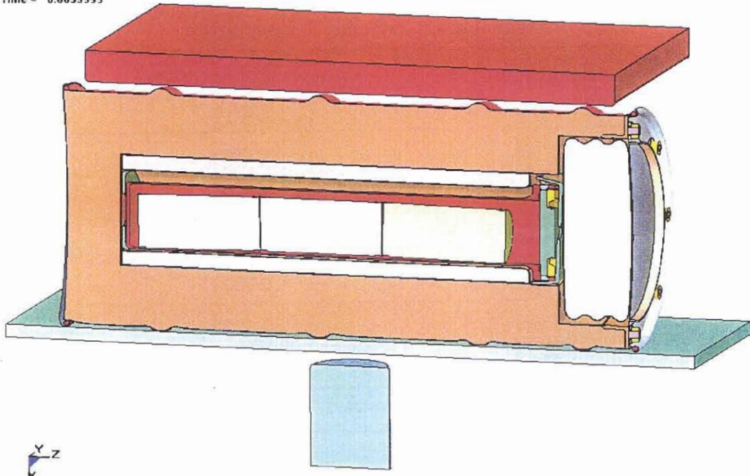
Figure 3.2.1 - HABC-run1hh, Configuration After the 4-Foot Impact
