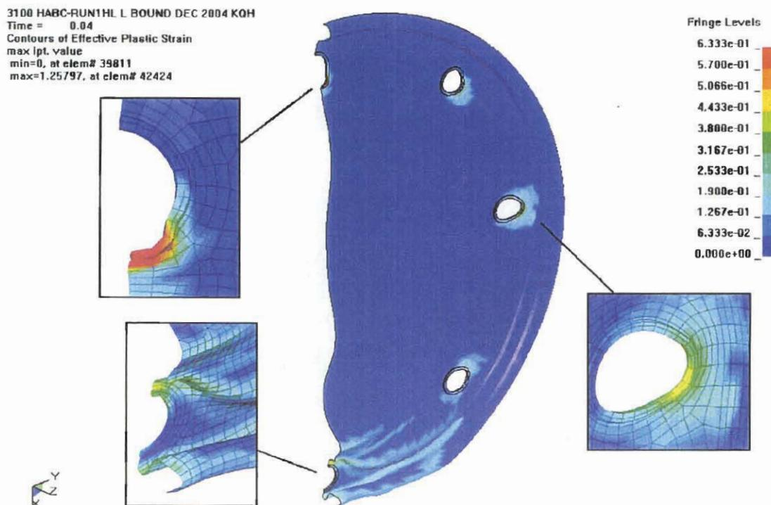
Figure 3.1.13 - HABC-run1hl, Crush Impact, Effective Plastic Strain in the Lid
