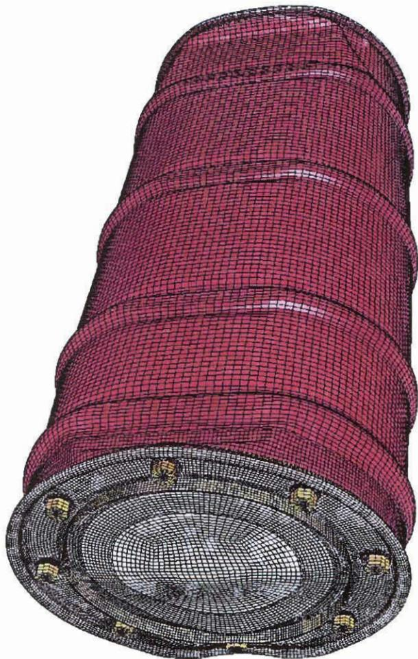
Figure 3.7.4.4 - HABC-run1hh, Cumulative Damage, Crush Plate Side
