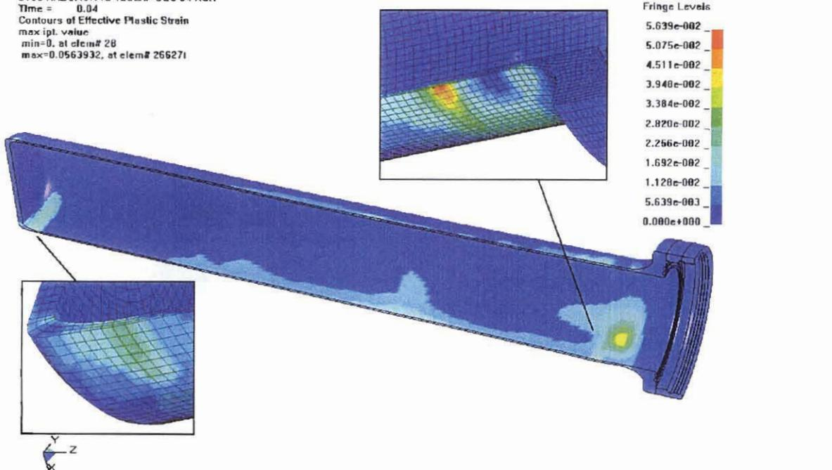
Figure 3.5.10 - HABC-run4g, Crush Impact, Effective Plastic Strain in the CV Body
