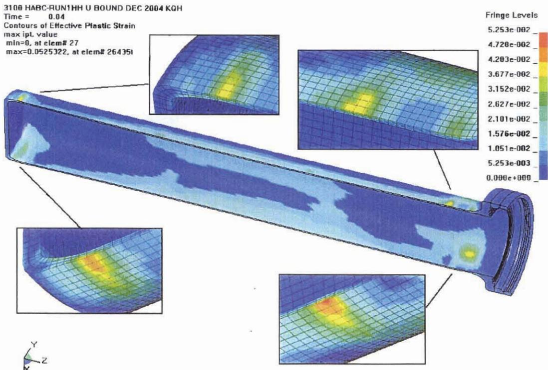
Figure 3.2.10 - HABC-run1hh, Crush Impact, Effective Plastic Strain in the CV Body
