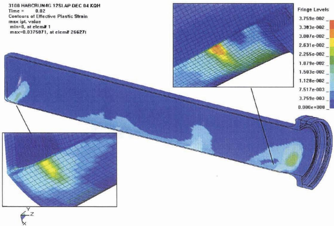
Figure 3.5.4 - HABC-run4g, 30-Foot Impact, Effective Plastic Strain in the CV Body
