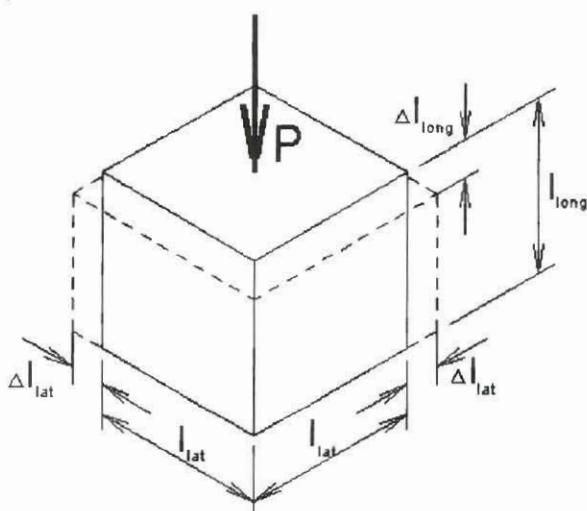
Figure 2.2.1.1 - Assumed Response of a Unit Cube
