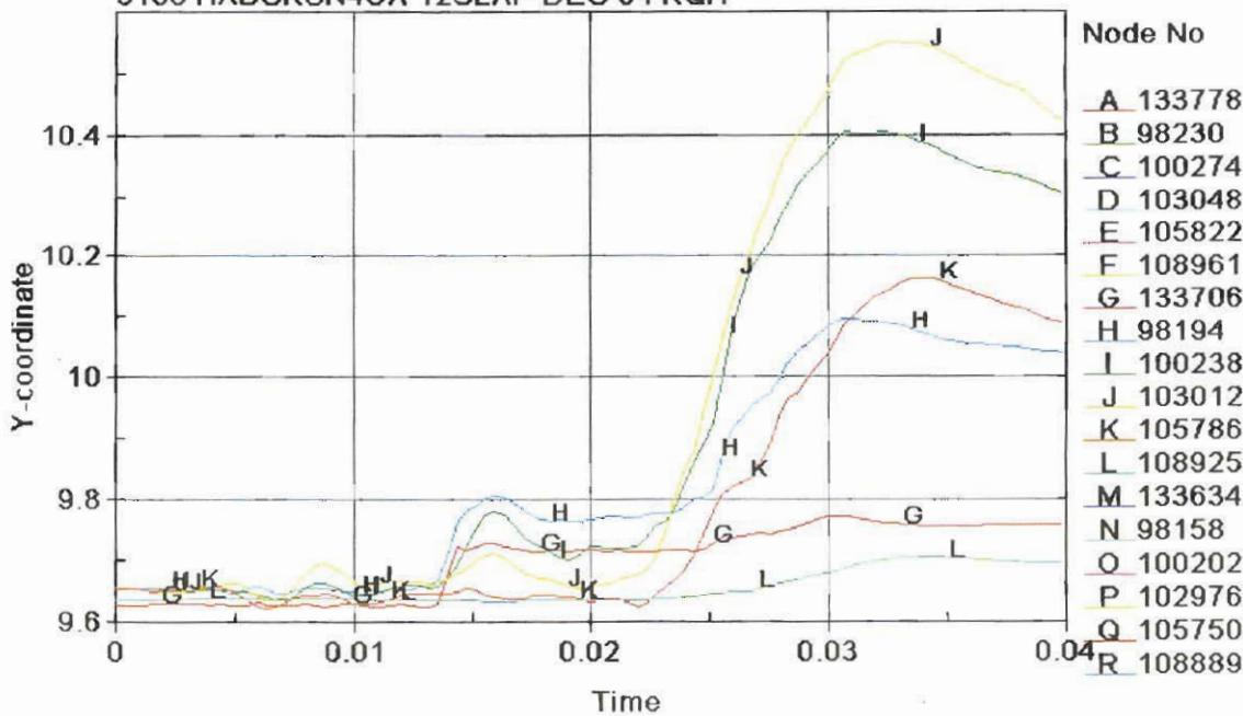
Figure 3.6.10 - HABC-run4ga, Radius Time History for the Drum in the Y Direction
