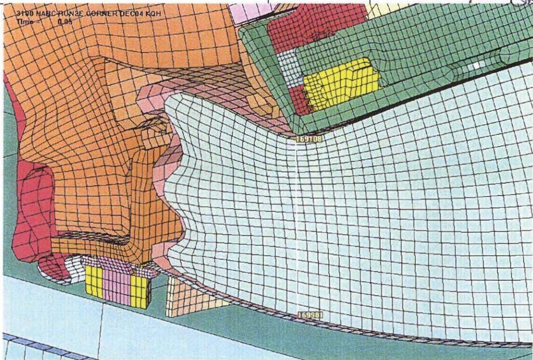
Figure 3.3.11 - HABC-run2e, Plug Thickness After the Crush Impact
