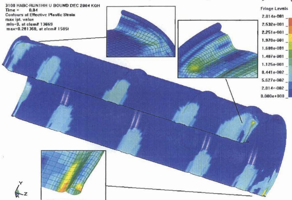
Figure 3.2.11 - HABC-run1hh, Crush Impact, Effective Plastic Strain in the Drum
