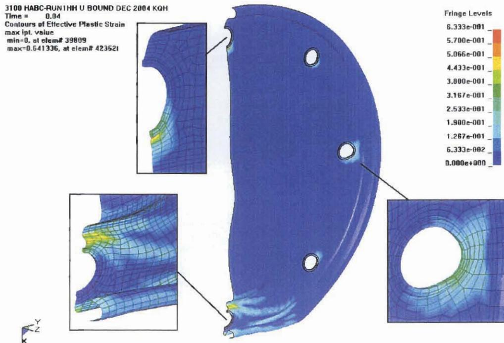
Figure 3.2.12 - HABC-run1hh, Crush Impact, Effective Plastic Strain in the Lid
