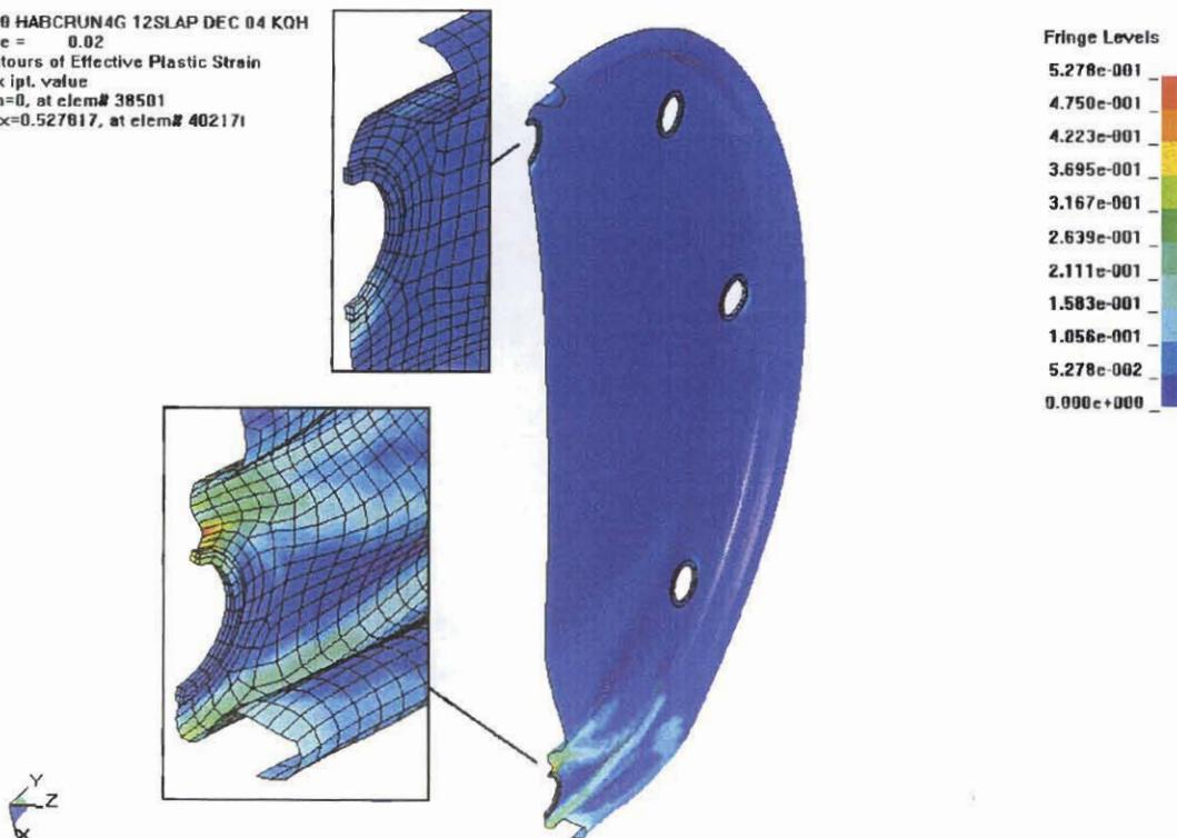
Figure 3.5.6 - HABC-run4g, 30-Foot Impact, Effective Plastic Strain in the Lid
