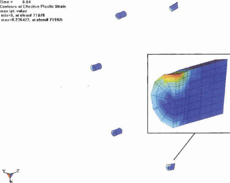
Figure 3.2.13 - HABC-run1hh, Crush Impact, Effective Plastic Strain in the Studs
