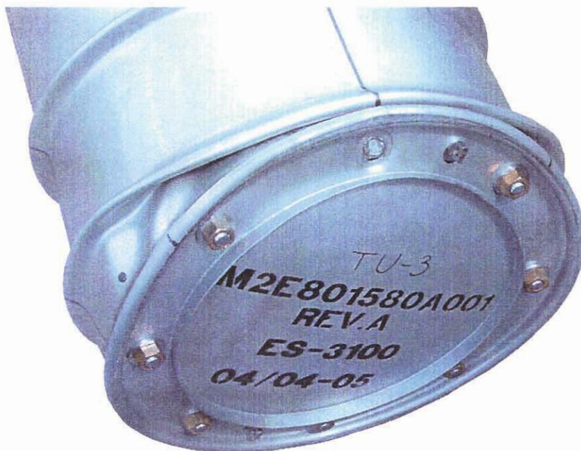
Figure 3.7.2.5 - TU3, Lid Damage from the Crush Impact
