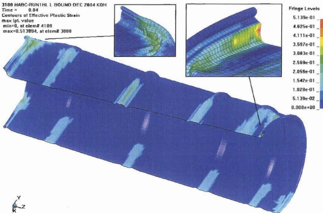
Figure 3.1.12 - HABC-run1hl, Crush Impact, Effective Plastic Strain in the Drum
