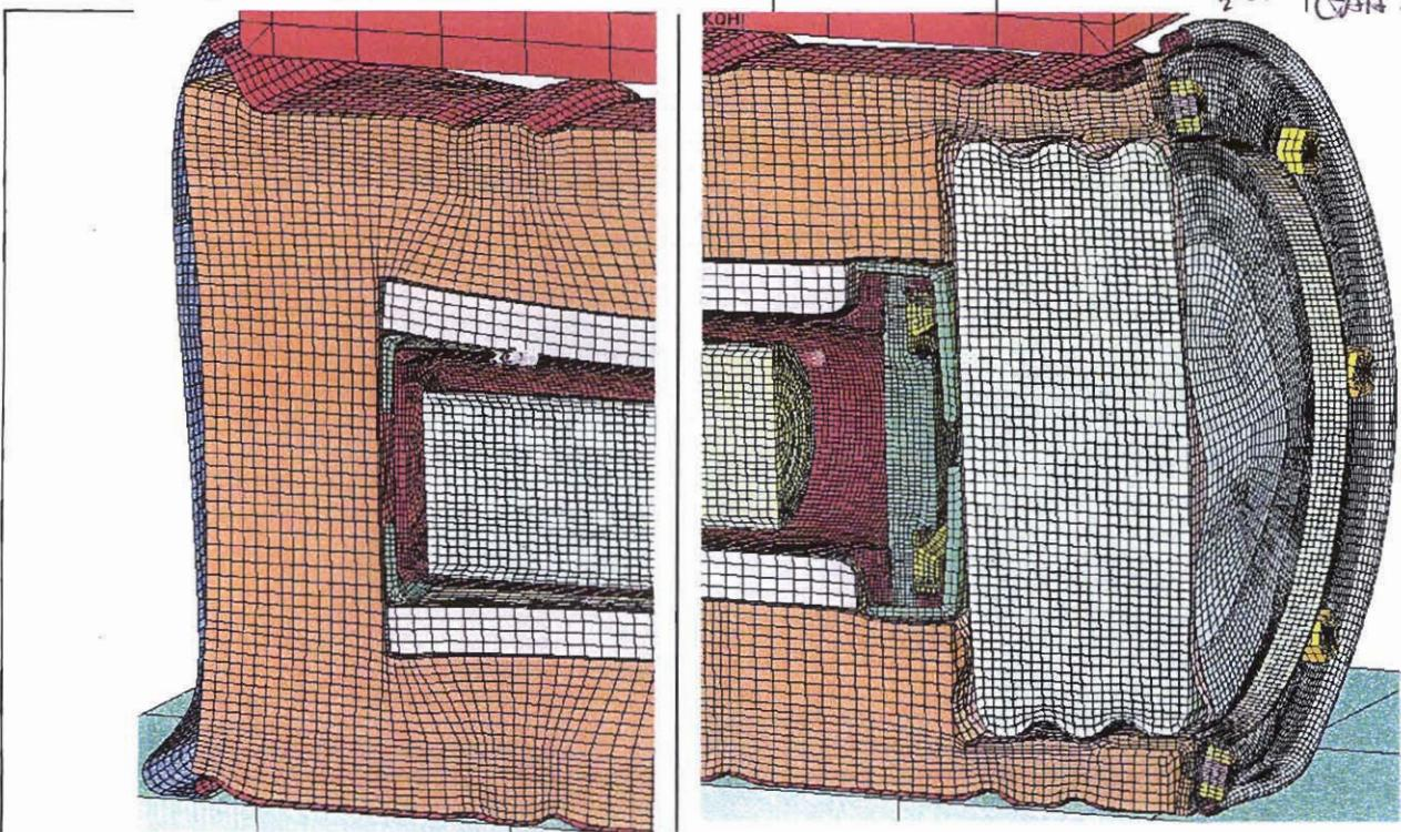
Figure 3.2.9 - HABC-run1hh, Crush Impact, Configuration of the Lid and Bottom
