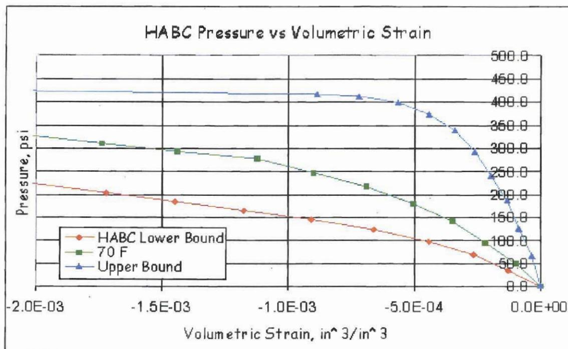
Figure 2.2.3.1 - Volumetric Strain vs Pressure Curves for the HABC Material
