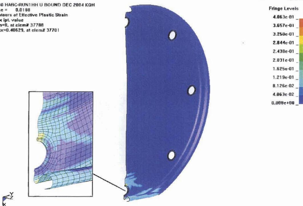
Figure 3.2.7 - HABC-run1hh, 30-Foot Impact, Effective Plastic Strain in the Lid
