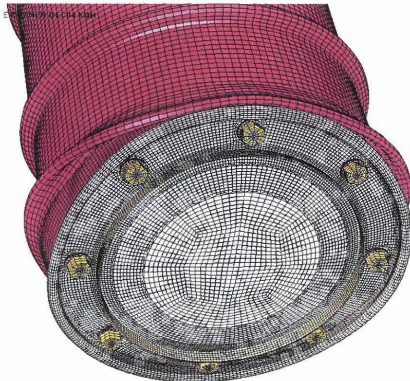
Figure 3.7.2.6 - HABC-run2e, Damage to the Bottom Head from the Crush Impact
