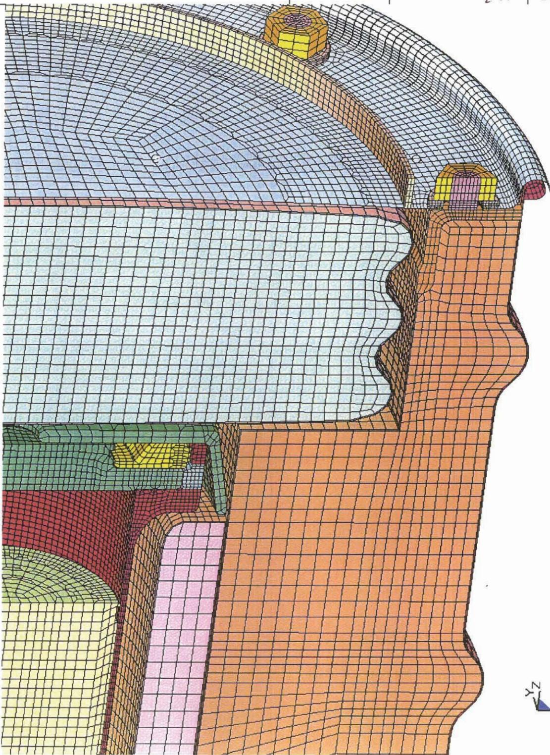
Figure 2.1.3 - Configuration of the HABC Analytical Model Near the Package Top
