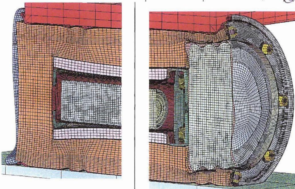
Figure 3.6.3 - HABC-run4ga, Crush Impact, Configurations at the Package Ends
