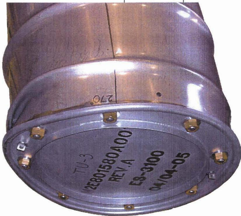
Figure 3.7.2.1 - TU3, Deformed Shape After the 30-Foot Impact
