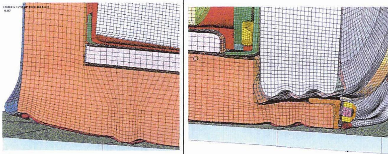
Figure 3.5.3 - HABC-run4g, 30-Foot Impact, Bottom and Lid Configurations
