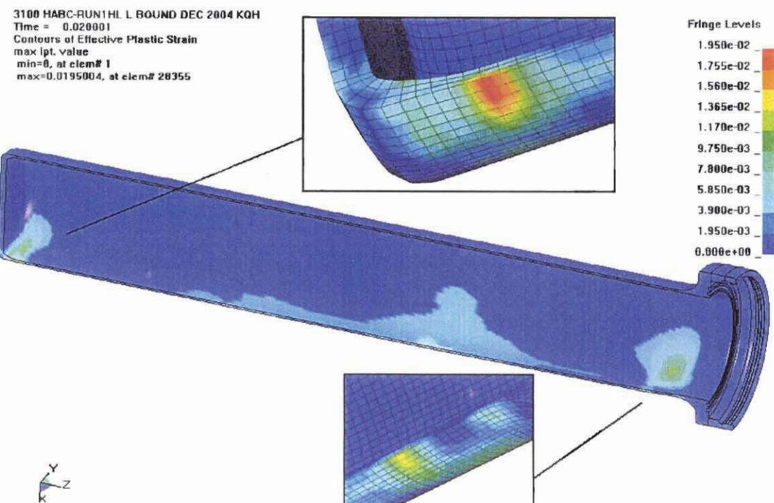
Figure 3.1.7 - HABC-run1hl, 30-Foot Impact, Effective Plastic Strain in the CV Body
