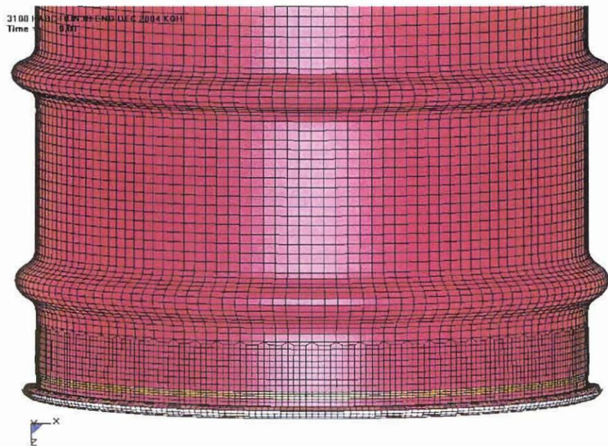
Figure 3.7.3.2 - HABC-Run3b, 30-Foot Impact Damage
