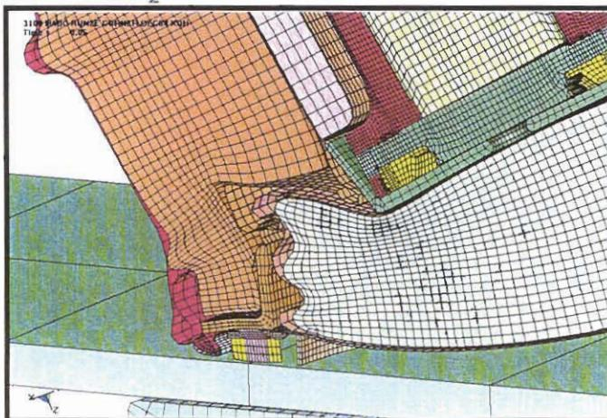
Figure 3.3.5 - HABC-run2e, Configuration After the Crush Impact
