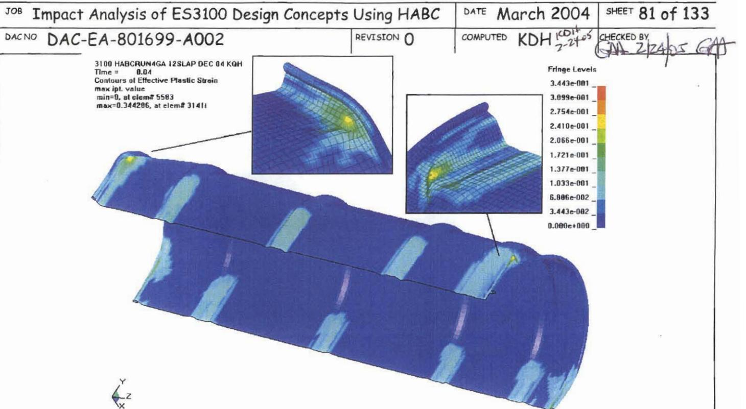
Figure 3.6.5 - HABC-run4ga, Crush Impact, Effective Plastic Strain in the Drum
