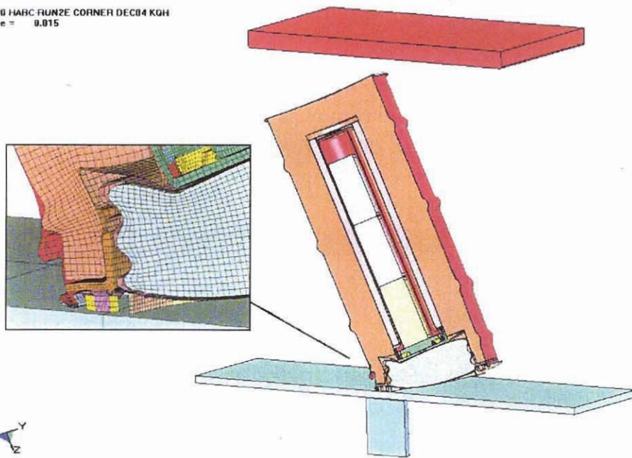
Figure 3.3.1 - HABC-run2e, Configuration of the ES-3100 After the 30-Foot Impact
