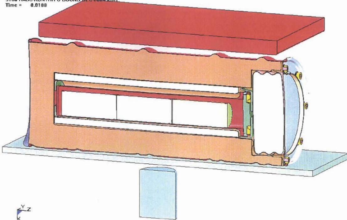
Figure 3.2.4 - HABC-run1hh, Configuration After the 30-Foot Impact
