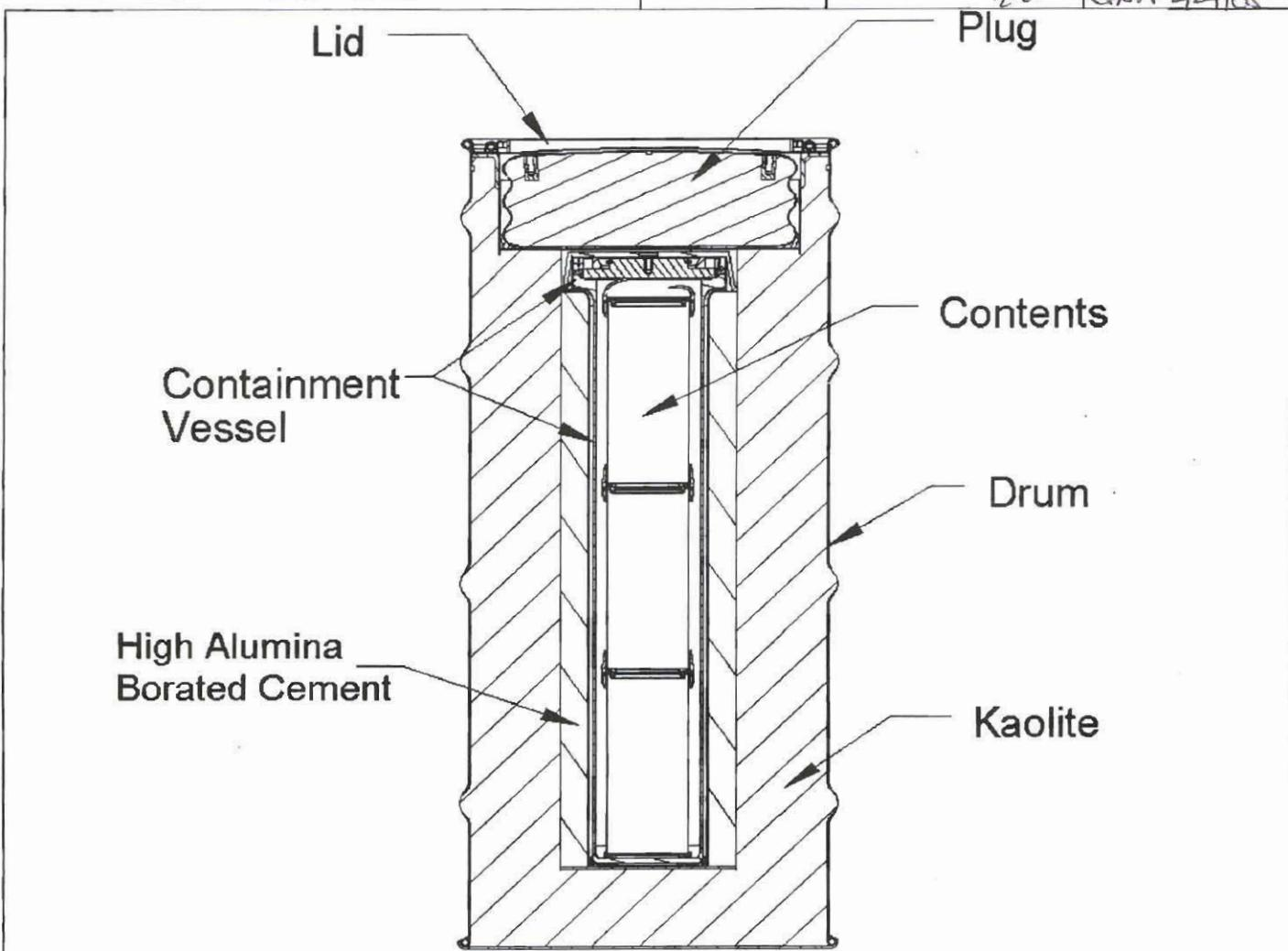
Figure 1.1 - Configuration of the Redesigned ES-3100 with the HABC as the Neutron Absorber
