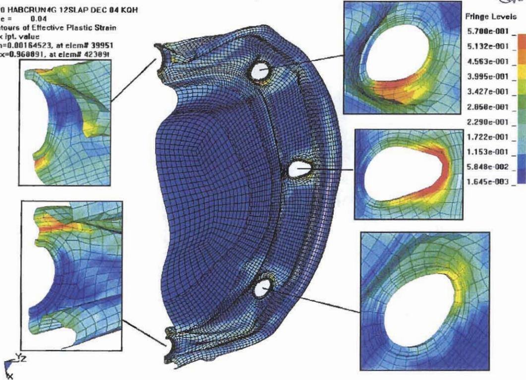
Figure 3.5.12 - HABC-run4g, Crush Impact, Effective Plastic Strain in the Lid
