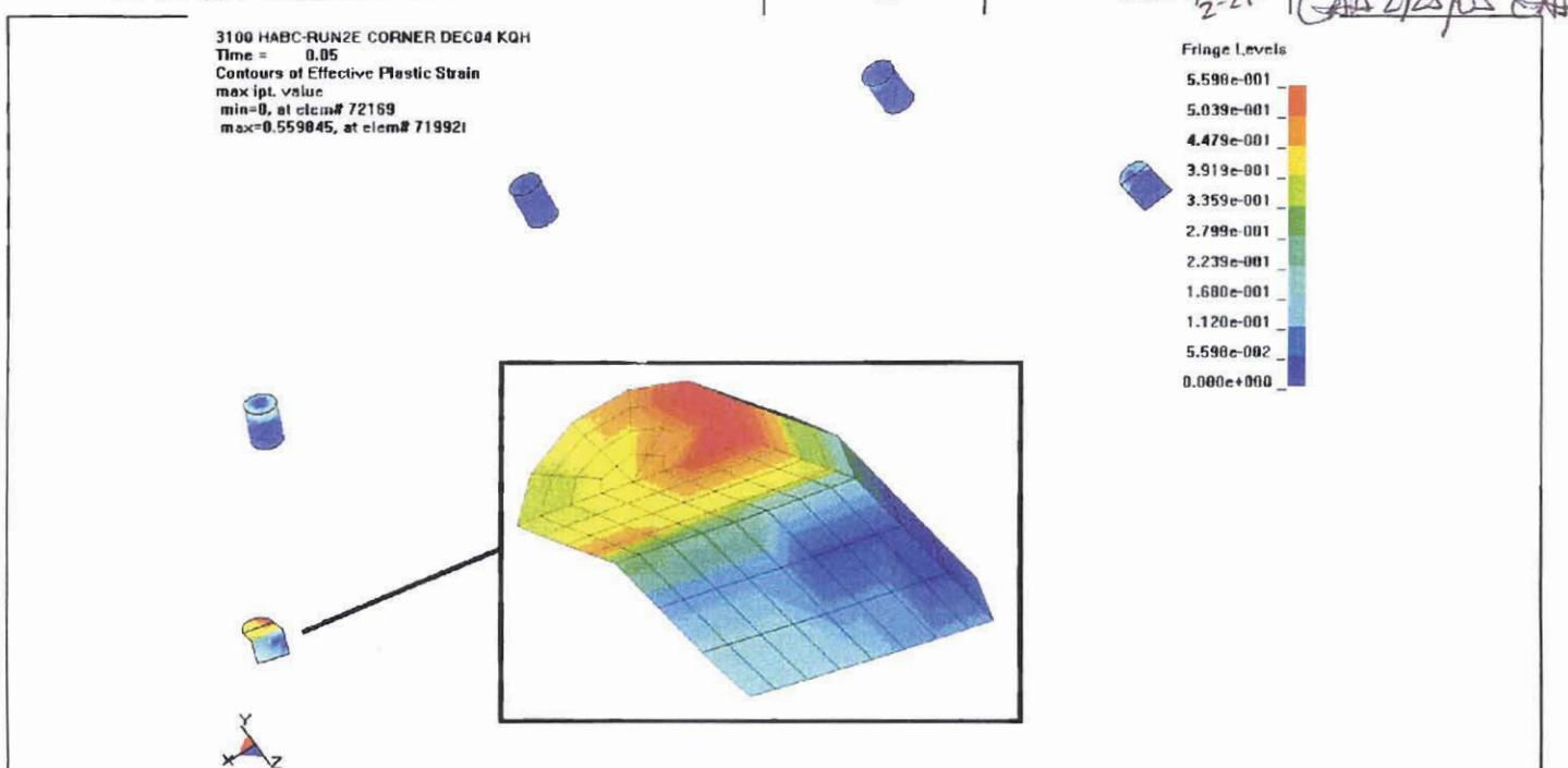
Figure 3.3.8 - HABC-run2e, Crush Impact, Effective Plastic Strain in the Studs
