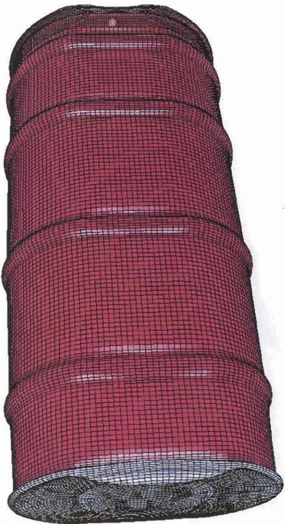
Figure 3.7.4.2 - HABC-run1hh, Cumulative Damage, Rigid Surface Side
