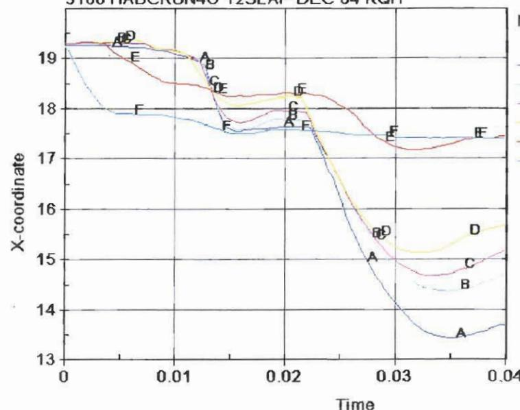
Figure 3.5.16 - HABC-run4g, Diameter Time History for the Drum in the X Direction
