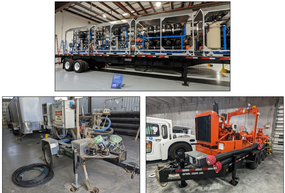
Figure 10: Examples of the Diverse and Flexible Coping Strategies (FLEX) and Strategic Alliance for FLEX Emergency Response (SAFER) Center Equipment
