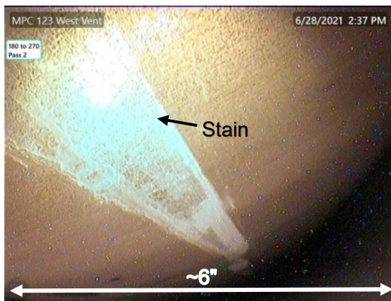
11. Deposit stain on MPC
