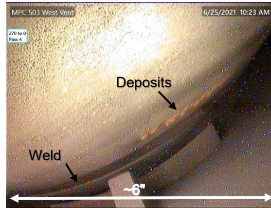
130. Rust colored deposits near lower weld of MPC (continued)
