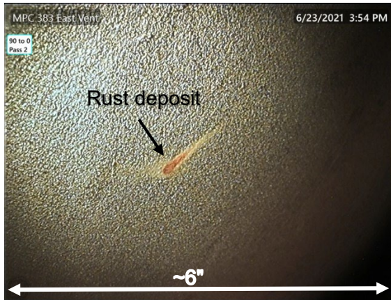
75. Rust deposit on MPC
