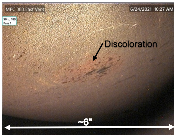
101. Rust colored discoloration on MPC
