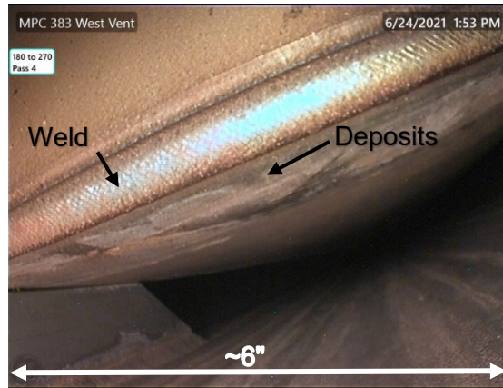
114. Deposits on MPC and overpack and along shim
