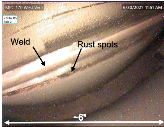
64. Rust spots along lower MPC weld
