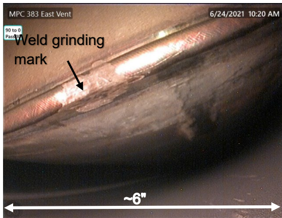
99. Grinding mark on upper weld of MPC
