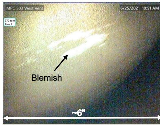
166. Blemish on MPC, no observable depth
