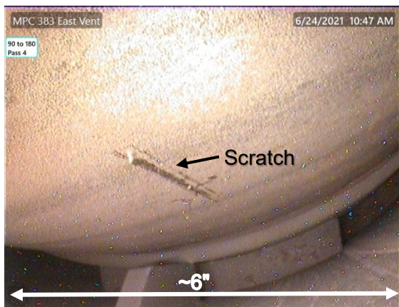
105. Scratch on MPC, no observable depth
