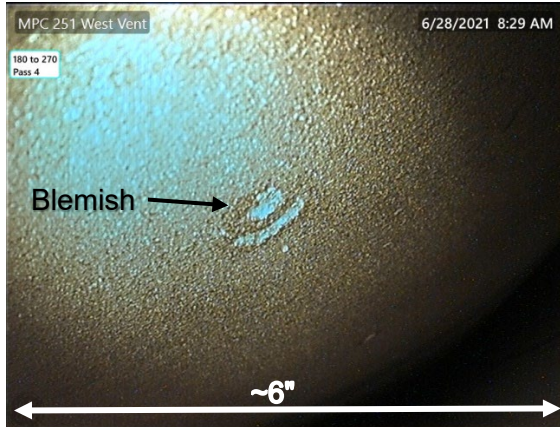
67. Surface blemishes on MPC, possibly scrape marks
