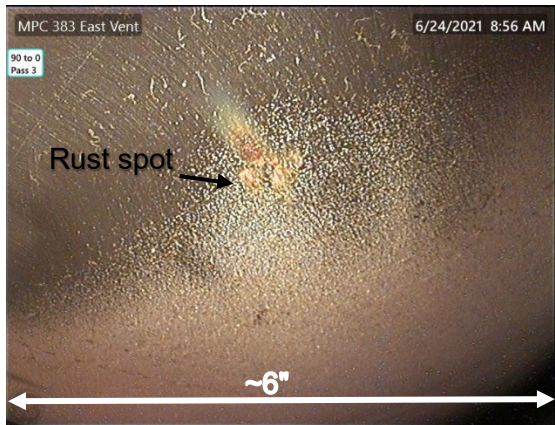
82. Rust spot on MPC, not 3-D
