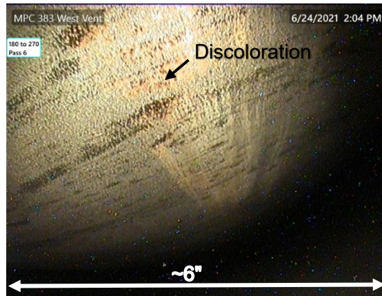
116. Rust colored discoloration on MPC
