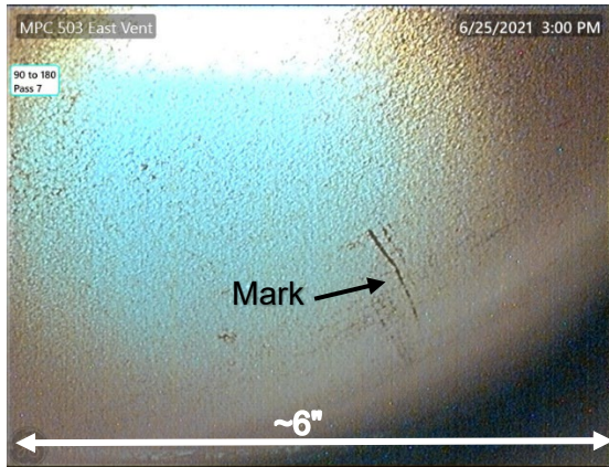
151. Marks on MPC, no observable depth
