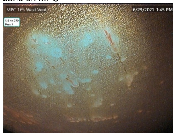
25a. Close up (photo 25) rust spots near middle weld of MPC, not 3-D
