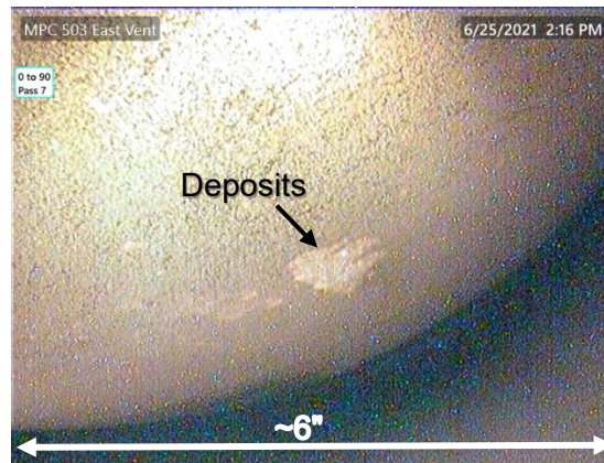
150. Deposit on MPC, no observable depth
