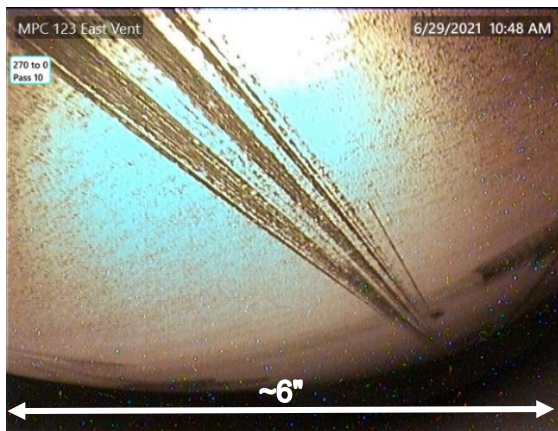
9. Superficial scratches on MPC
