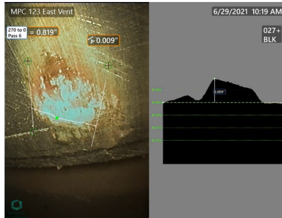
4a. Rust spot (photo 4) measurement, buildup of 0.009" 5
