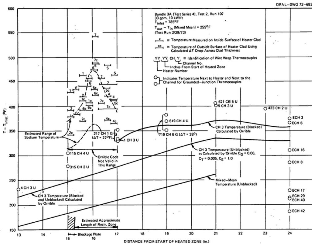
Figure 5-21 Measured Cladding and Coolant Temperature from ORNL 3A Experiments (References [11], [17], and [27]) with 32.8 kW/m and 33 gpm
