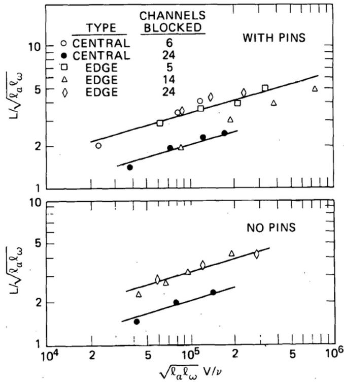
Figure 5-17 Wake Length to Blockage Diameter Ratio versus Blockage Reynolds Number from ORNL (Reference [17], Page 71)
