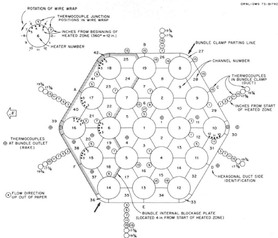
Figure 5-26 Schematic of ORNL THORS 5B 14-Subchannel Edge Blockage [28]
