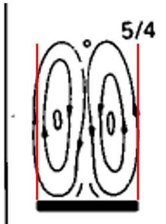
**Figure 5-13: Streamlines from 169 Pin SNR Bundle [17] with Red Lines added to Represent Gap Faces**
