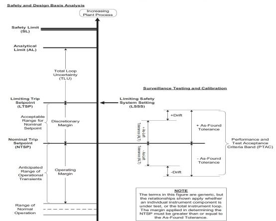
Figure 4-2 Setpoint Relationships during Surveillance Testing and Calibration
