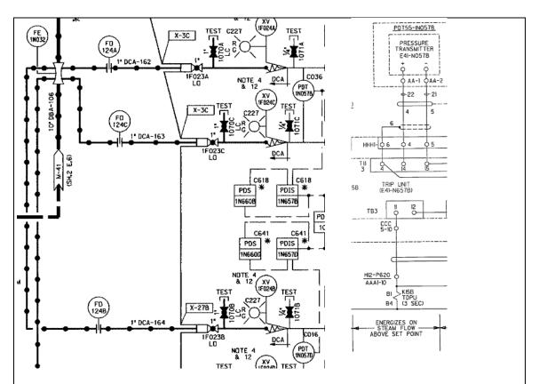
The flow element FE-1N032 is a D/P type flow detector. With no flow in the system, D/P is equal across the detector and sensed at the transmitter. As flow increases, the downstream pressure will drop due to the flow restriction. This d/p is then sensed and converted into a signal which will isolate the HPCI steam lines when the flow rate reaches 300% of normal maximum flow with a 3 sec. time delay to prevent spurious actuation.
