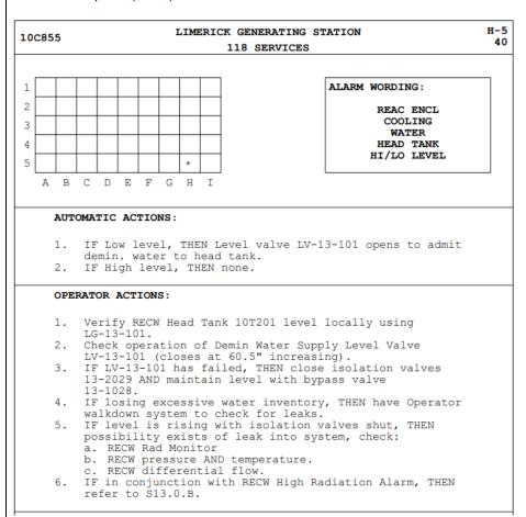
In conjunction with the RECW High Radiation Alarm, the correct conclusion is that water is leaking into RECW from a higher pressure system with contaminated water.
