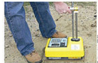
A moisture density gauge indicates whether a foundation is suitable for constructing a building or roadway.
