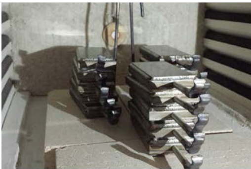
Plates of FM steel were encapsulated in stainless steel encasings, filled with Ar, and aged up to 50kh
