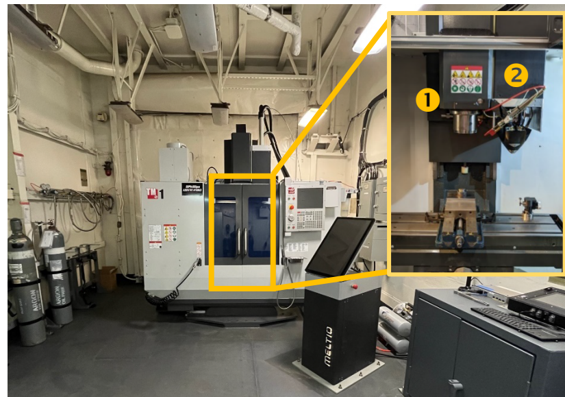
Phillips Additive Hybrid Aboard USS Bataan – November 2022 Laser Metal Wire Deposition System Inset: 1) CNC Tool Spindle, 2) Deposition Head
