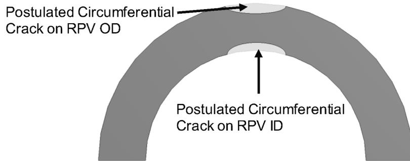
**Figure 3-9 Representation of Postulated Semi-Elliptical Axial Cracks in Reactor Pressure Vessel Wall**
