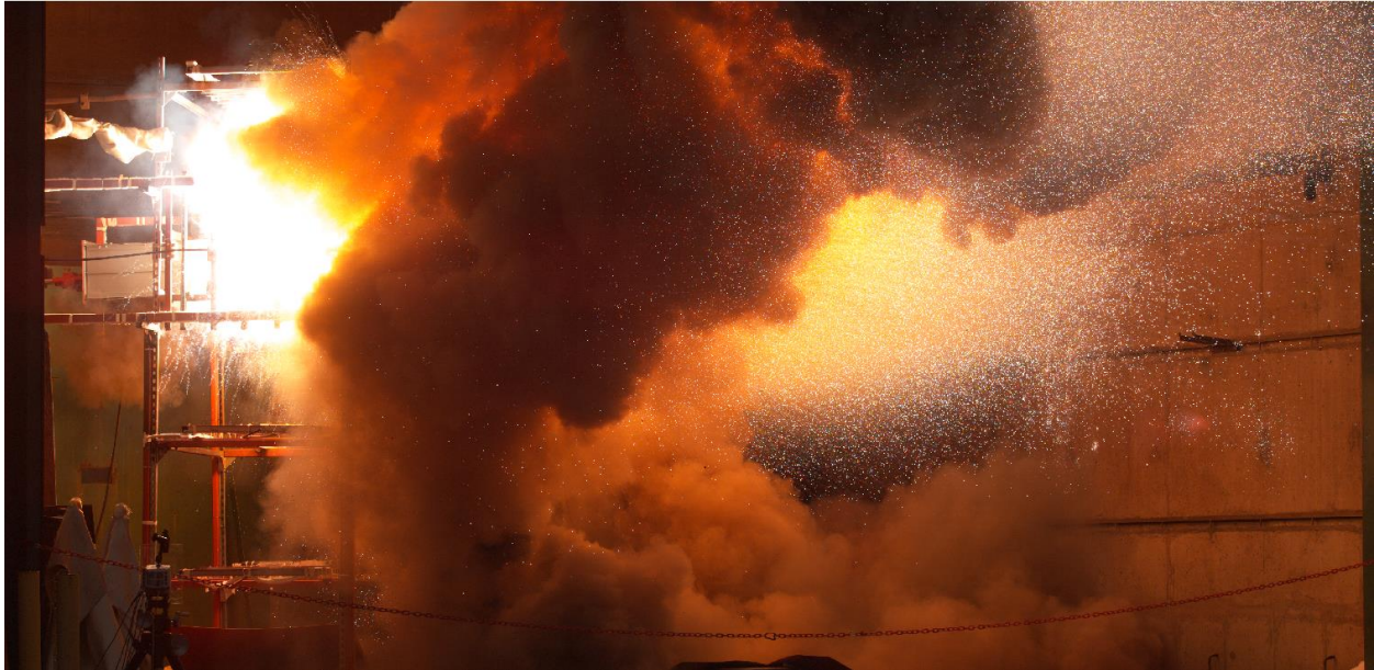
Figure 3-11: Test 2-27 imaged through 4k camera – camera imaging at 1000 fps. Notice the orange/red color flame and dust, and the bright white particulate 0.93 seconds from trigger.
