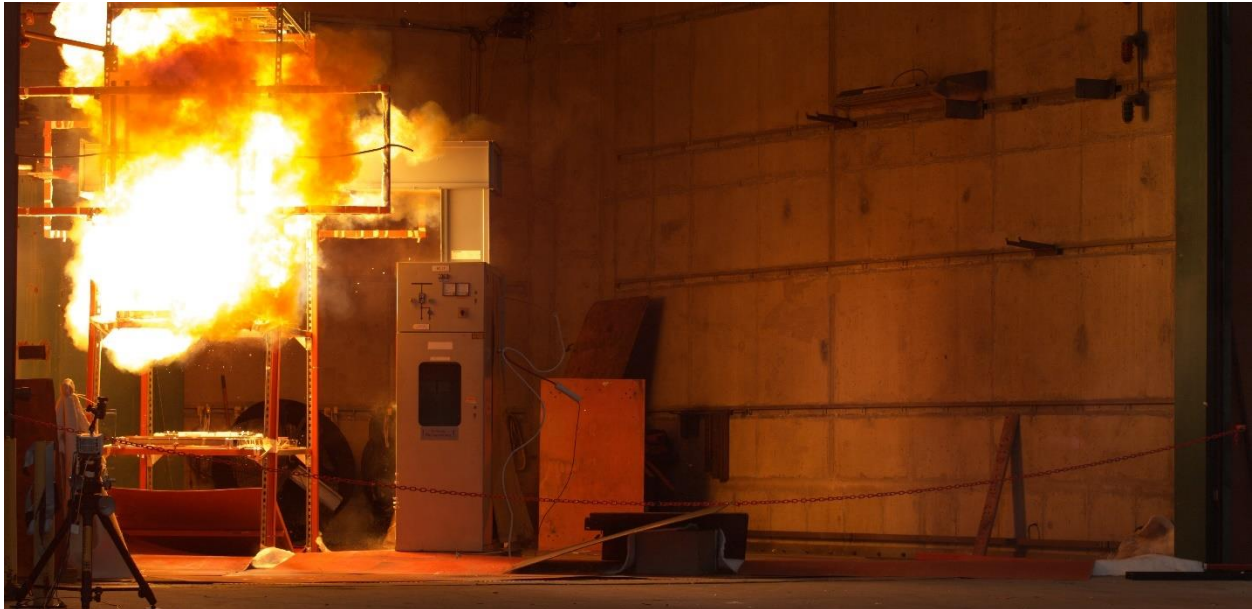
Figure 3-2: Test 2-25 imaged through 4k camera – camera imaging at 1000 fps. Notice the orange/red color in the background 0.19 seconds from trigger.
