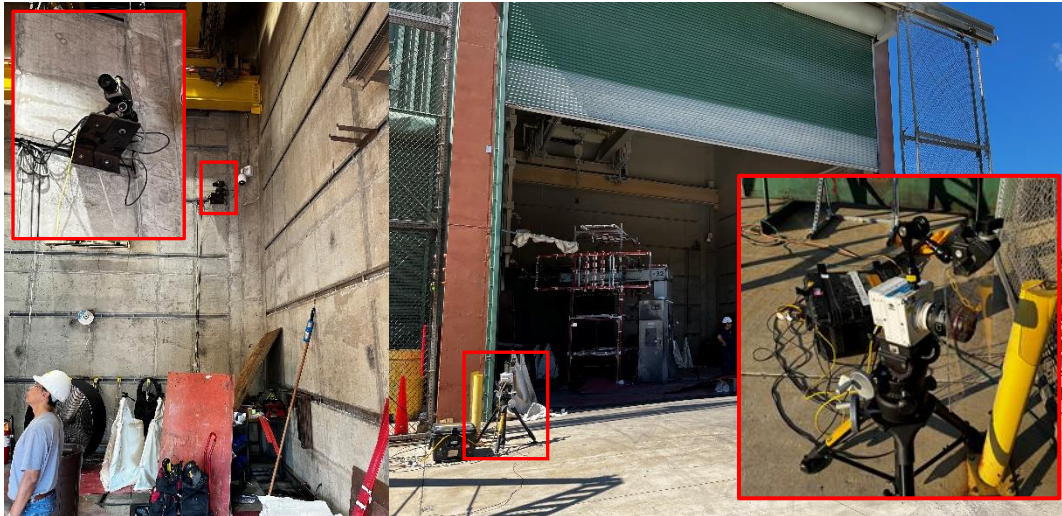
Figure 1-4: Phantom v7 HS camera (left panel) perched at the top of the northeast side of TC9; 1310 VEO (right panel) near the ground and southeast, just outside TC9. Both cameras were looking in these locations at the bus ducts. The insets show close up of the cameras.
