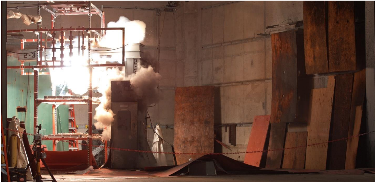
Figure 3-21: Test 2-31 imaged through 4k camera – camera imaging at 1000 fps. Notice the luminosity of the white cloud of Alumina illuminated by the arc and the burning aluminum 0.09 seconds from trigger.
