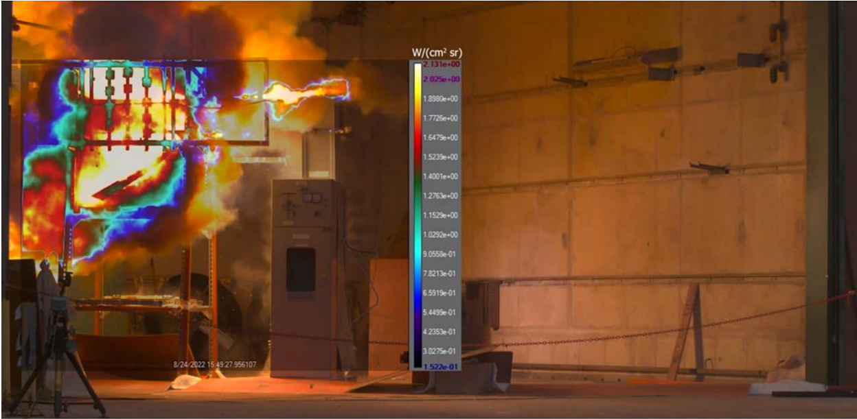
Figure 3-4: Image fusion of IR camera (in radiance units of W/cm^2\ sr ) synchronized with a visible image 0.37 seconds from trigger.
