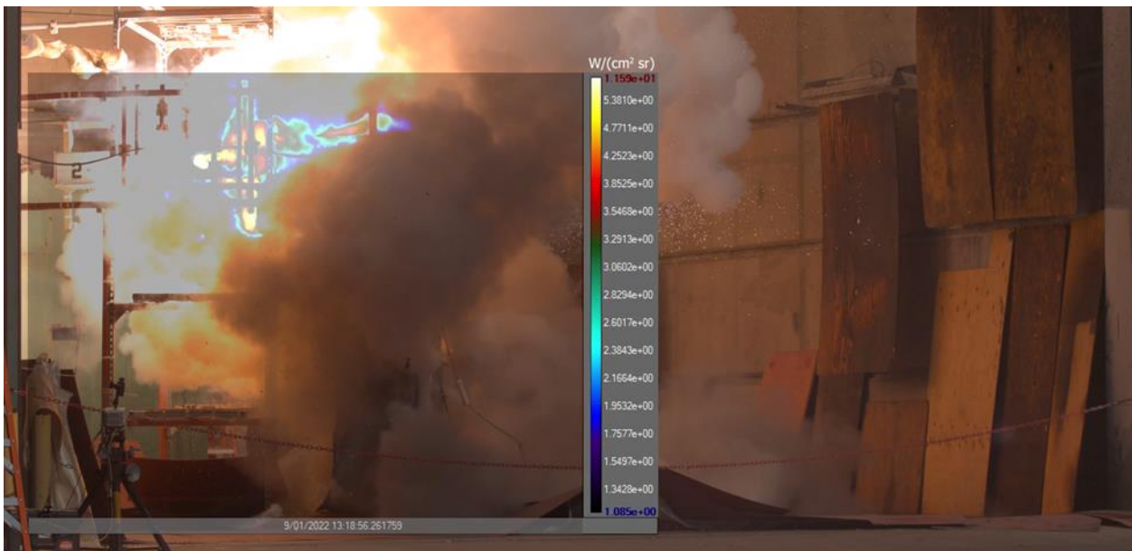
Figure 3-23: Image fusion of IR camera (in radiance units of W/cm^2\ sr ) synchronized with a visible image 0.64 seconds from trigger.
