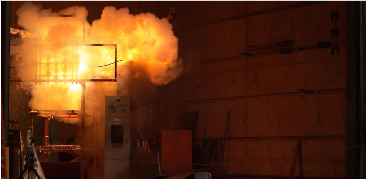
Figure 3-8: Test 2-30 imaged through 4k camera – camera imaging at 1000 fps. Notice the orange/red color in the background 0.24 seconds from trigger. The first 100 milliseconds seems to show a white cloud.
