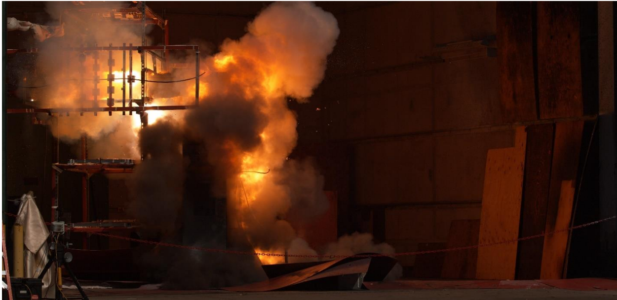
Figure 3-18: Test 2-30B imaged through 4k camera – camera imaging at 1000 fps. Notice the orange/red color in the background 0.180 seconds from trigger. The first 130 milliseconds seems to show a white burning cloud.
