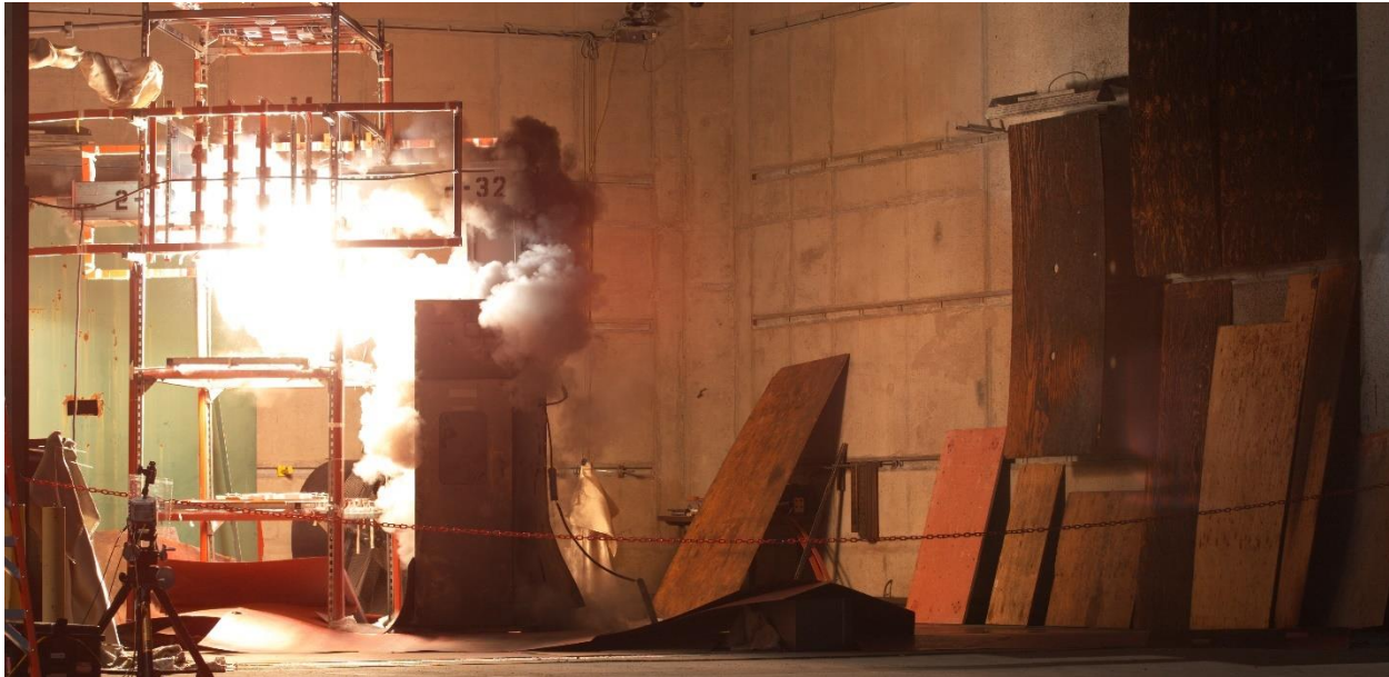
Figure 3-24: Test 2-32 imaged through 4k camera – camera imaging at 1000 fps. Notice the luminosity of the white cloud of Alumina (similar to 2-31) illuminated by the arc and the burning aluminum 0.08 seconds from trigger.
