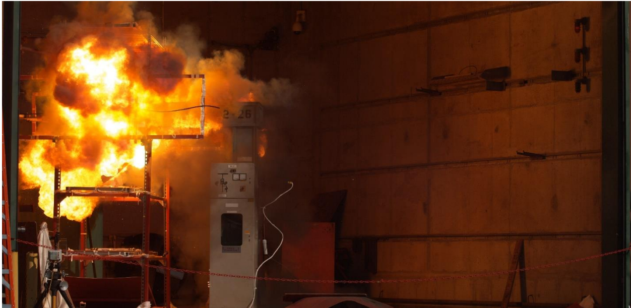
Figure 3-5: Test 2-26 imaged through 4k camera – camera imaging at 1000 fps. Notice the orange/red color in the background 0.25 seconds from trigger.
