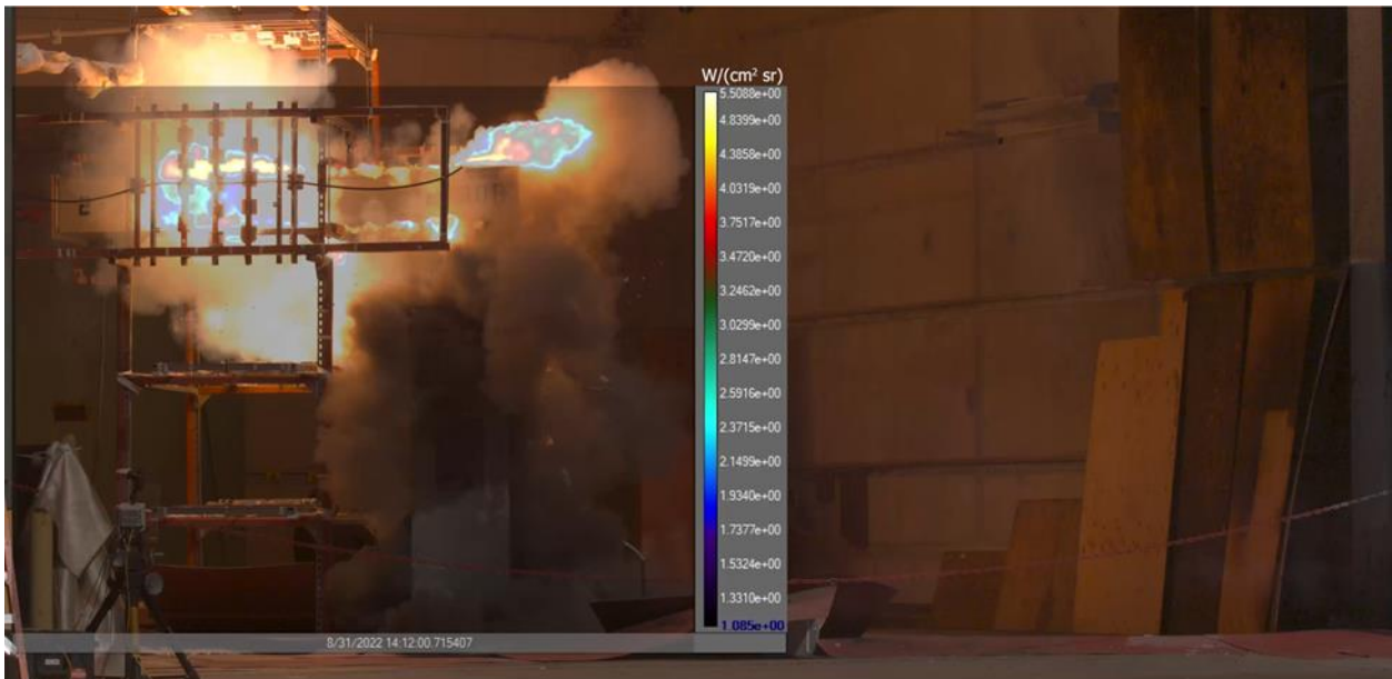
Figure 3-20: Image fusion of IR camera (in radiance units of W/cm^2 \text{ sr} ) synchronized with a visible image 0.12 seconds from trigger.
