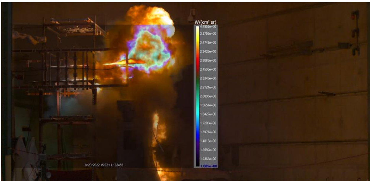
Figure 3-13: Image fusion of IR camera (in radiance units of W/cm 2 sr) synchronized with a visible image 0.2 seconds from trigger.
