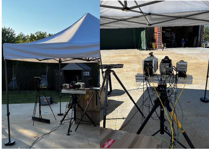
Figure 1-3: Front (left panel) and back view (right panel) of the HS remote cameras collecting during the bus duct tests.
