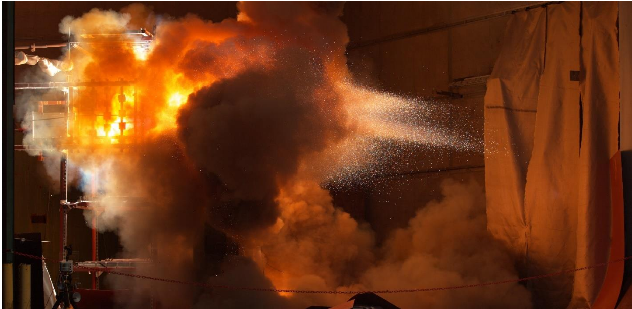
Figure 3-14: Test 2-28 imaged through 4k camera – camera imaging at 1000 fps Notice the orange/red color flame and dust, and the bright white particulate ejected towards the east 0.65 seconds from trigger.
