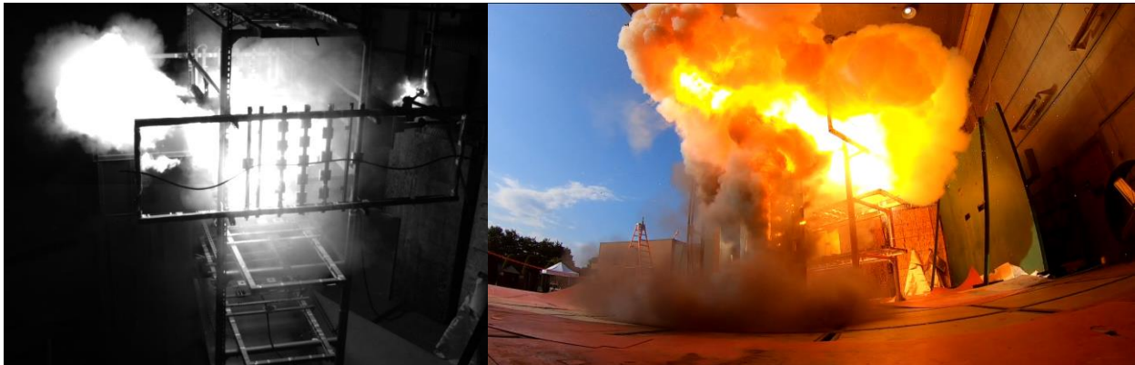
Figure 3-9: From left to right: Phantom v7, 4,000 fps, at top northeast side – notice the arcing at the right side of the image at the juncture between the test and the facility (0.15 seconds from trigger); GoPro inside floor at northeast.
