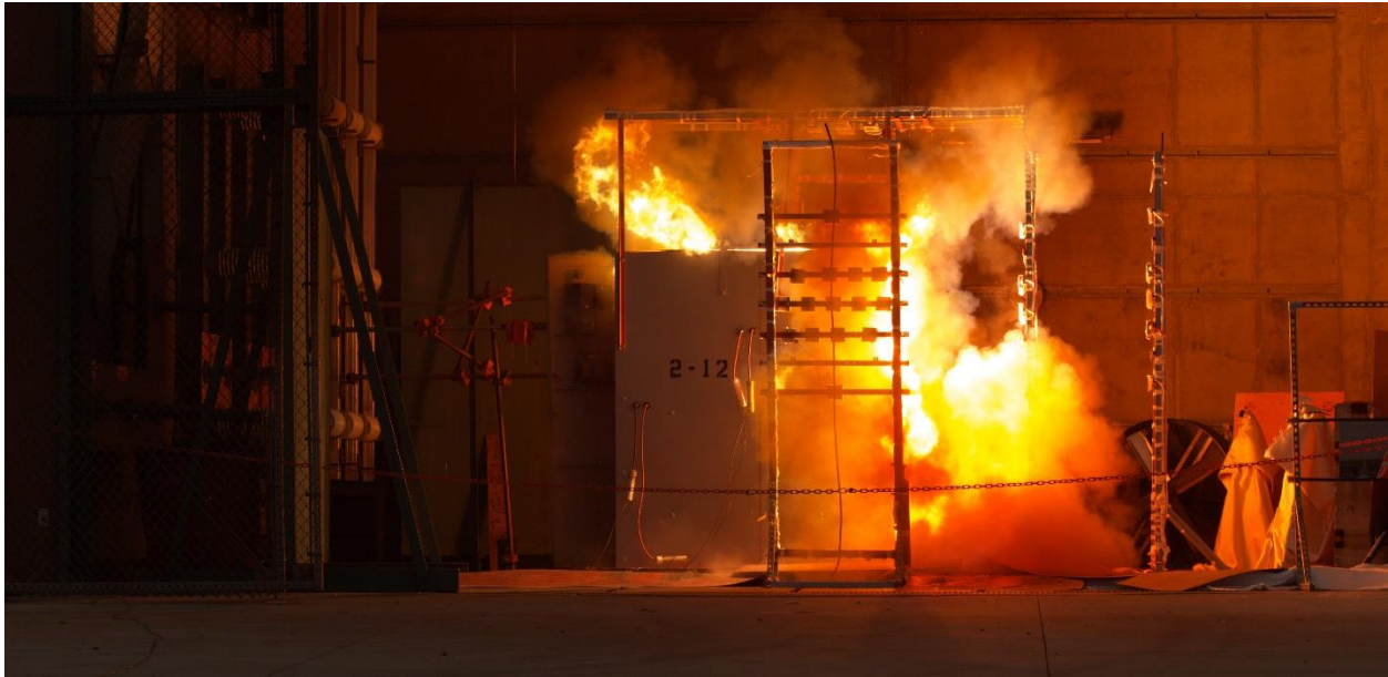
Figure 2-5: Test 2-12 imaged through 4k camera –camera imaging at 1000 fps. Notice the orange/red color in the background 0.17 seconds from trigger.
