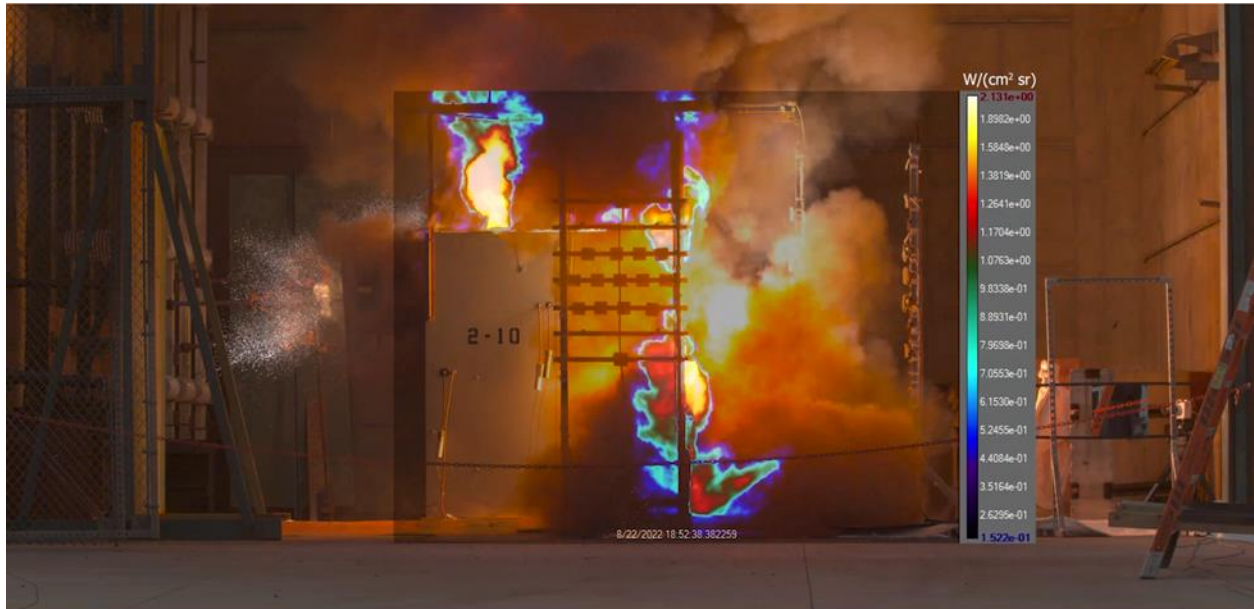
Figure 2-4: Image fusion of IR camera (in radiance units of W/cm^2 \text{ sr} ) synchronized with a visible image 0.52 seconds from trigger.
