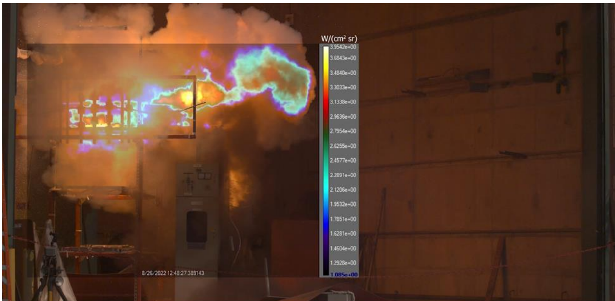
Figure 3-10: Image fusion of IR camera (in radiance units of W/cm^2\ sr ) synchronized with a visible image 0.3 seconds from trigger.
