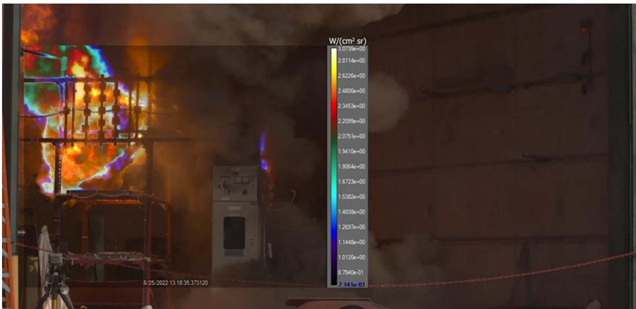
Figure 3-7: Image fusion of IR camera (in radiance units of W/cm^2 sr ) synchronized with a visible image 1.68 seconds from trigger.
