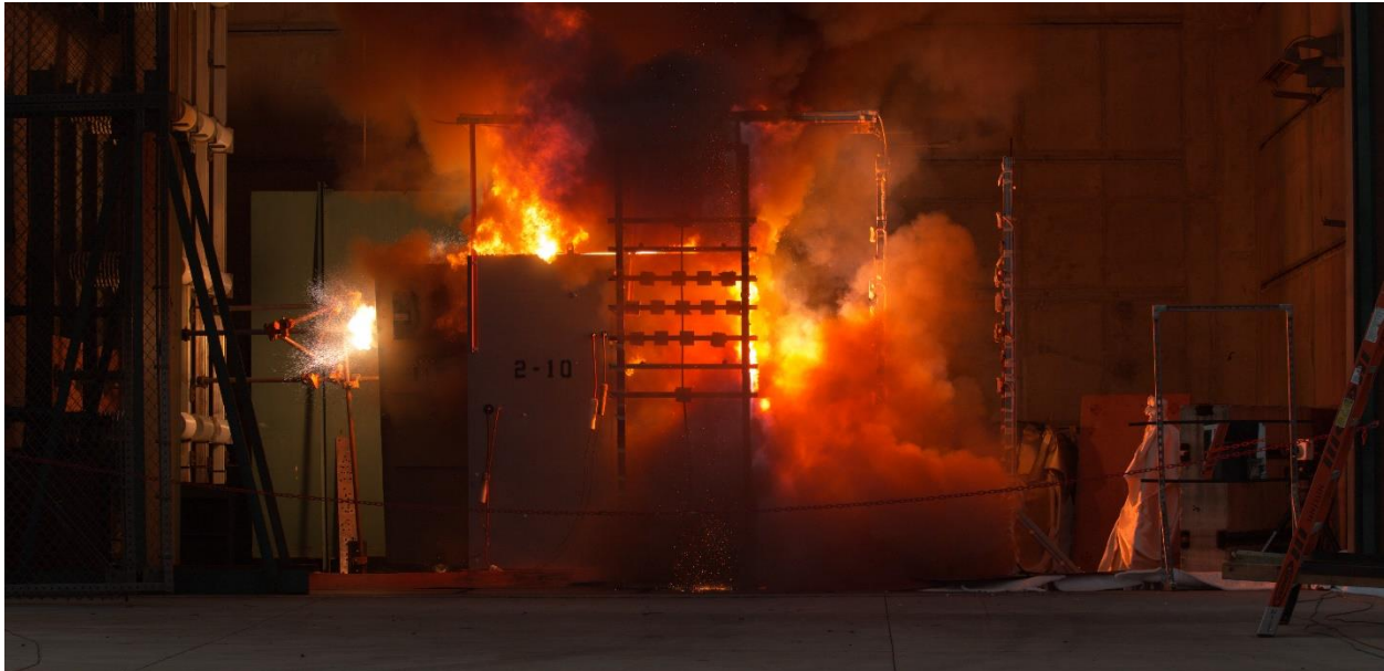
Figure 2-2: Test 2-10 imaged through 4k VEO camera – camera imaging at 1,000 fps. Notice the yellow orange/red color in the background 0.5 seconds from trigger.
