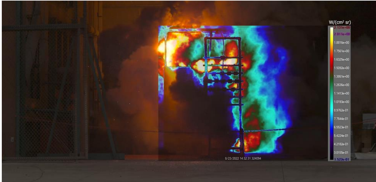
Figure 2-7: Image fusion of IR camera (in radiance units of W/cm^2 sr ) synchronized with a visible image 2.53 seconds from trigger.
