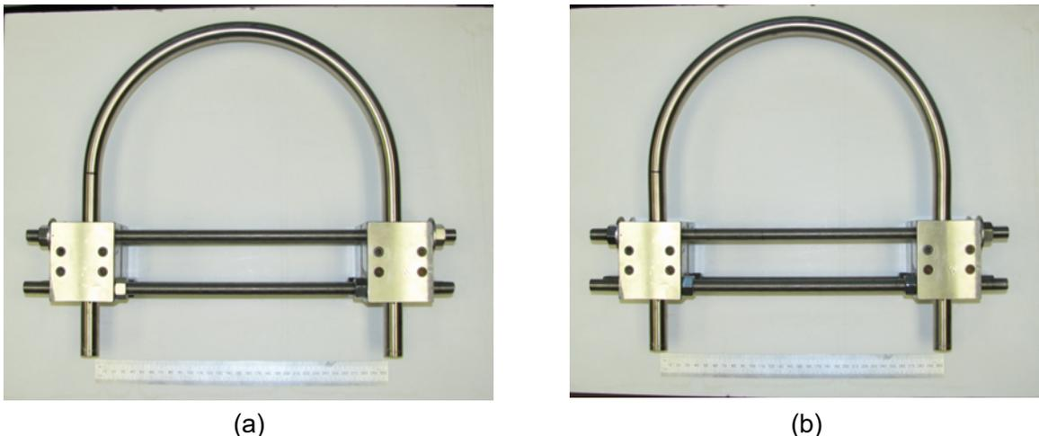
**Figure 2-13. 152-mm bend radius U-bend with clamps (a) before and (b) after the inward leg displacement. Note that the ruler in the photos is 300 mm long.**
