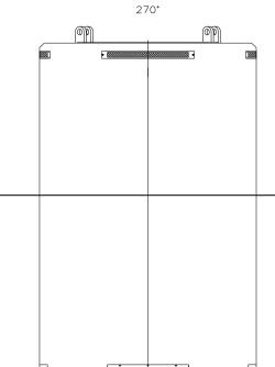
TSC mid-plane – approximately 92 inches from bottom. Measure dose rates at four target points (approximately 0, 90, 180 & 270 degrees) on the mid-plane.
