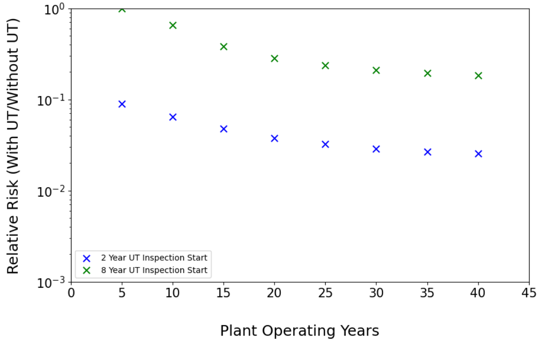
Figure 1 Relative risk of SB LOCA in long flaw case with UT inspections normalized against long flaw case without UT inspections when UT inspections start at 2 years and 8 years.
