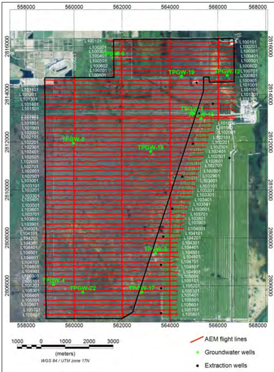
Figure 4.2-1. 2022 AEM Survey Area, Flight Lines, Monitoring Well Locations and Designation of Compliance Area Boundary (Black Line)
