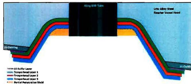
Figure 7 – Final Weld Configuration.
