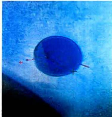
**Figure 1 – Two indications identified at the surface of the Reactor Vessel Level Indication System vent line.**
