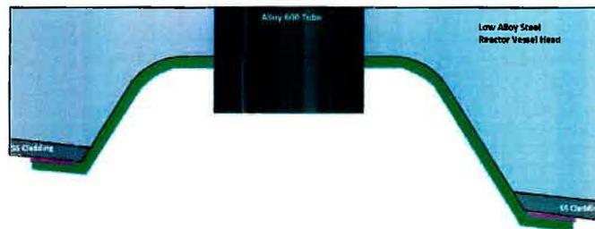
**Figure 5 – First Layer Temper Bead**
