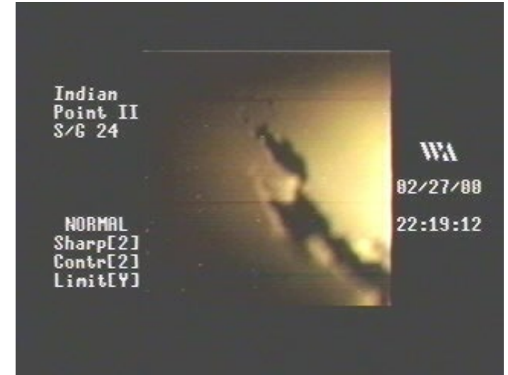
Indian Point SG tube leak (February 2000)
