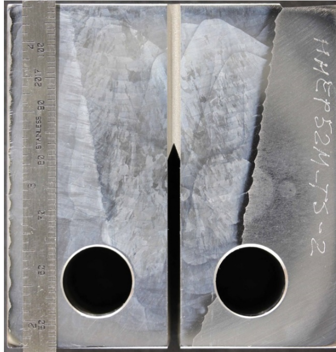
Figure 90 Specimen HHEP52M-TS-2 machined from the high heat input Alloy 52M weld produced by EPRI.
