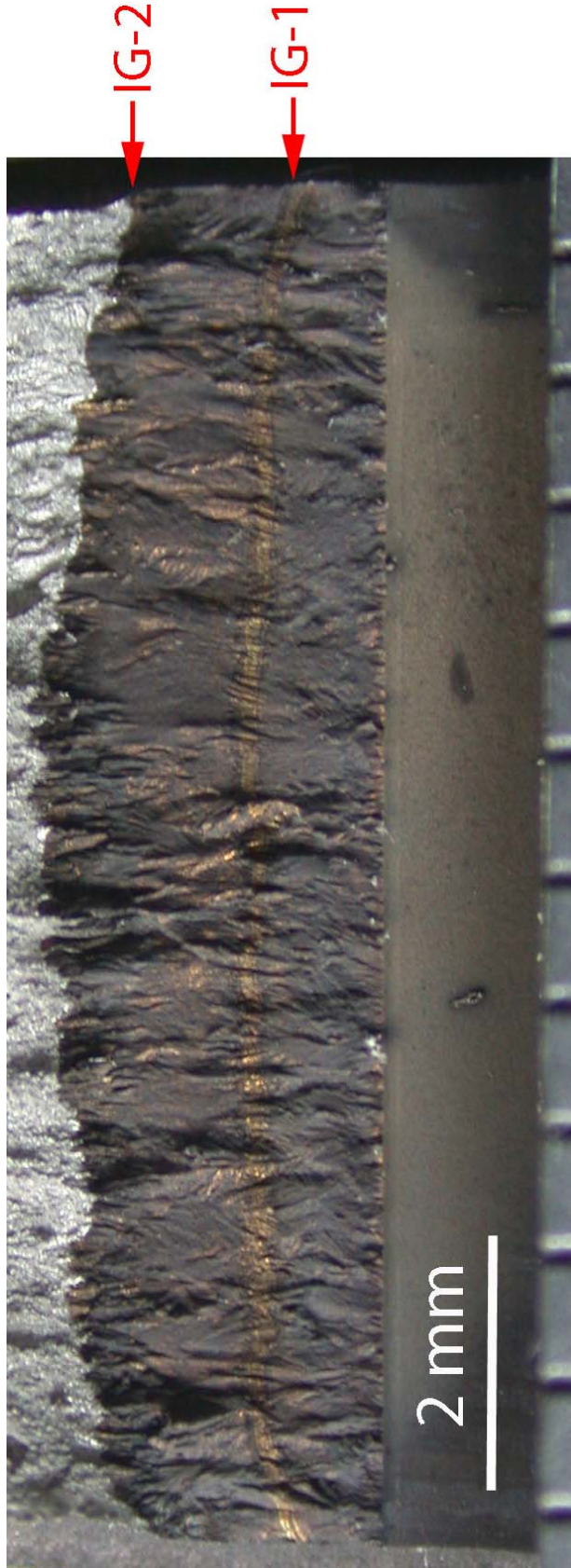
Figure 81 Fracture surface of specimen NC152-CR-1. Crack advance is from bottom to top.
