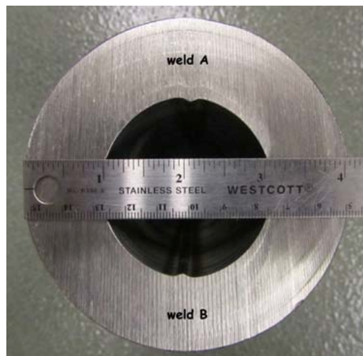
Figure 10 Alloy 52 welds produced by MHI on a piece of CRDM tubing.
