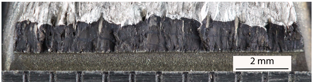
Figure 111 Fracture surface of Alloy 52 specimen MC52-20CF-CR-1 tested in simulated PWR environment. Crack advance is from bottom to top.
