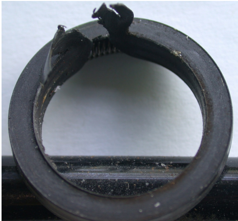
Figure 107 The ruptured of the pullrod seal appears consistent with a “jolt”.
