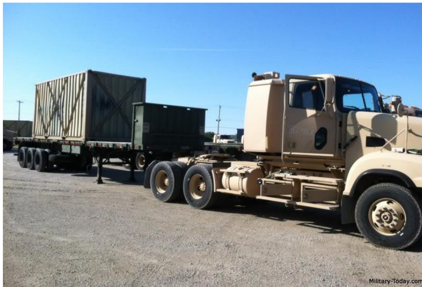
Figure 1-2. An Army M915A5 Tractor with a M872A4 Semi-Trailer Carrying a 20 ft ISO Container 3
