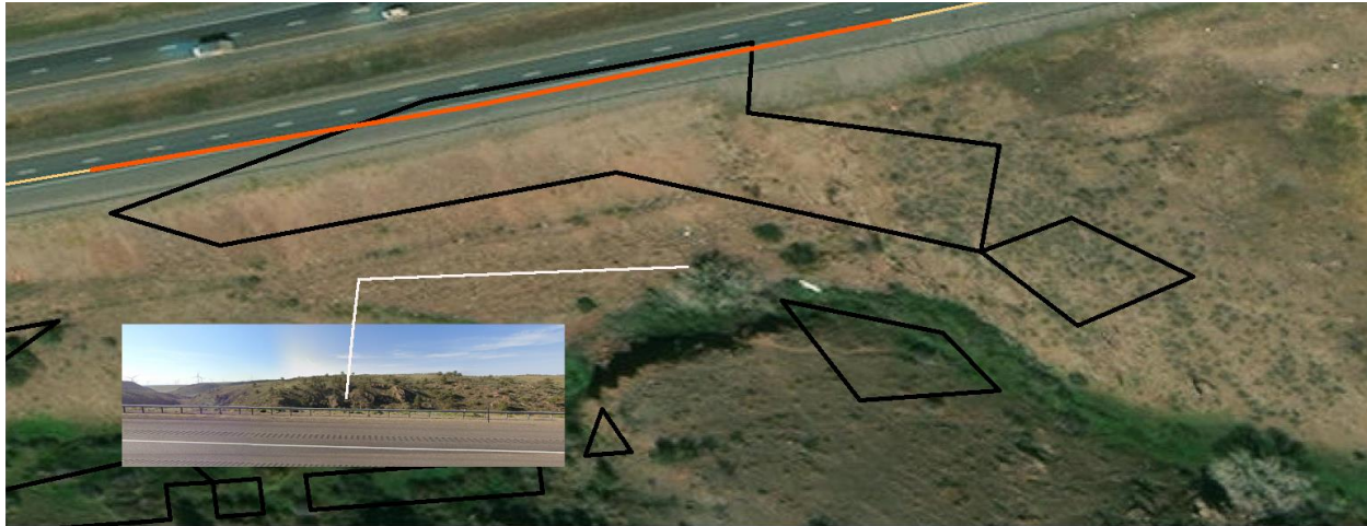
Figure 4-18. Large Ditch where the Slope appears both Down and Away as well as Down and Toward the Route
