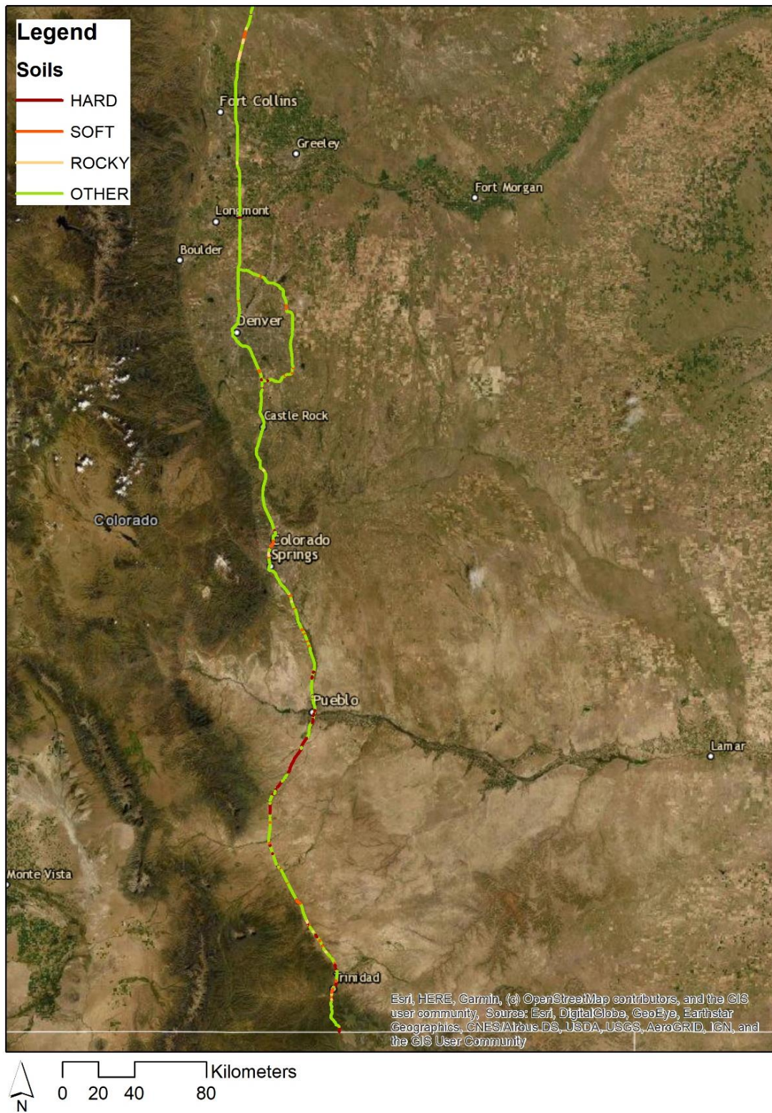
Figure 4-6. Potential Route from INL to WSMR with Wayside Geology Classification: Colorado
