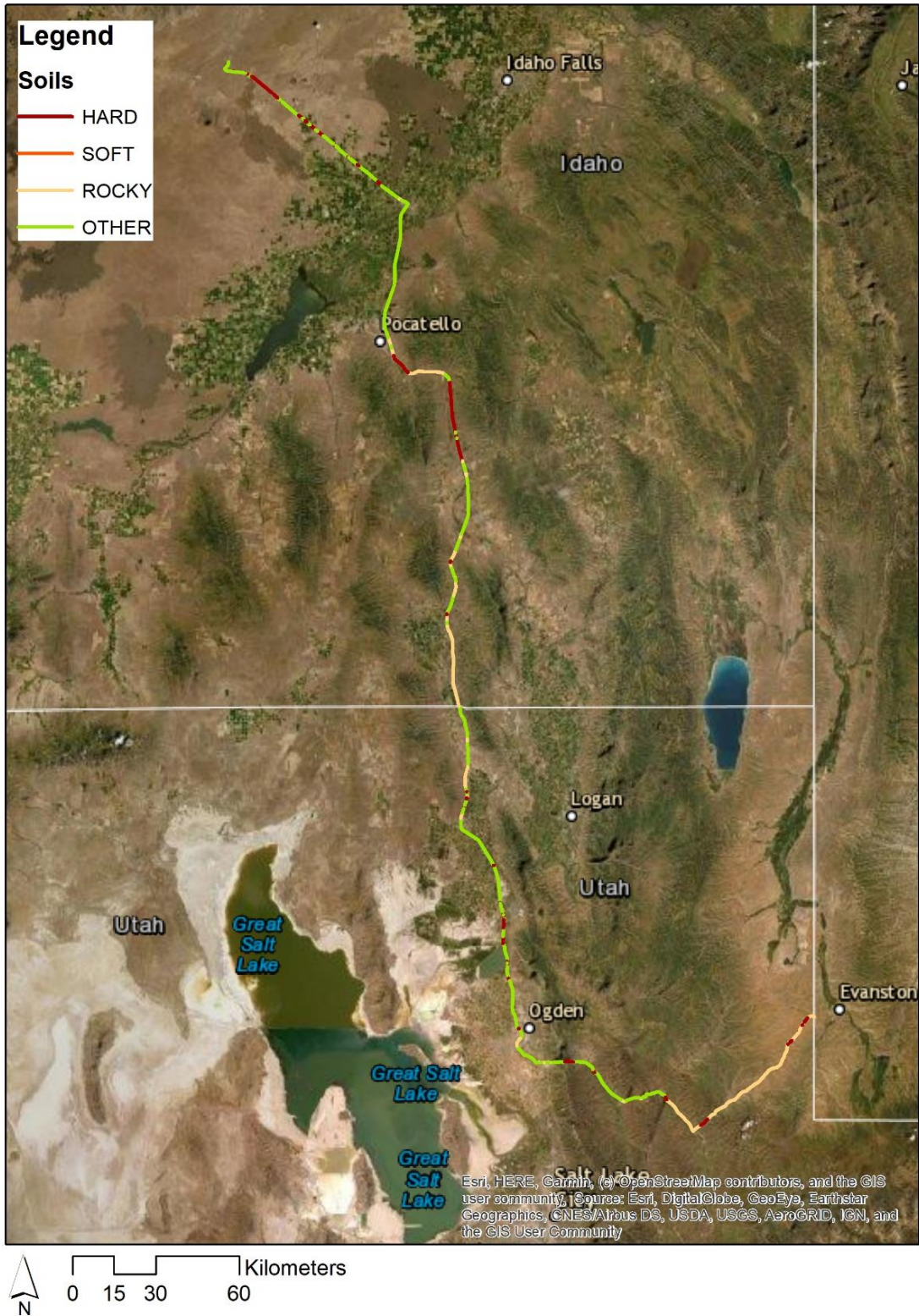
Figure 4-4. Potential Route from INL to WSMR with Wayside Geology Classification: Idaho and Utah
