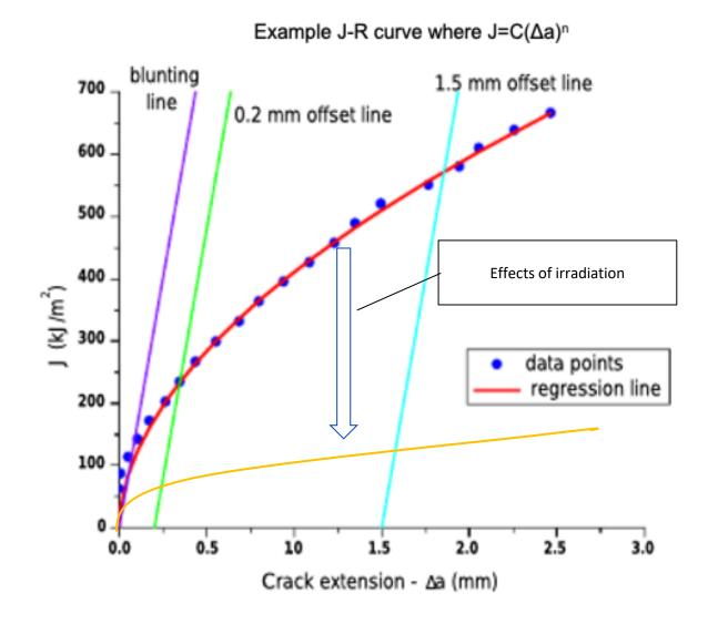
Effects of irradiation will typically result in lower toughness and hence lower J-∆a curves but this can also be the result of the material that is being tested (weld vs base metal)
