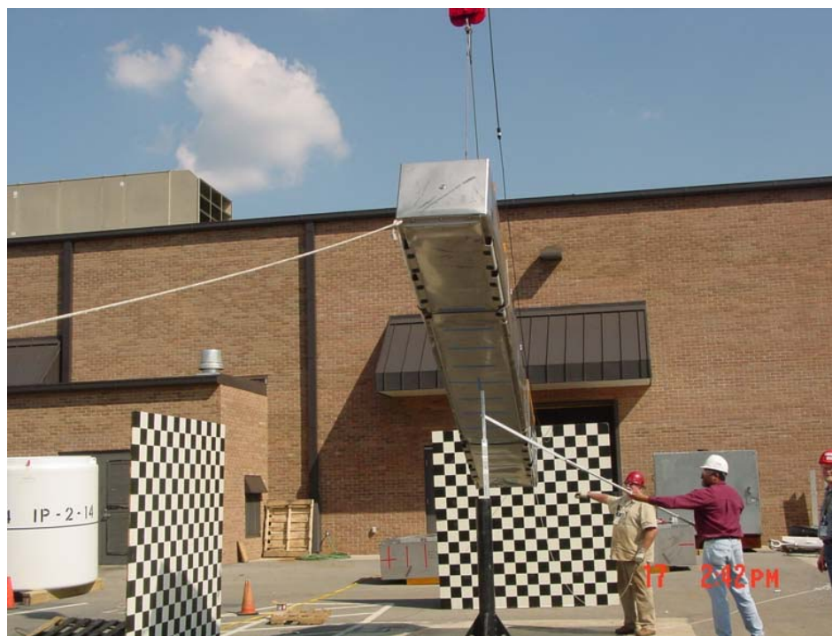
Figure 2-26 Alignment for Oblique Puncture
