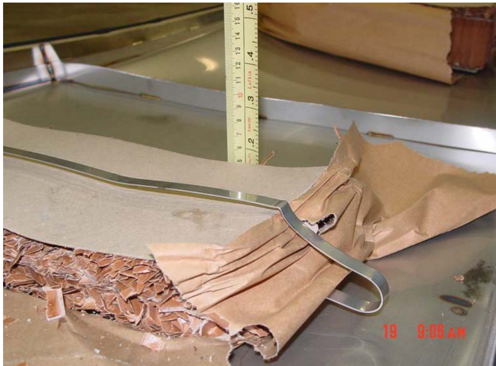
Figure 2-38 Lid Crush on CTU 1
