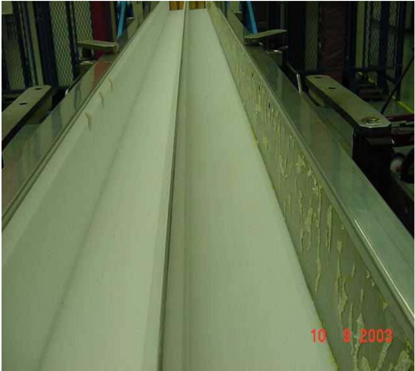
Figure 2-16 Inner Container Being Prepared to Receive Mockup Fuel and Added Weight
