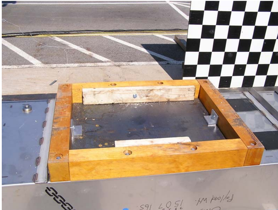
Figure 2-23 Addition of Tare Weight to CTU 1
