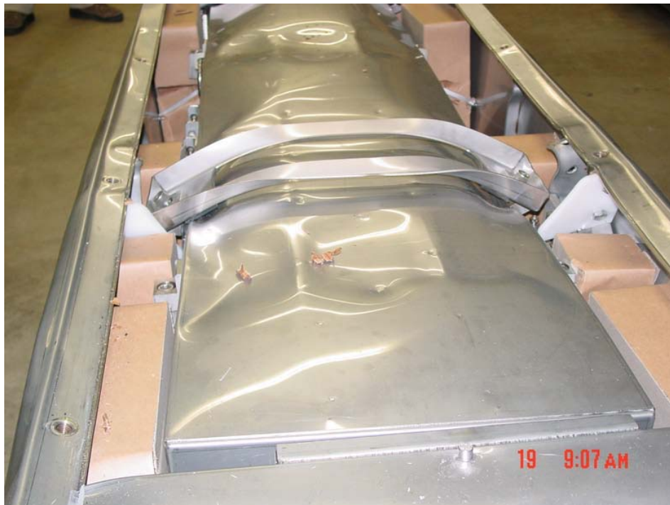
Figure 2-36 Damage Inside Outer Container to CTU 1
