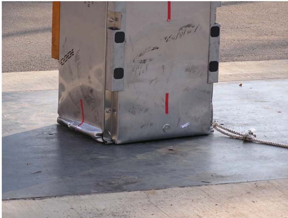
Figure 2-35 End Impact Damage (Top and Side)
