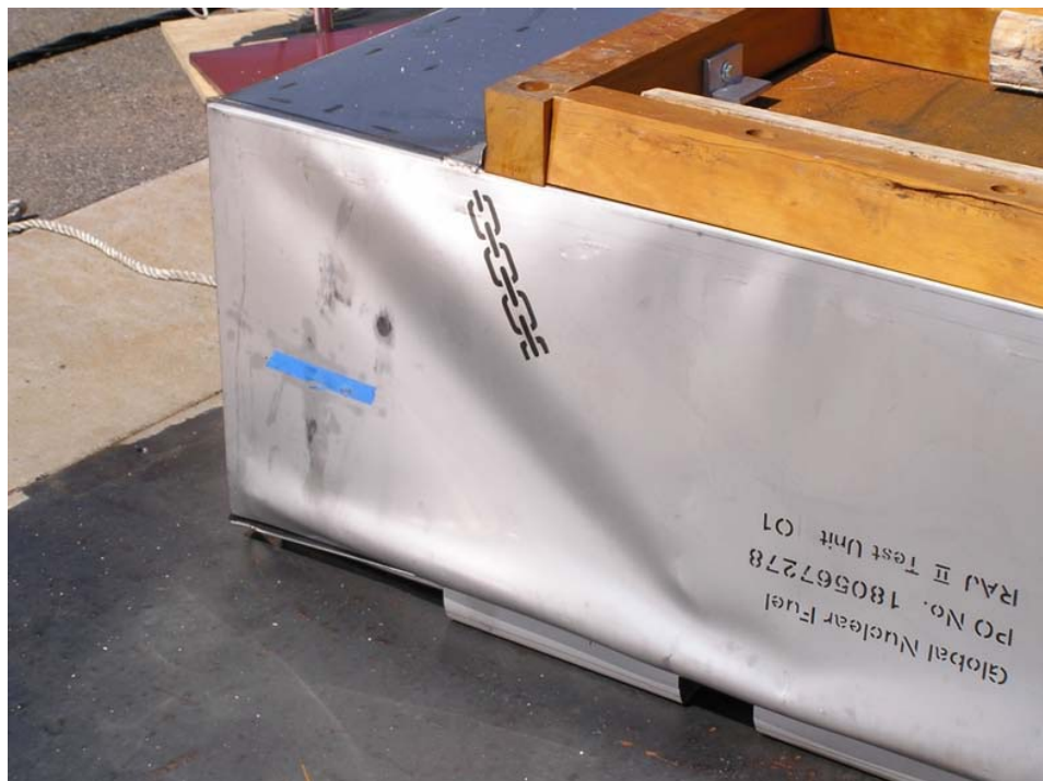
Figure 2-30 Secondary Impact End Damage
