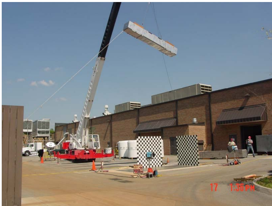
Figure 2-25 CTU 1 Positioned for 15° 9-m (30-foot) Slap-down Drop
