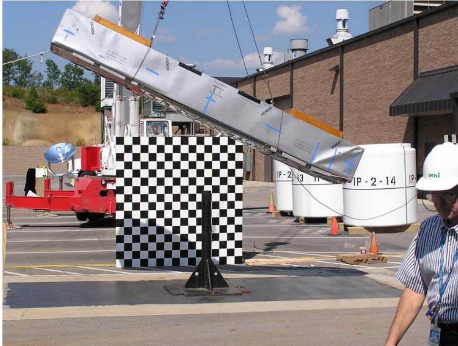
Figure 2-27 Position for Puncture Test
