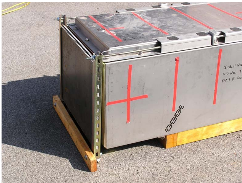
Figure 2-24 Addition of Tare Weight to CTU 2
