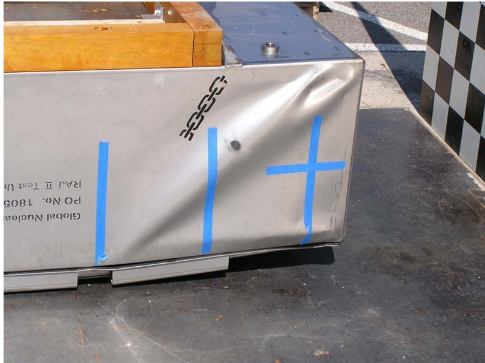
Figure 2-29 Primary Impact End Slap-down Damage
