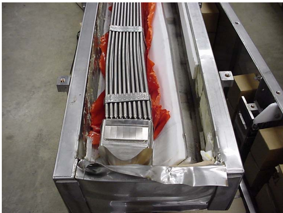
Figure 2-40 Internal Damage to CTU 2
