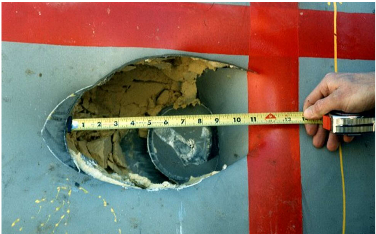
Figure 2.10.3-41 – CTU-1 Puncture Drop No. 7; Post-Drop Damage
