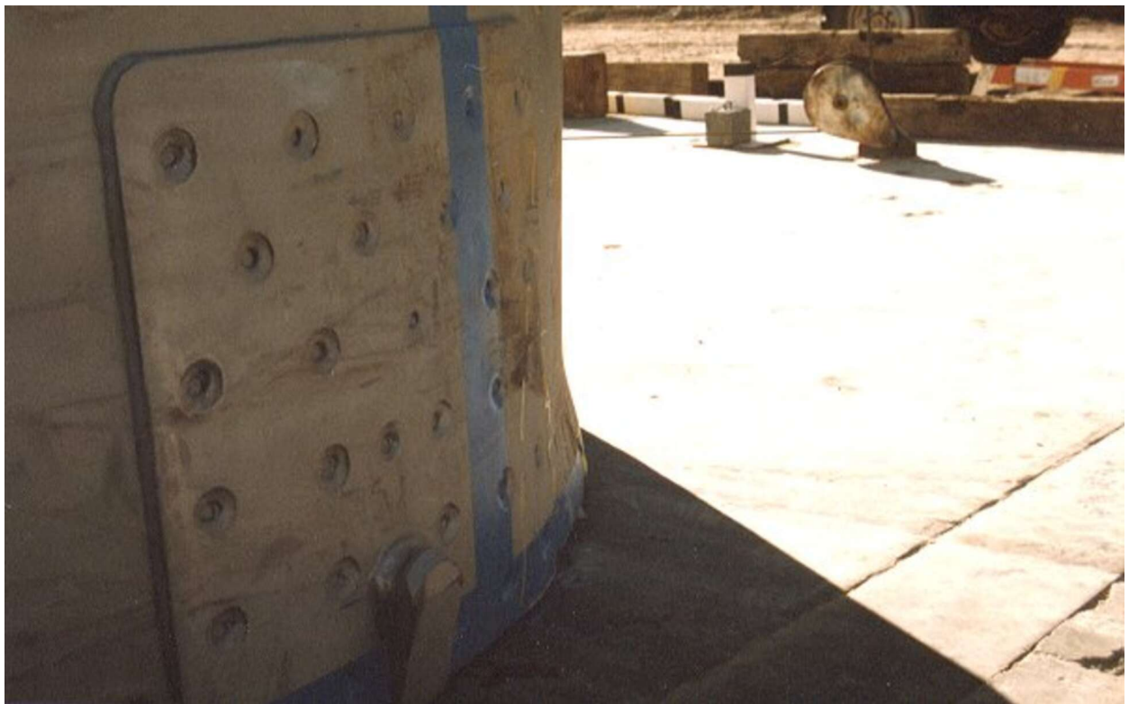
Figure 2.10.3-59 – CTU-2 Free Drop No. 2; Post-Drop Damage
