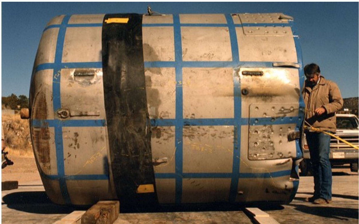
Figure 2.10.3-61 – CTU-2 Free Drop No. 3; Post-Drop Damage
