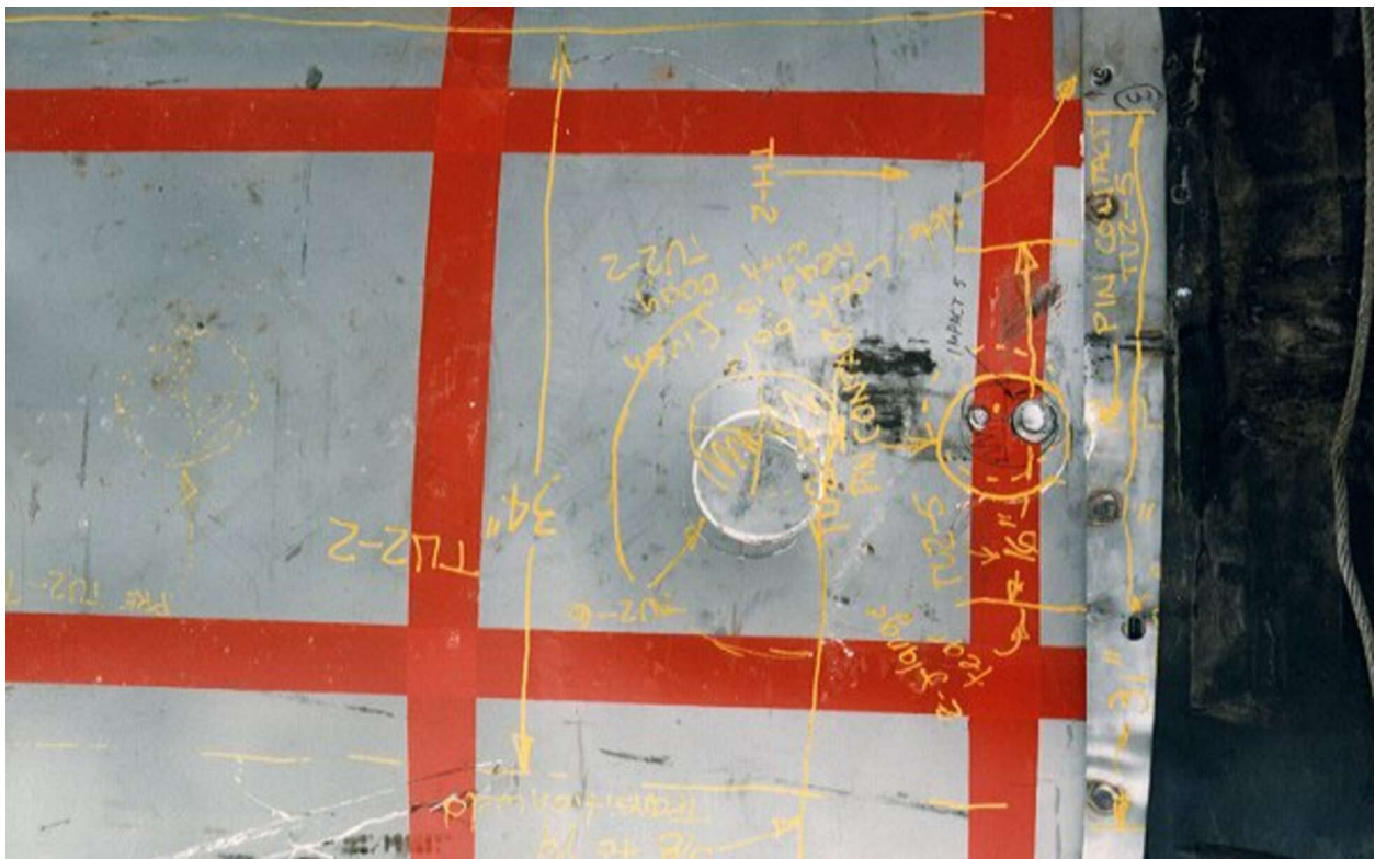
Figure 2.10.3-39 – CTU-1 Puncture Drop No. 6; Post-Drop Damage
