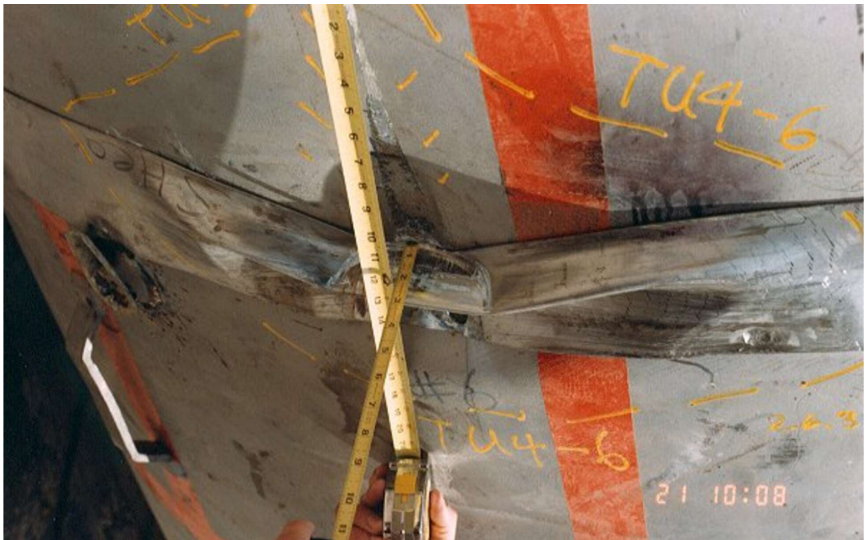
Figure 2.10.3-91 – CTU-3 Puncture Drop 6; Post-Drop Damage
