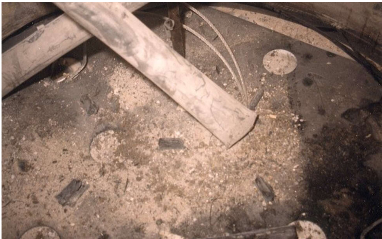
Figure 2.10.3-53 – CTU-1 Disassembly; Loose Debris on Pallet in ICV Body
