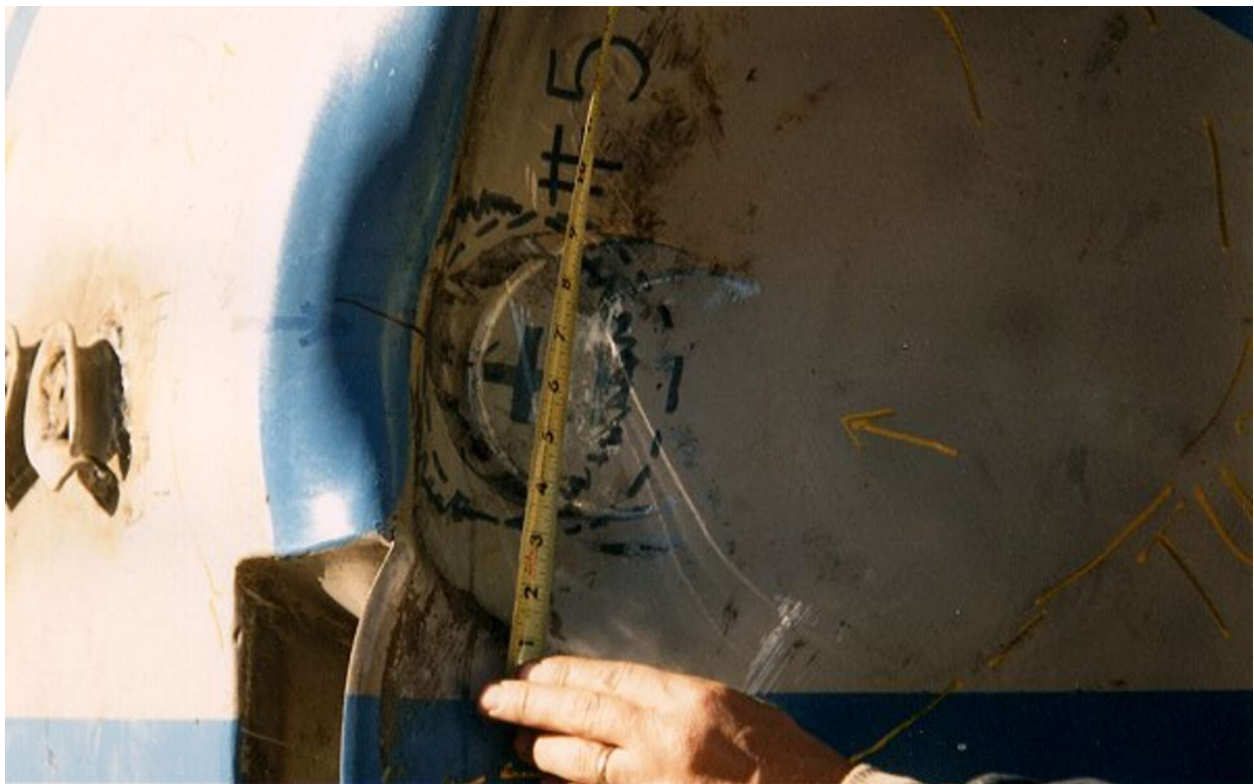
Figure 2.10.3-67 – CTU-2 Puncture Drop 5; Post-Drop Damage
