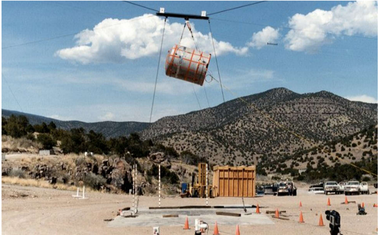
Figure 2.10.3-84 – CTU-3 Free Drop No. 3; Pre-Drop Positioning
