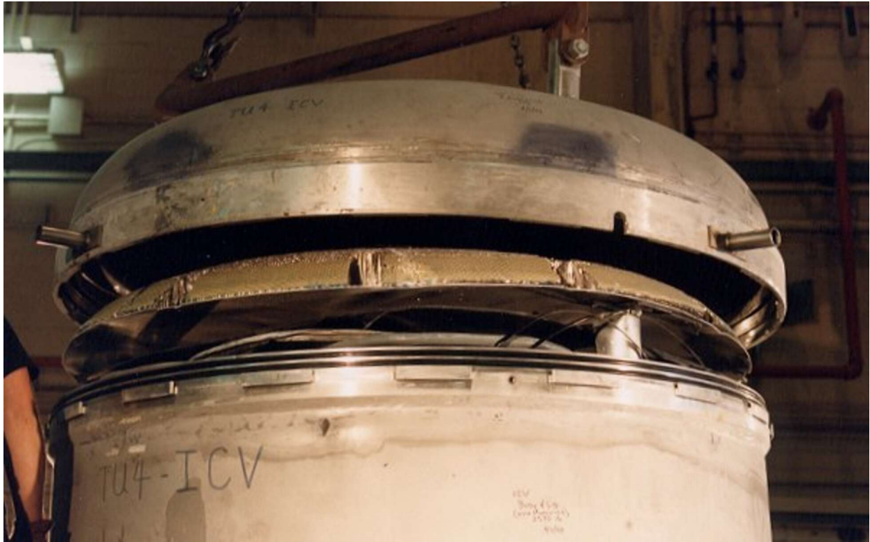
Figure 2.10.3-98 – CTU-3 Disassembly; ICV Lid Removal
