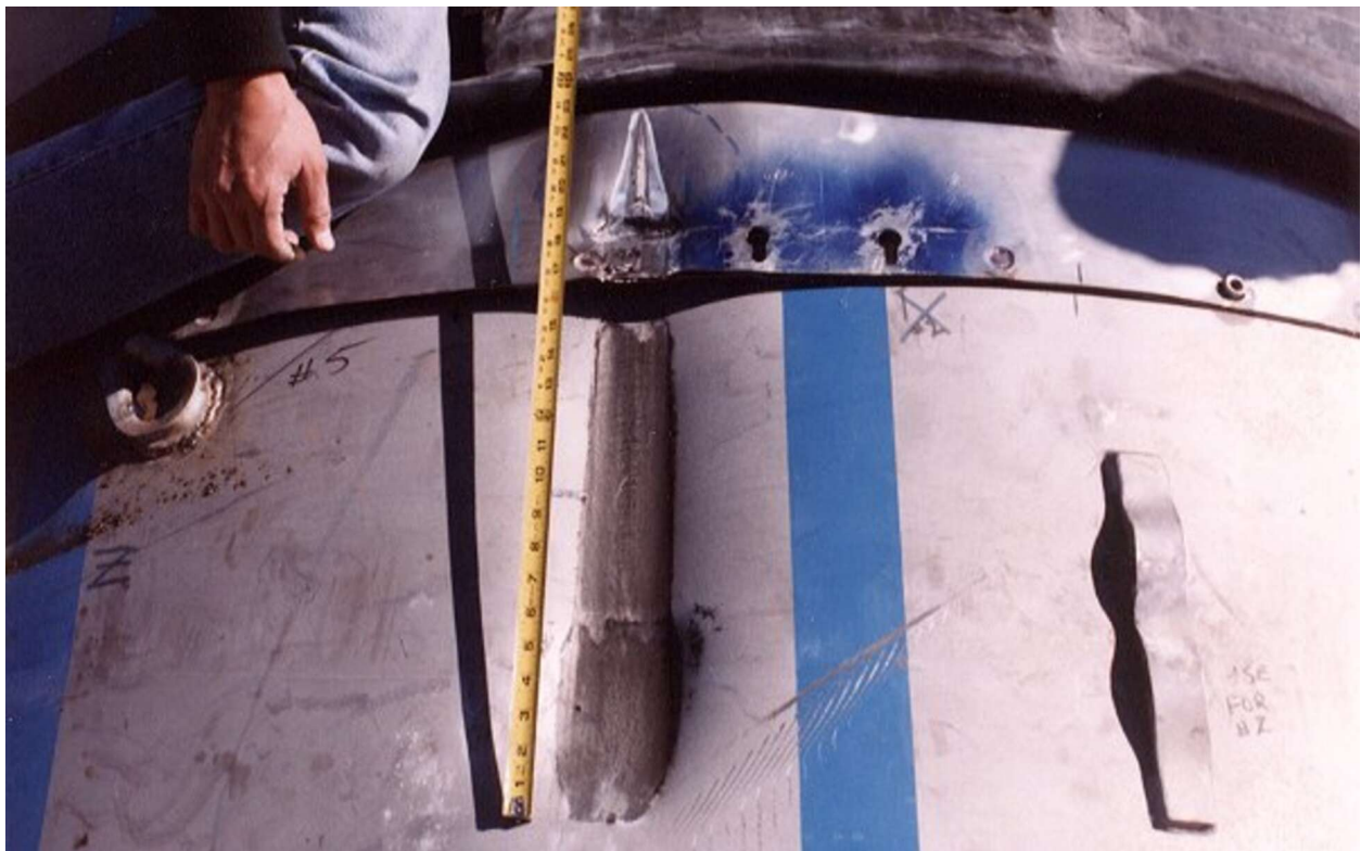
Figure 2.10.3-69 – CTU-2 Puncture Drop 6; Post-Drop Damage
