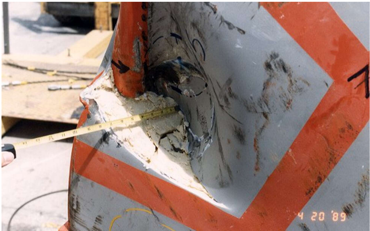
Figure 2.10.3-89 – CTU-3 Puncture Drop 5; Post-Drop Damage
