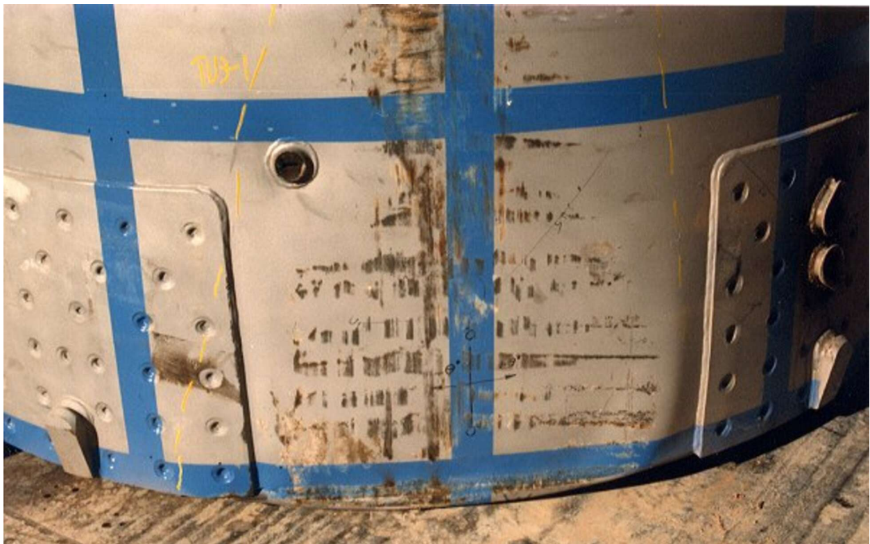
Figure 2.10.3-57 – CTU-2 Free Drop No. 1; Post-Drop Damage
