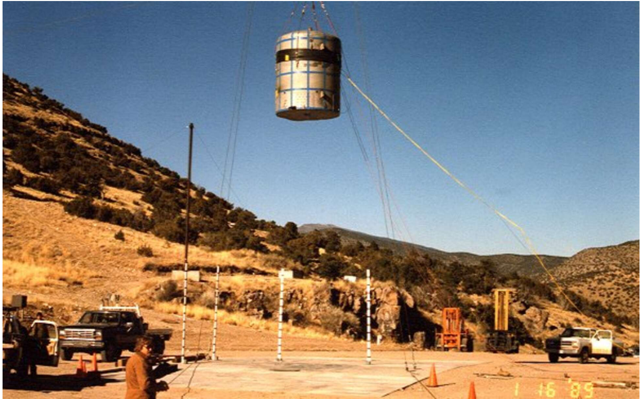
Figure 2.10.3-58 – CTU-2 Free Drop No. 2; Pre-Drop Positioning
