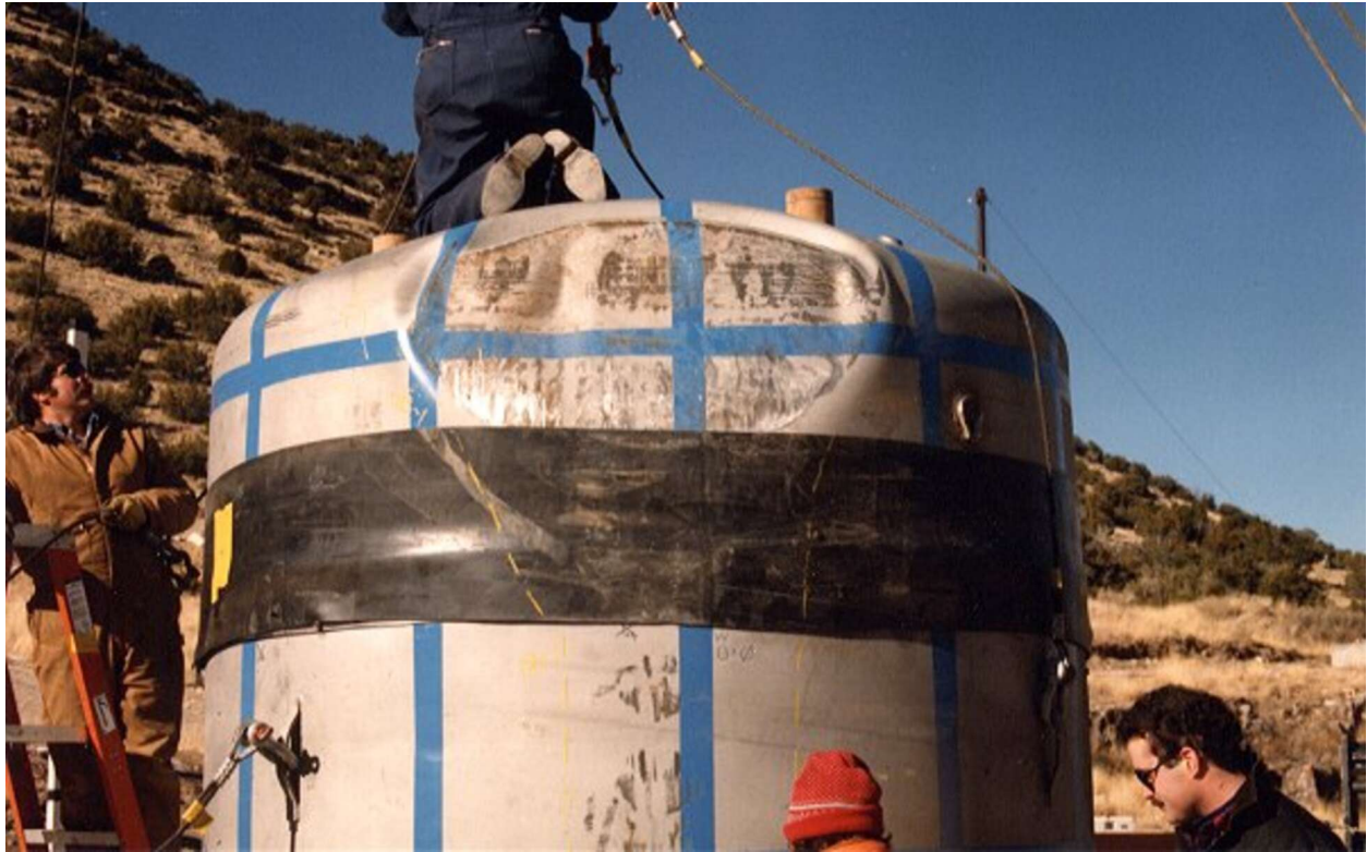
Figure 2.10.3-56 – CTU-2 Free Drop No. 1; Post-Drop Damage
