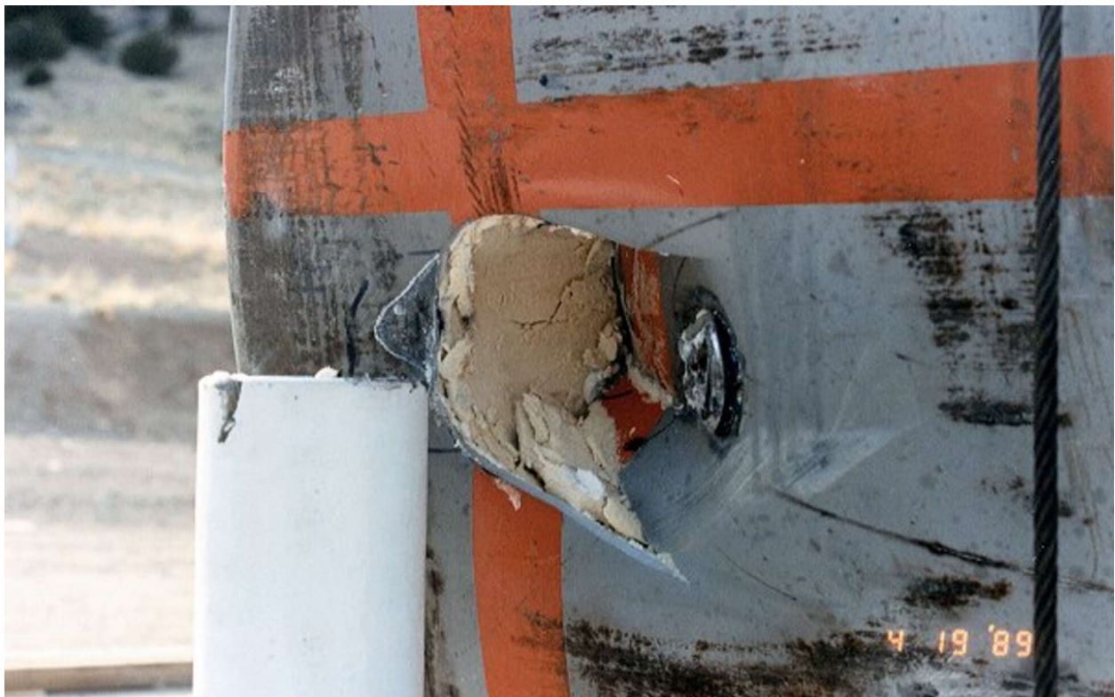
Figure 2.10.3-87 – CTU-3 Puncture Drop 4; Post-Drop Damage
