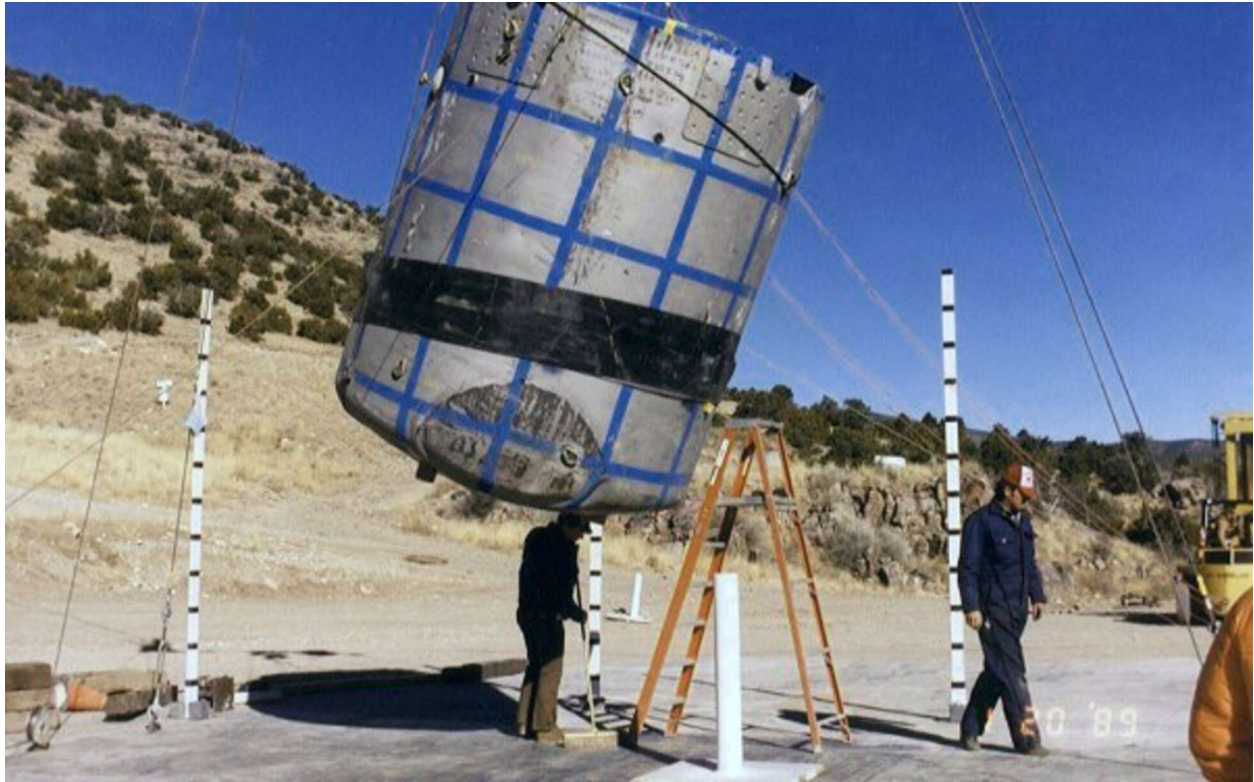
Figure 2.10.3-68 – CTU-2 Puncture Drop No. 6; Pre-Drop Positioning
