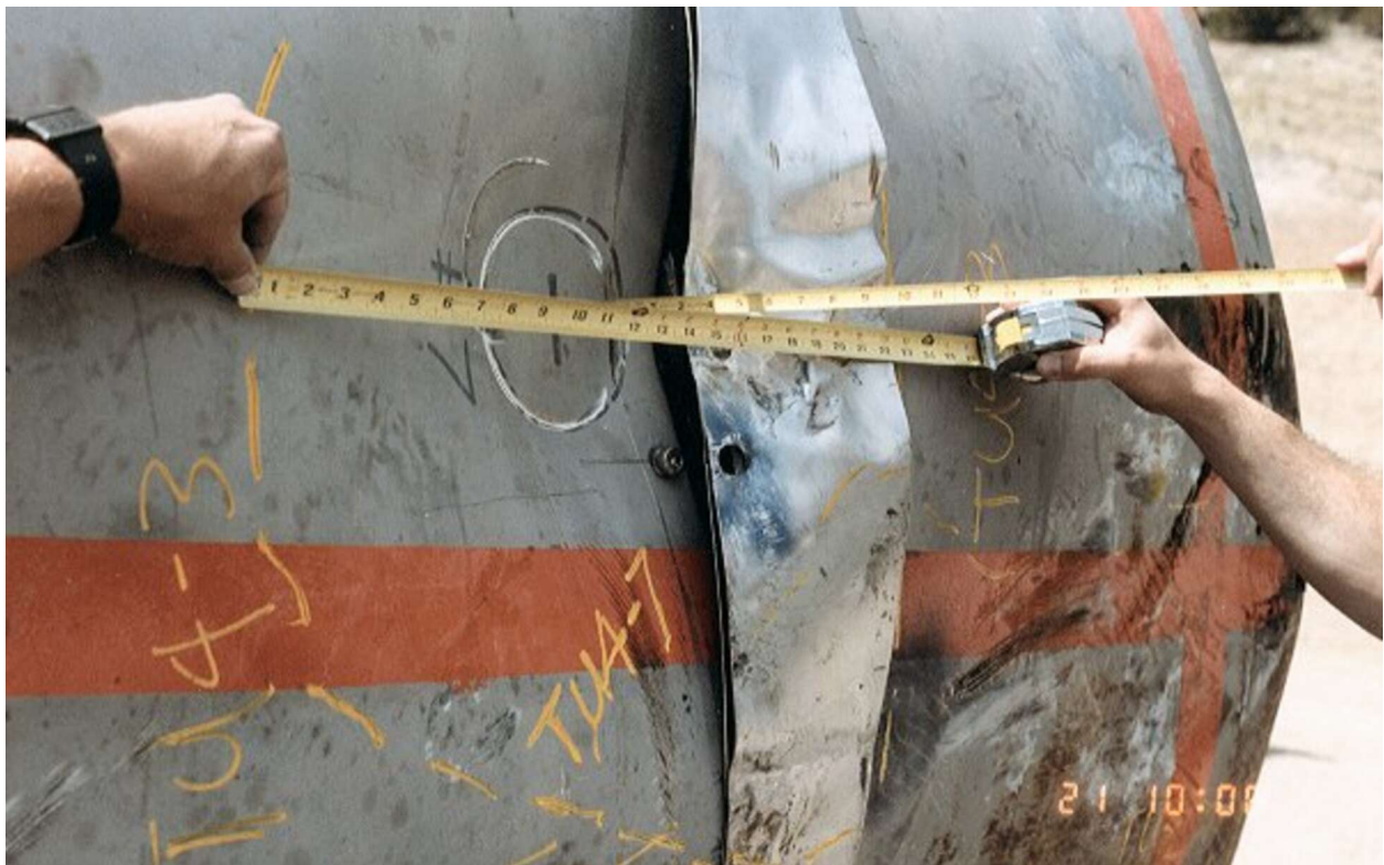
Figure 2.10.3-93 – CTU-3 Puncture Drop 7; Post-Drop Damage
