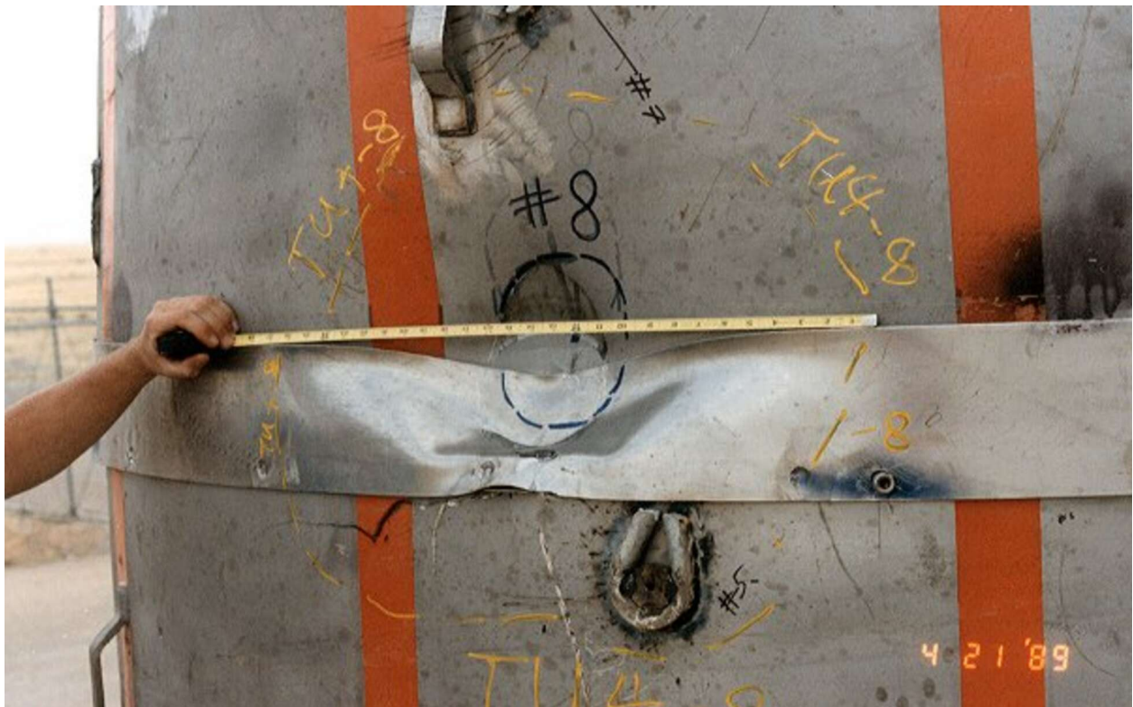
Figure 2.10.3-95 – CTU-3 Puncture Drop 8; Post-Drop Damage
