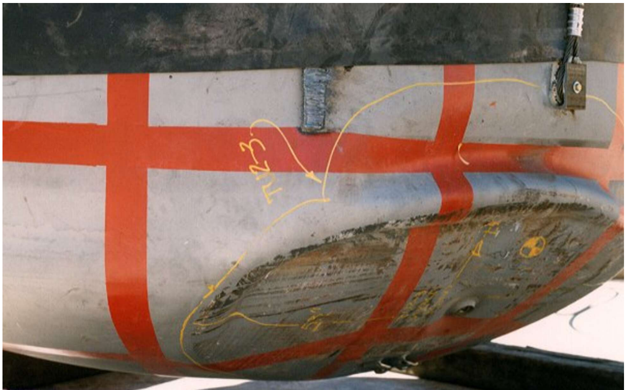
Figure 2.10.3-33 – CTU-1 Free Drop No. 3; Post-Drop Damage
