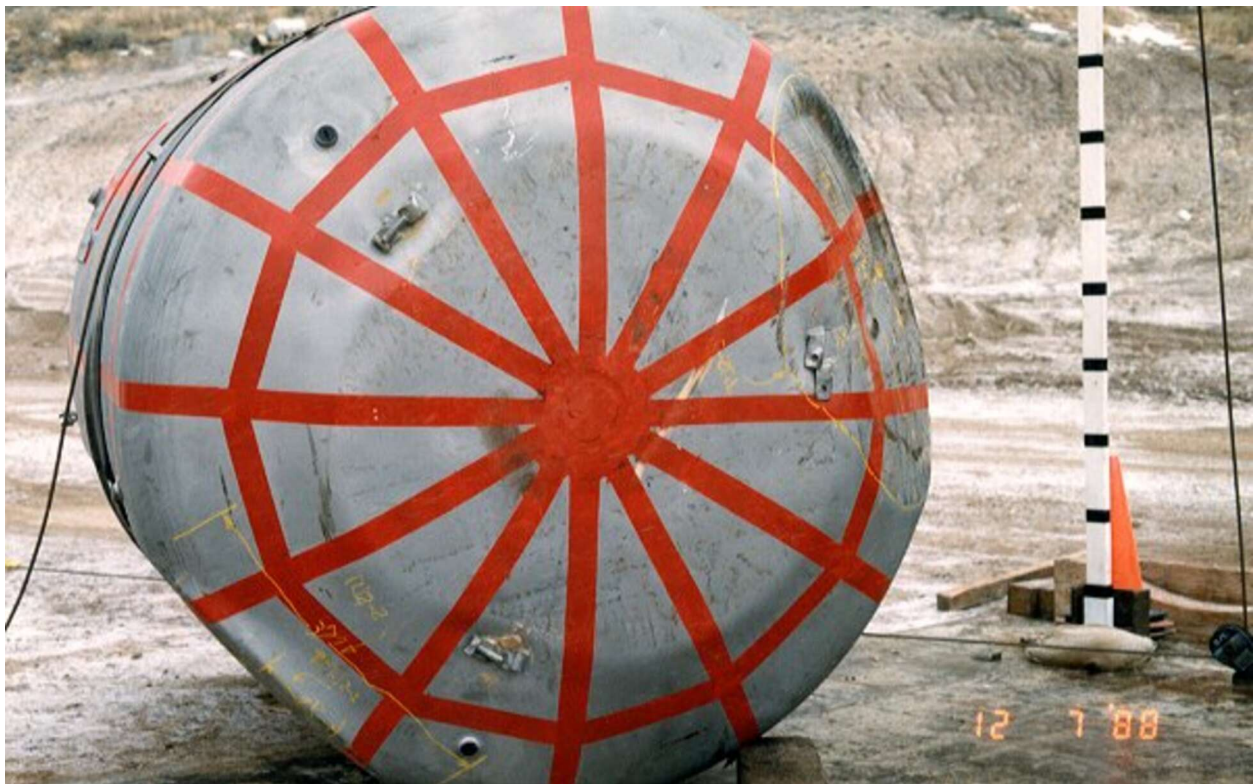
Figure 2.10.3-35 – CTU-1 Free Drop No. 4; Post-Drop Damage
