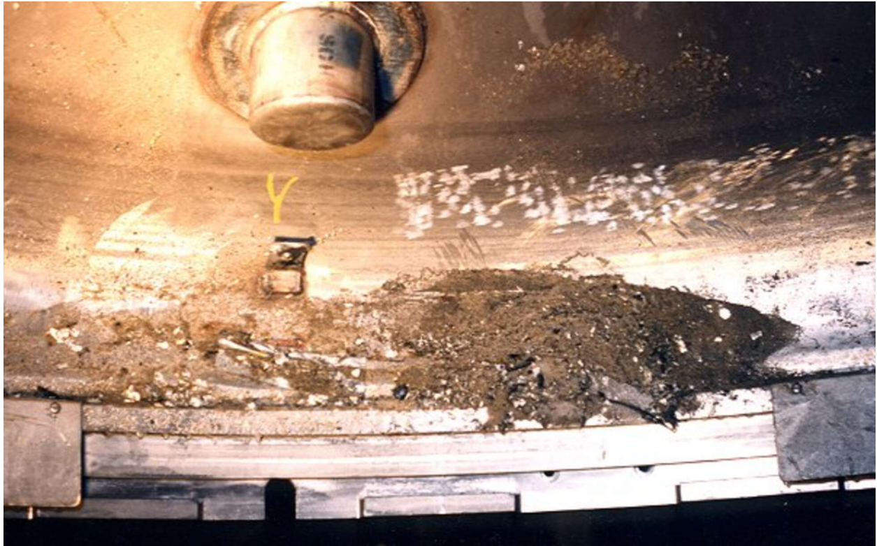
Figure 2.10.3-78 – CTU-2 Disassembly; Loose Debris in ICV Lid
