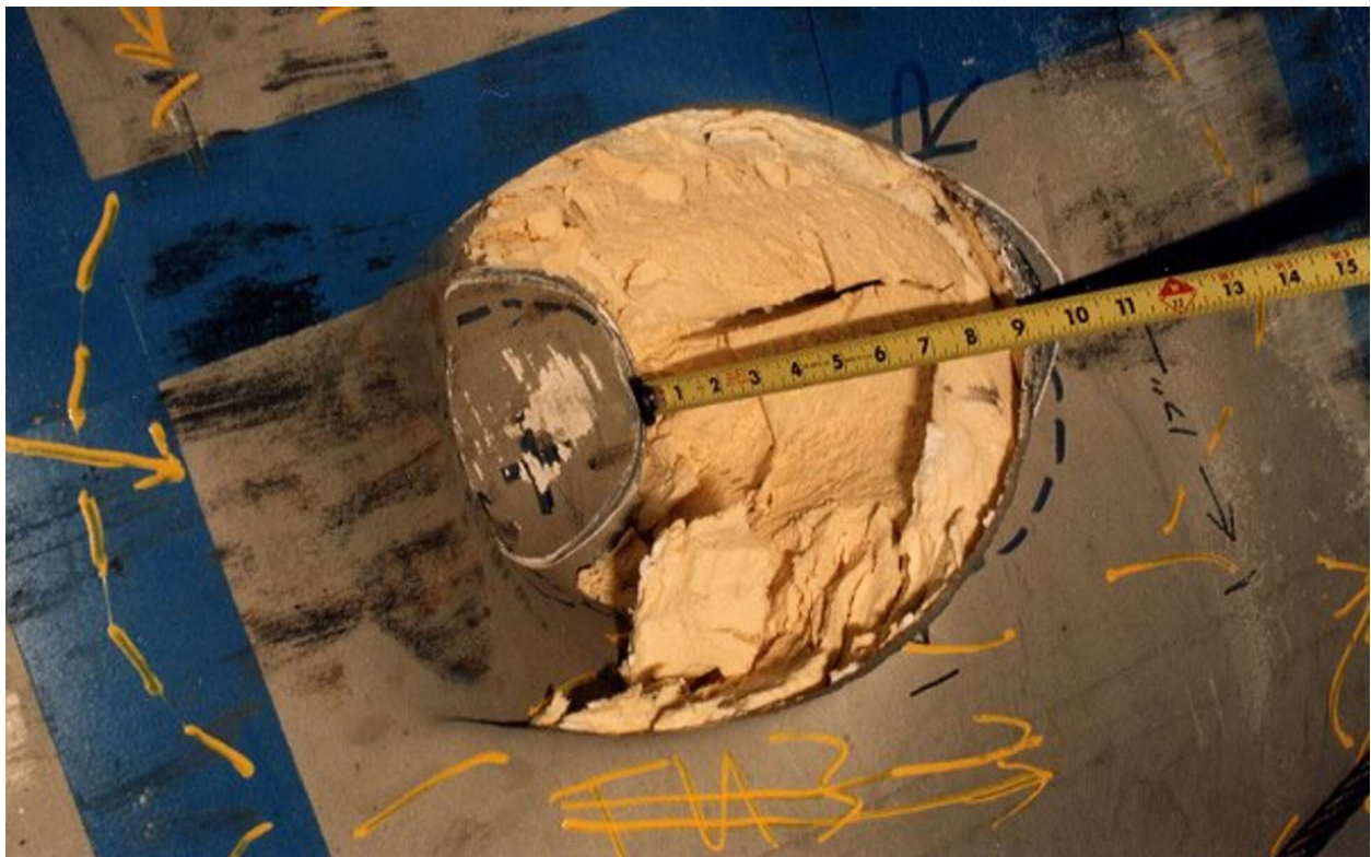
Figure 2.10.3-63 – CTU-2 Puncture Drop R; Post-Drop Damage
