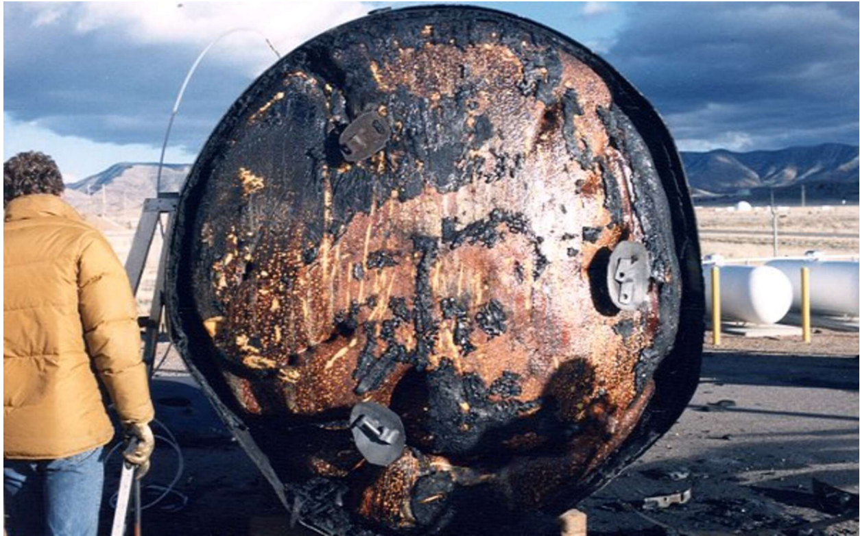
Figure 2.10.3-50 – CTU-1 Disassembly; OCA Lid Unburned Foam
