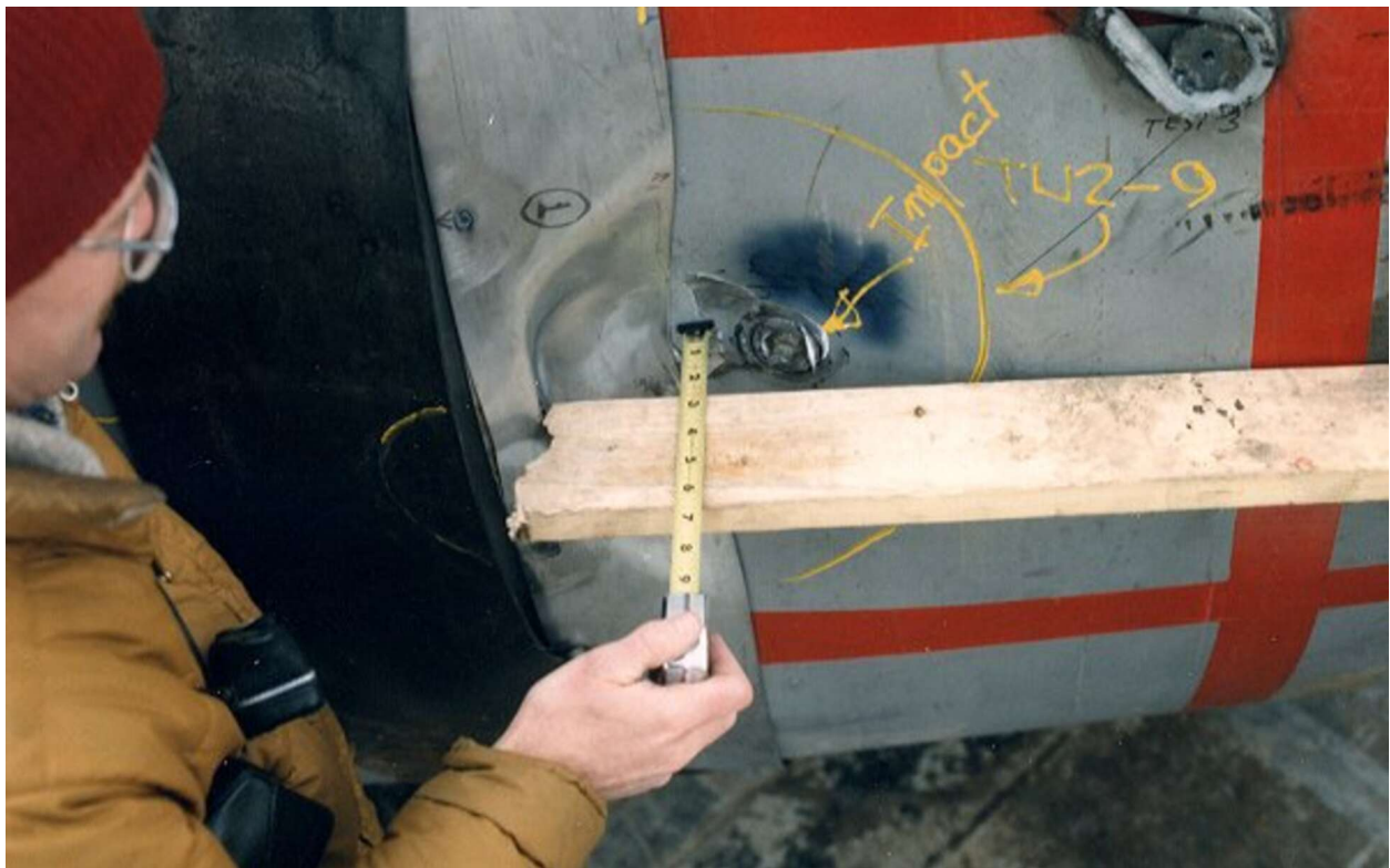
Figure 2.10.3-45 – CTU-1 Puncture Drop No. 9; Post-Drop Damage
