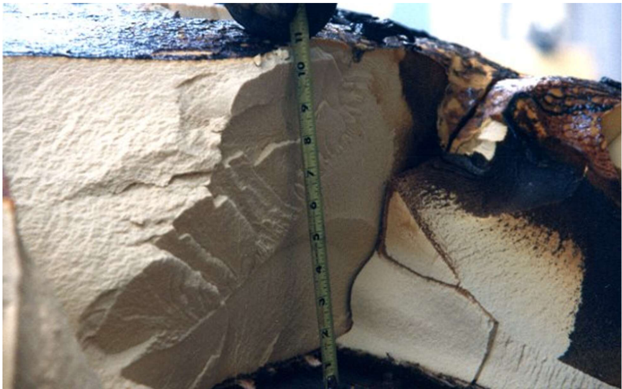
Figure 2.10.3-51 – CTU-1 Disassembly; OCA Lid Unburned Foam Thickness
