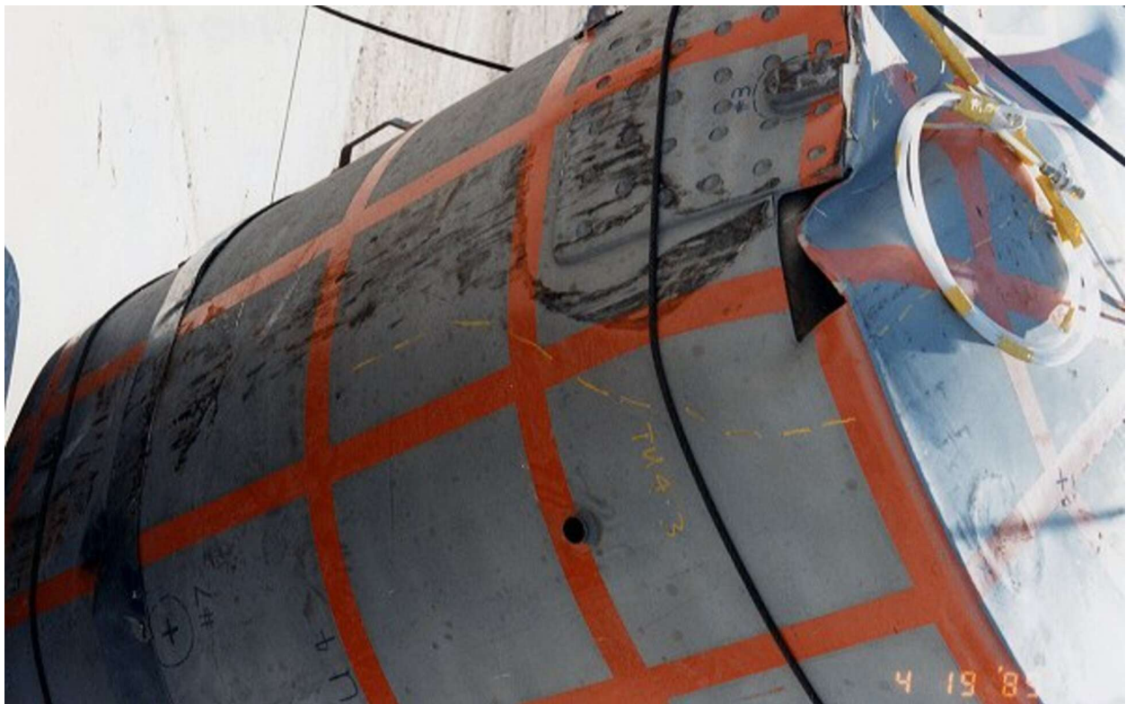
Figure 2.10.3-85 – CTU-3 Free Drop No. 3; Post-Drop Damage
