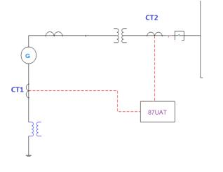
Maintenance of the Unit Auxiliary Transformer breakers is particularly important because their failure could lead to an extended duration generator-fed fault at the first switchgear bus. Operating experience has shown that this breaker is more likely to fail during automatic bus transfers.
