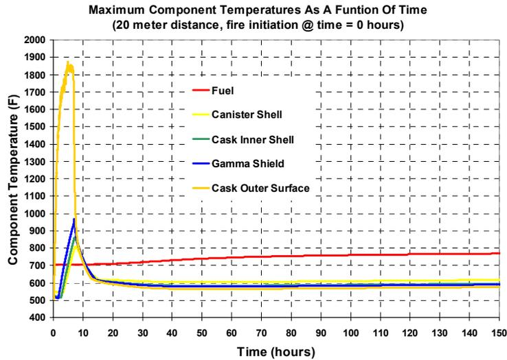
**Figure 5.** Component Temperature Plot
