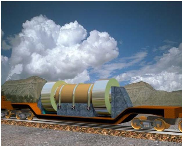
**Figure 3.** Spent Fuel Cask on Railcar (Image Courtesy of HOLTEC International)
