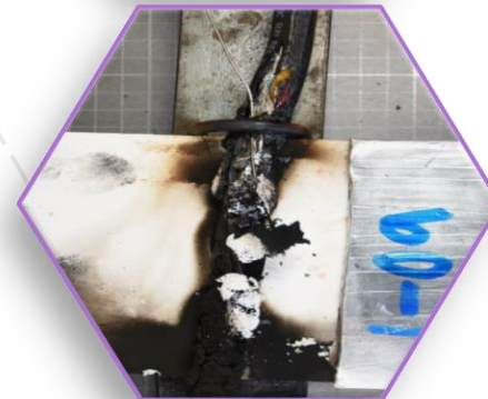
Test 1-09 (206 MJ/m²): Cable insulation and bare wire exposed
