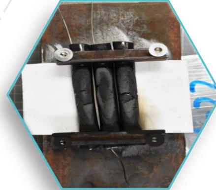
Test 1-22 (7 MJ/m²): Surface damage to jacket only
