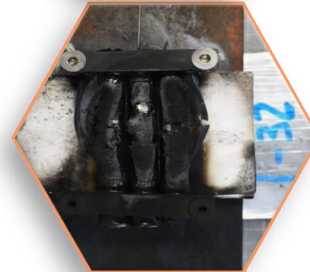
Test 1-32 (24 MJ/m²): Sub-jacket shielding visible
