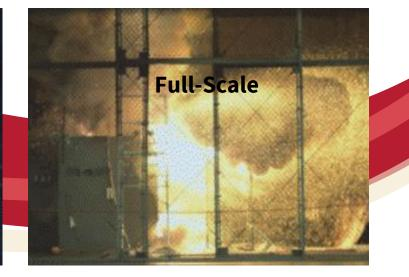
Enclosure breach, event progression, pressure rise, thermal/visual imaging. Served as benchmark cases for CFD model.
