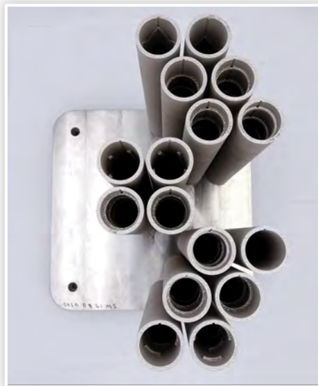
Additive manufacturing of ribbed piping for improved heat transfer
