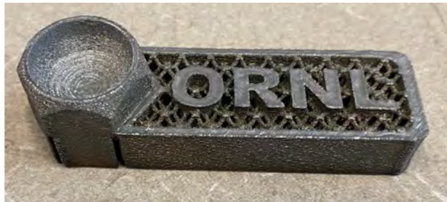
Pure tungsten (W) plasma-facing component coupled with mesh structure
