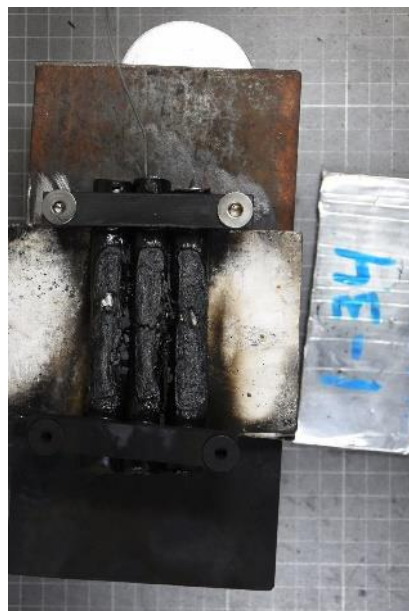
Figure 7 Solar Furnace Test 1-34 (3 cable bundle, ~ 25 MJ/m 2 )
