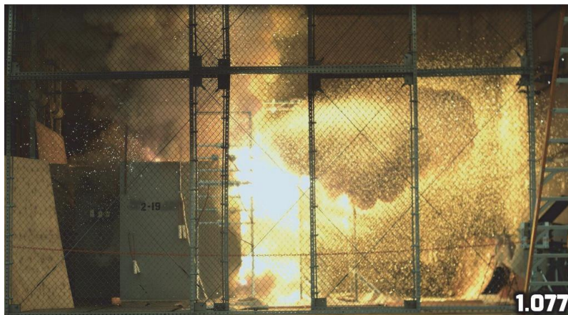
Figure 5 Medium voltage switchgear testing, Test 2-19 (6.9 kV, 25.8 kA rms)
