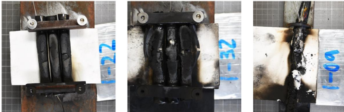
Figure 3 Post-test thermoplastic cable following incident energy exposure to 7 MJ/m 2 (test 1-22), 24 MJ/m 2 (1-32), and 206 MJ/m 2 (test 1-09)
