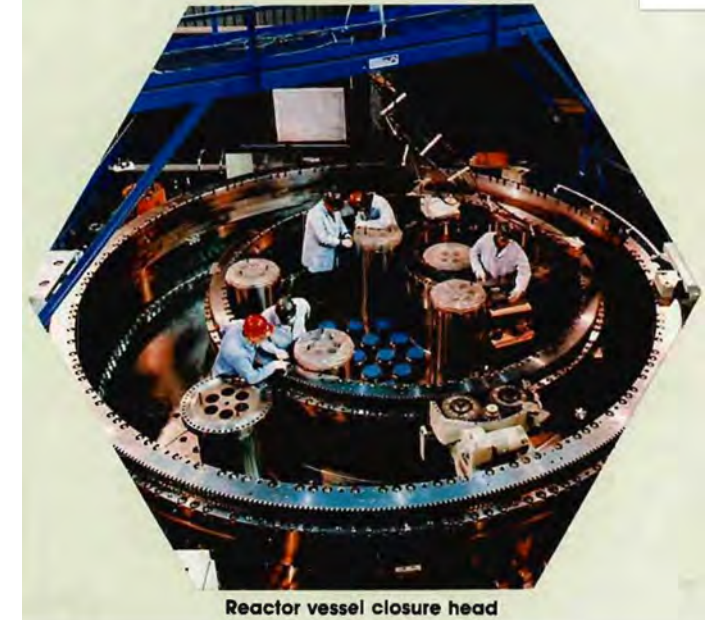
Reactor vessel closure head
