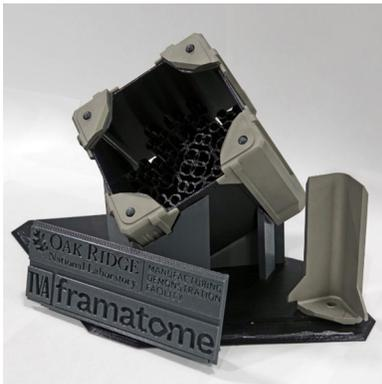
Figure 14. Assembly channel fasteners developed for use in the Browns Ferry-2 reactor [63].
