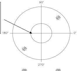
TSC mid-plane – approximately 92 inches from bottom. Measure dose rates at four target points (approximately 0, 90, 180 & 270 degrees) on the mid-plane.
