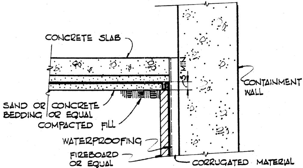
WATERPROOFING AT FLOOR SLAB AGAINST CONTAINMENT WALL
