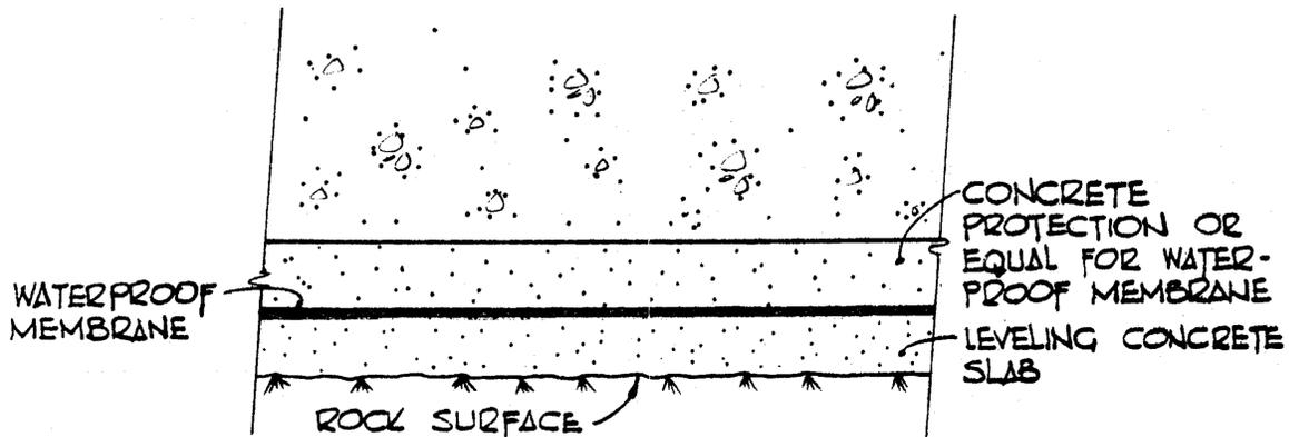
WATERPROOFING AT BOTTOM SIDE OF FOUNDATION MAT ON ROCK
