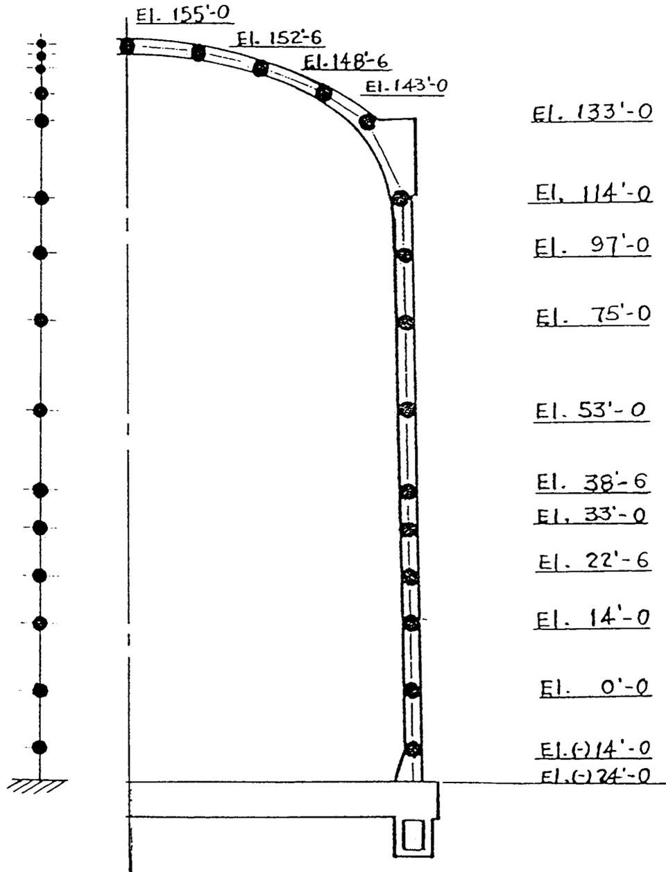
**FIGURE 5.8-15 MODE SHAPES FOR THE CONTAINMENT BUILDING**
