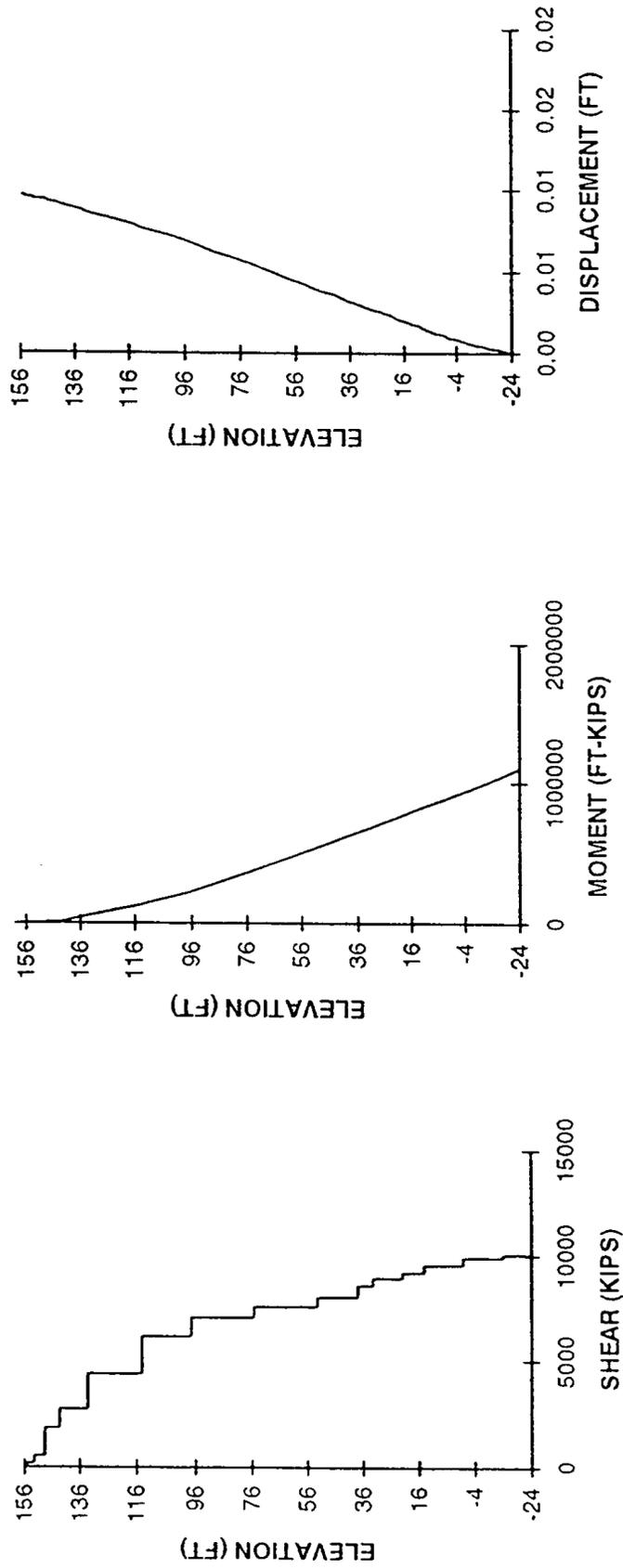
**FIGURE 5.8-17 CONTAINMENT BUILDING DESIGN EARTHQUAKE 17% GROUND ACCELERATION**
