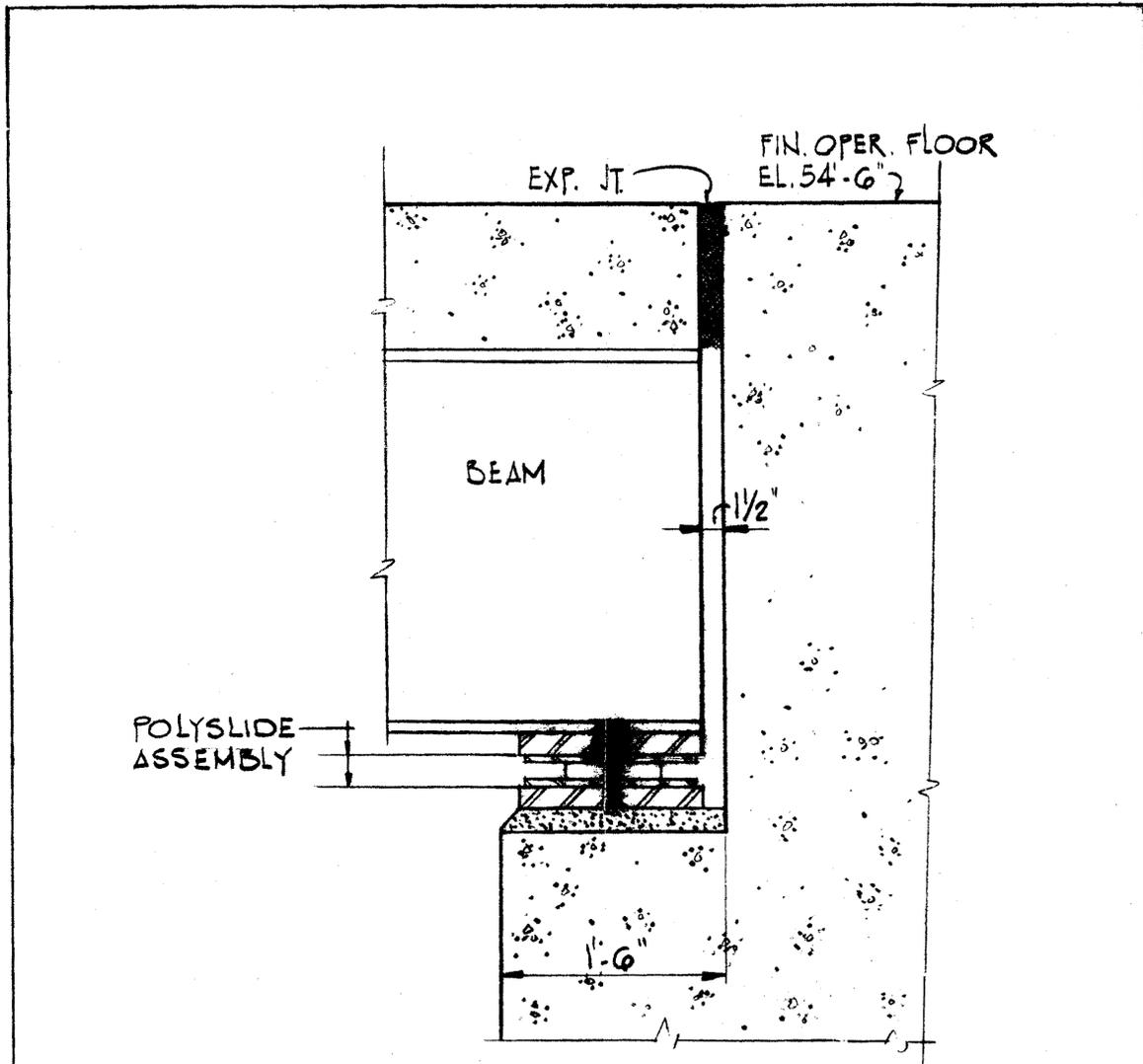
JOINT DETAIL AT TURBINE PEDESTAL
