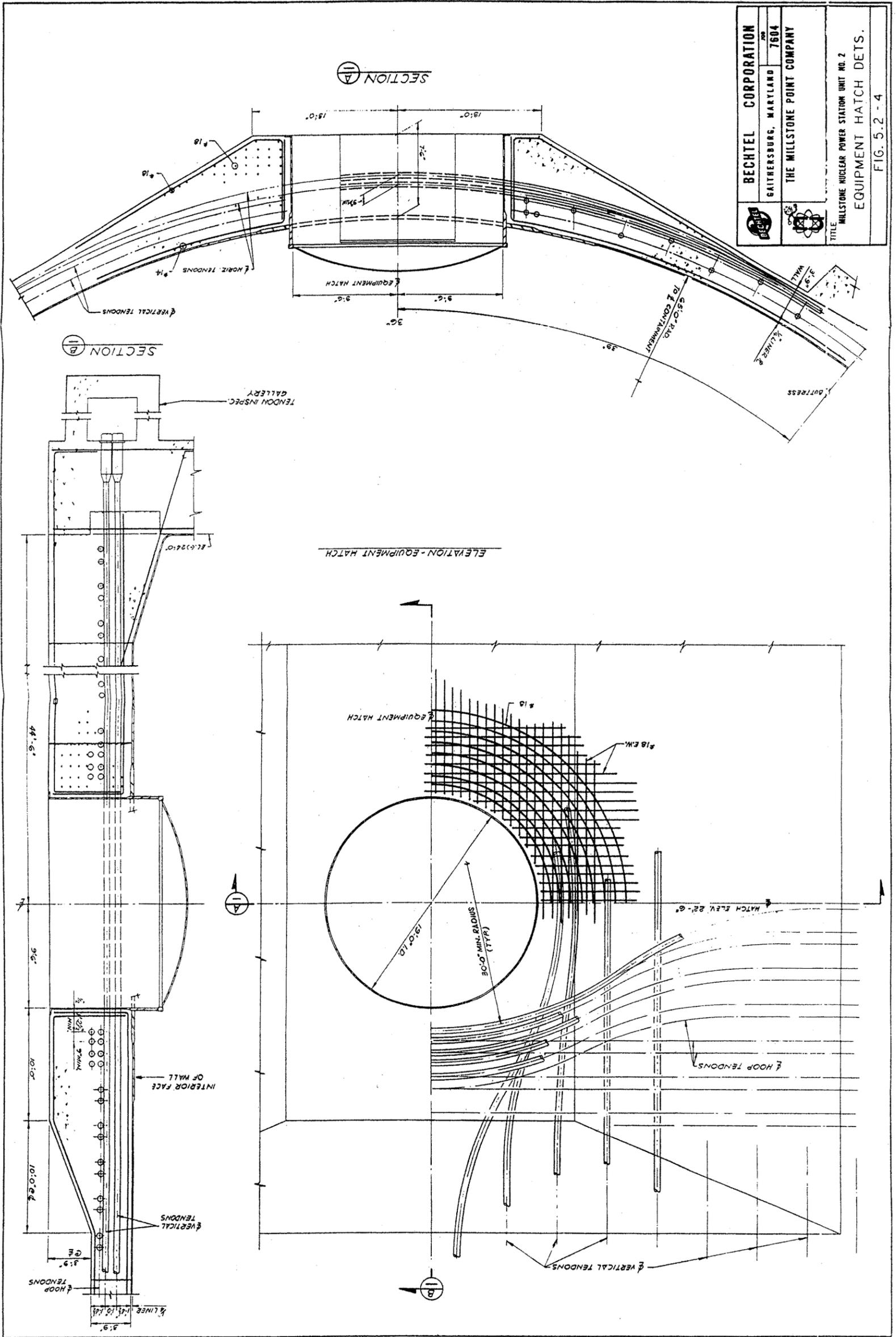
FIGURE 5.2-4 EQUIPMENT HATCH DETAILS
