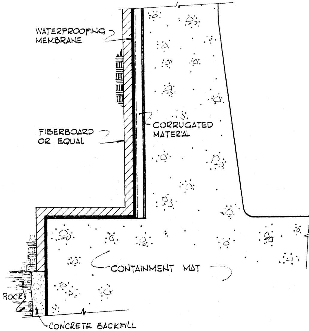
**WATERPROOFING AT CONTAINMENT MAT AND WALL INTERSECTION**
