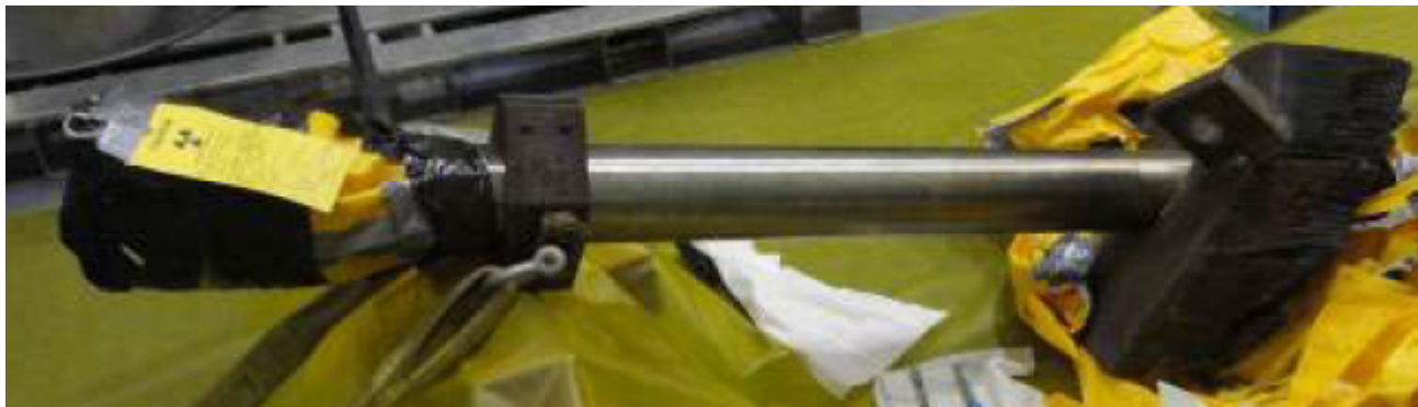
Figure: Control rod drive mechanism (CRDM) Nozzle 63 from the North Anna Unit 2 reactor ( NUREG/CR-7142 )
