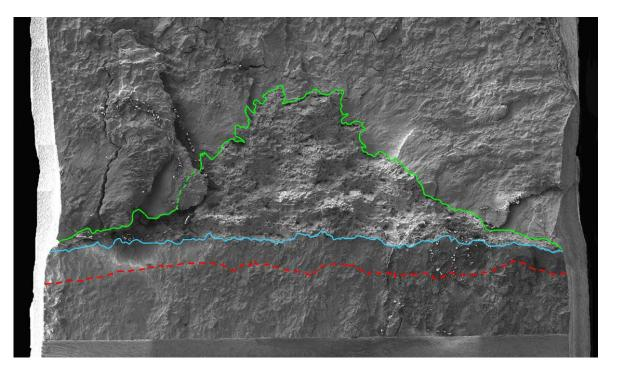
HAZ Fracture surface and tracing of crack fronts, taken from MRP-451 (Zorita Weld HAZ)
