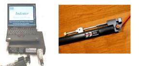
Oven-aged cables used for training aids for demonstrating how to use the indenter to monitor cable hardening.
