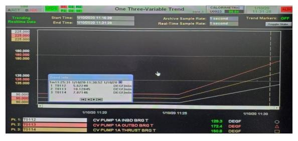
(1) If FP is NOT aligned to the 1A CV pump oil coolers, 1A CV pump temperatures will initially reach a trip limit at...
