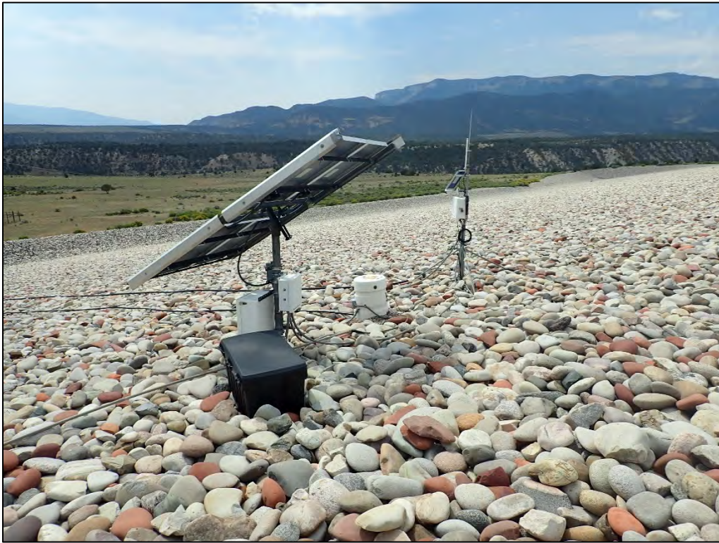
PL-5. Standpipe SP-02 and Instrumentation
