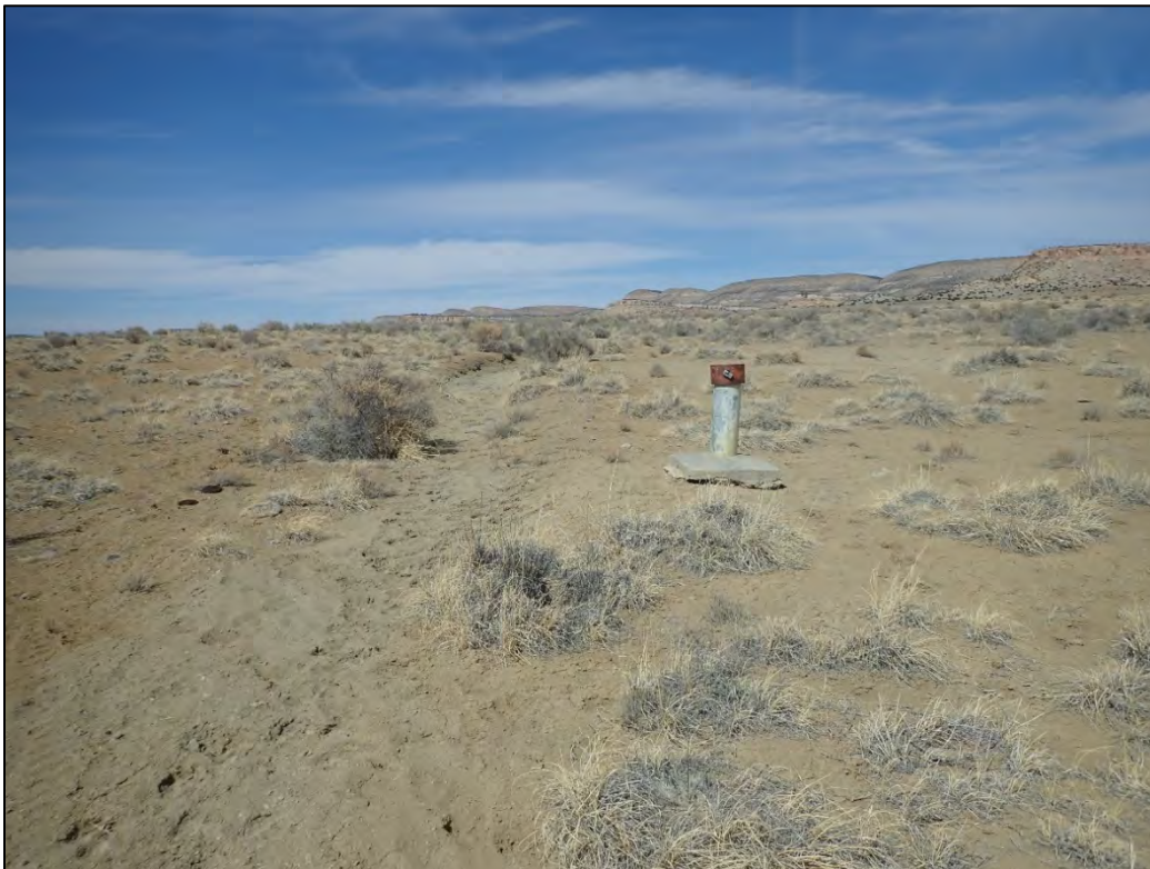
PL-6. Erosional Rills Around Monitoring Well 0678
